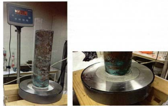
Figure 2-1. Left: copper heater and steel bottom plate. The plastic filter (white) is visible at the bottom of the groove. The outer diameter of this groove is 18.2 cm, and the inner diameter is 10.8 cm. Right: bentonite ring emplaced.
