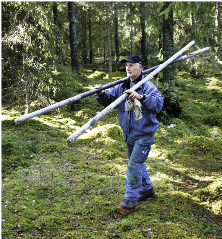
Figure 2. More than two-hundred, 3-m long, unbroken core sticks were acquired at depth during core drillings, which support the hydraulic observation of few flowing fractures in the deeper bedrock.
