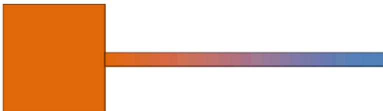
Figure A3. The walls of the container are impervious to water and to colloids. The clay in the container is fully water saturated and the fracture is filled with water.
