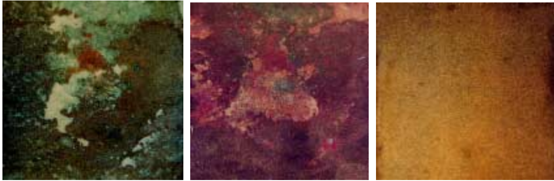
Figure 8-2 Copper coupon A after removal from bentonite (left), after the final washing in water (centre), and coupon J after the last treatment with diluted H_2SO_4 , (right). Coupons A and J had a similar appearance after the last treatment.
