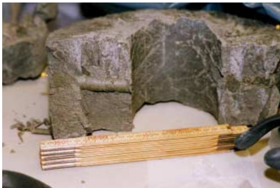
Figure 7-1 Block 29 in the S1 parcel has been ruptured and a set of three plugs that were inoculated with bacteria become visible. The plugs were removed and analysed after 15 months' exposure. (Photograph: M. Motamedi)
