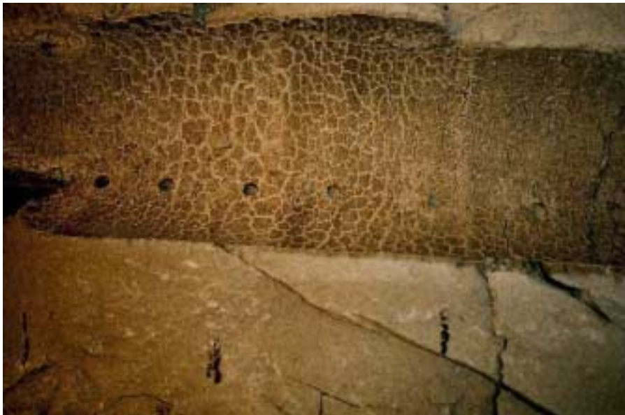
Figure 4-14 Inner mantle surface of the bentonite, which was in contact with the copper tube in parcel S1. The small holes in the centre are due to sampling for tracer analyses. Photograph by Kjell Svärdröm, KTH, Stockholm.
