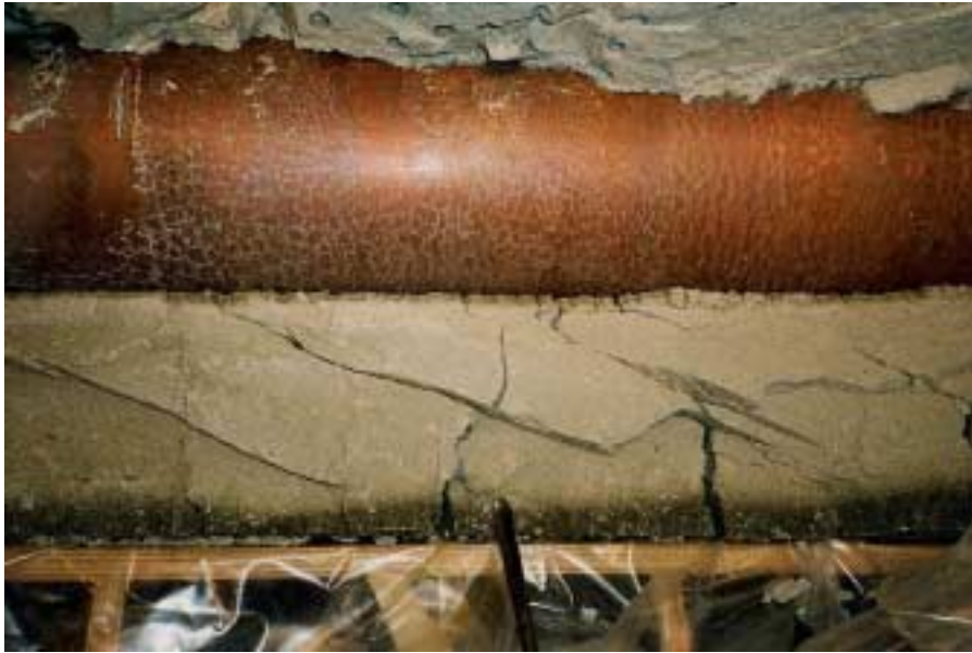
Figure 4-13 White precipitation on the copper tube in the S1 parcel. Note also the darker mm-thick precipitation affected layer just below the copper tube. Photograph by Kjell Svärdröm, KTH, Stockholm.
