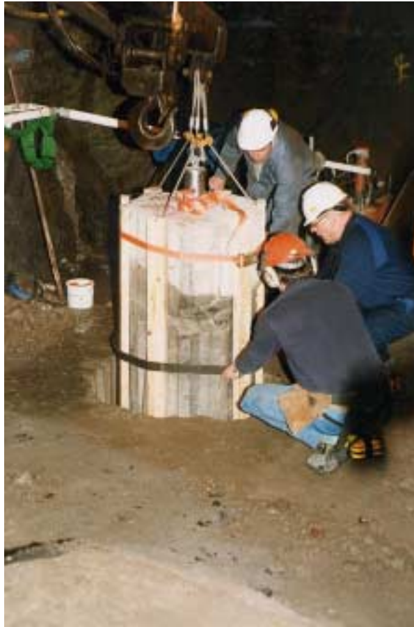
Figure 4-11 Uplift of the S1 parcel after termination.
