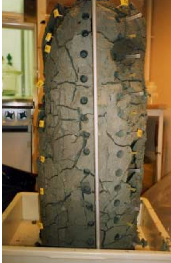
Figure 6-2 Lower part of test parcel A-1. The holes are due to sampling. Photograph by Kjell Svärdröm, KTH, Stockholm.
