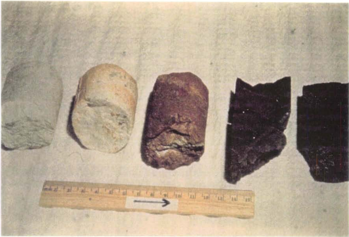
Figure 2.5 Profile from the massive clay showing the colour change from the clay/ore contact (grey/black) grading through to the Fe-oxyhydroxide/hematite clay (red) to eventually the bleached (white) clay [SKB's archive material].
