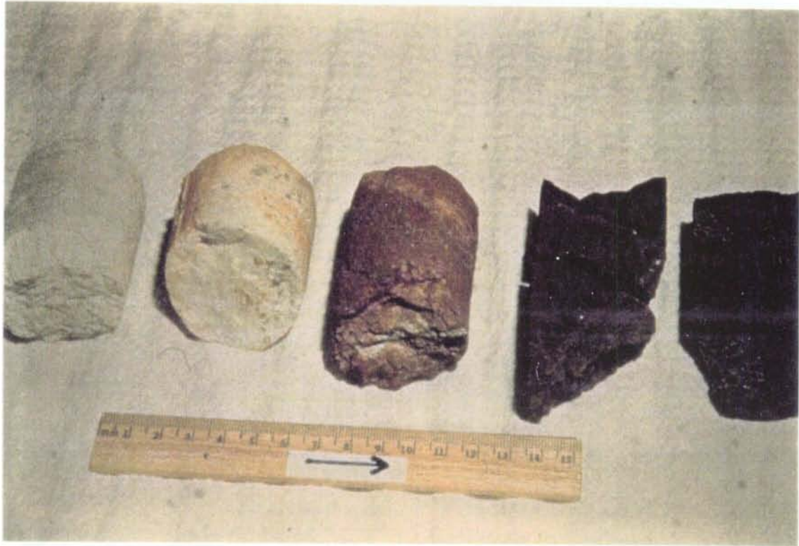
Figure 4.2 Drillcore through the clay halo surrounding the uranium ore at Cigar Lake. The clay close to the ore has been coloured by haematite (from [SKB, 1992b]).
