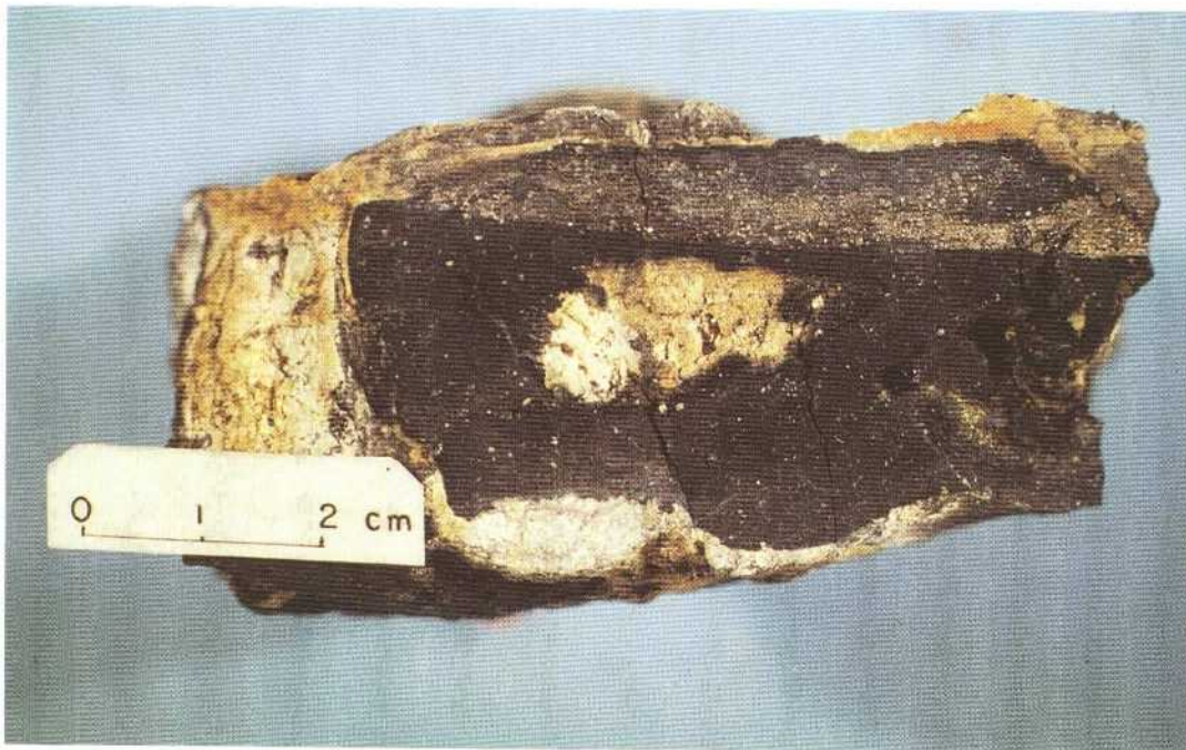
PLATE 3:9-8. Sawn surface of the nodule illustrated in Plate 3:9-7. The nodule consists of a white coloured core of hydrothermally altered and argillised rock (phonolite), surrounded by a black nodule-forming pitchblende zone and a fine external yellowish white clay shell. Note the "horizontal" zone which is extremely rich in secondary coarse-grained pyrites in the top portion of the pitchblende zone (yellow reflectivity). This probably represents a former water table-related phenomenon.
