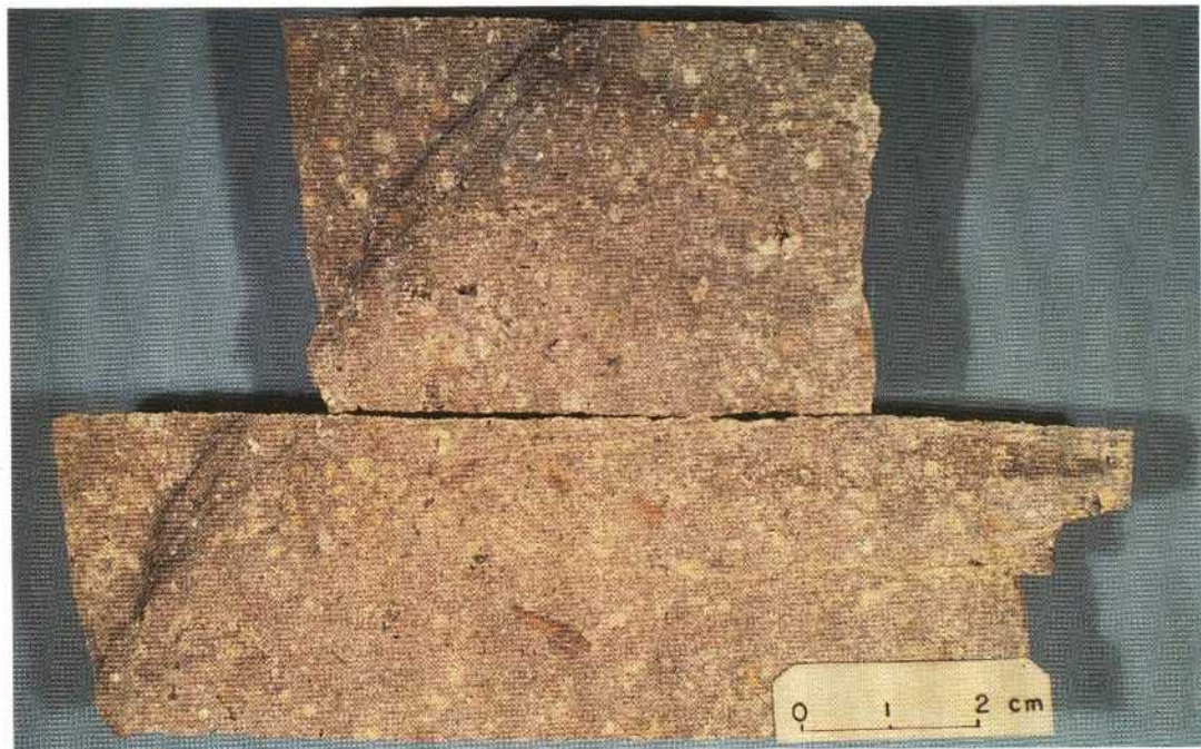
PLATE 3:9-2. Reduced medium-grained porphyritic phonolite with massive structures. The dark seams in the left hand corners of the drillcores are hydrothermally altered fractures mineralised with microcrystalline pyrite.
