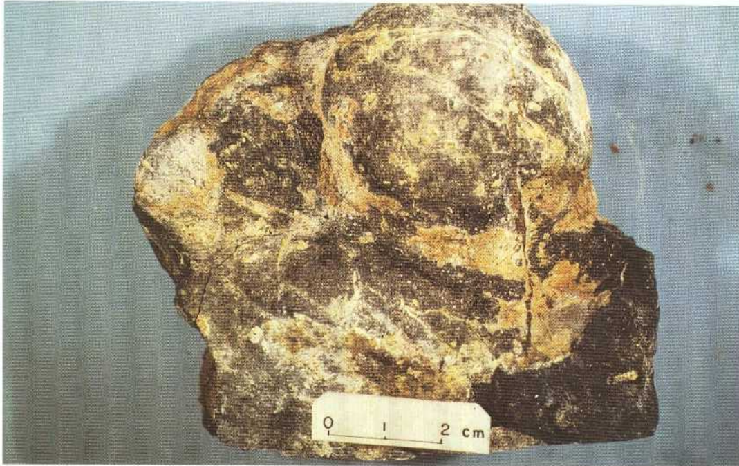
PLATE 3:9-7. Massive pitchblende nodule. Note external concretionary "Löss-Kindl" shape. Specimen no. S/N-24.
