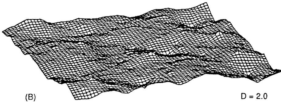
Examples of fractal surfaces used in the simulations. Both surfaces have the same rms height  $\sigma$ . Both were generated with the same set of random numbers but have different fractal dimensions. The fractal dimensions shown ( $D = 2.0, 2.5$ ) represent the limiting values observed by *Brown and Scholz (1985b)*.
