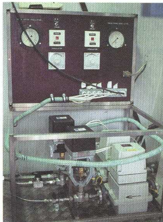
Figure 7.12 Schematic illustration of the Pipe String Equipment with photos from the operator's room and the flow meter and flow regulator unit used for pumping tests.
