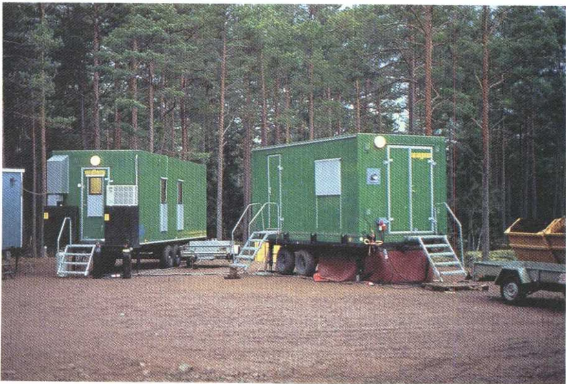
Figure 9.4 The two trailers of the mobile field laboratory, similar as the trailers of the Umbilical Hose System.
