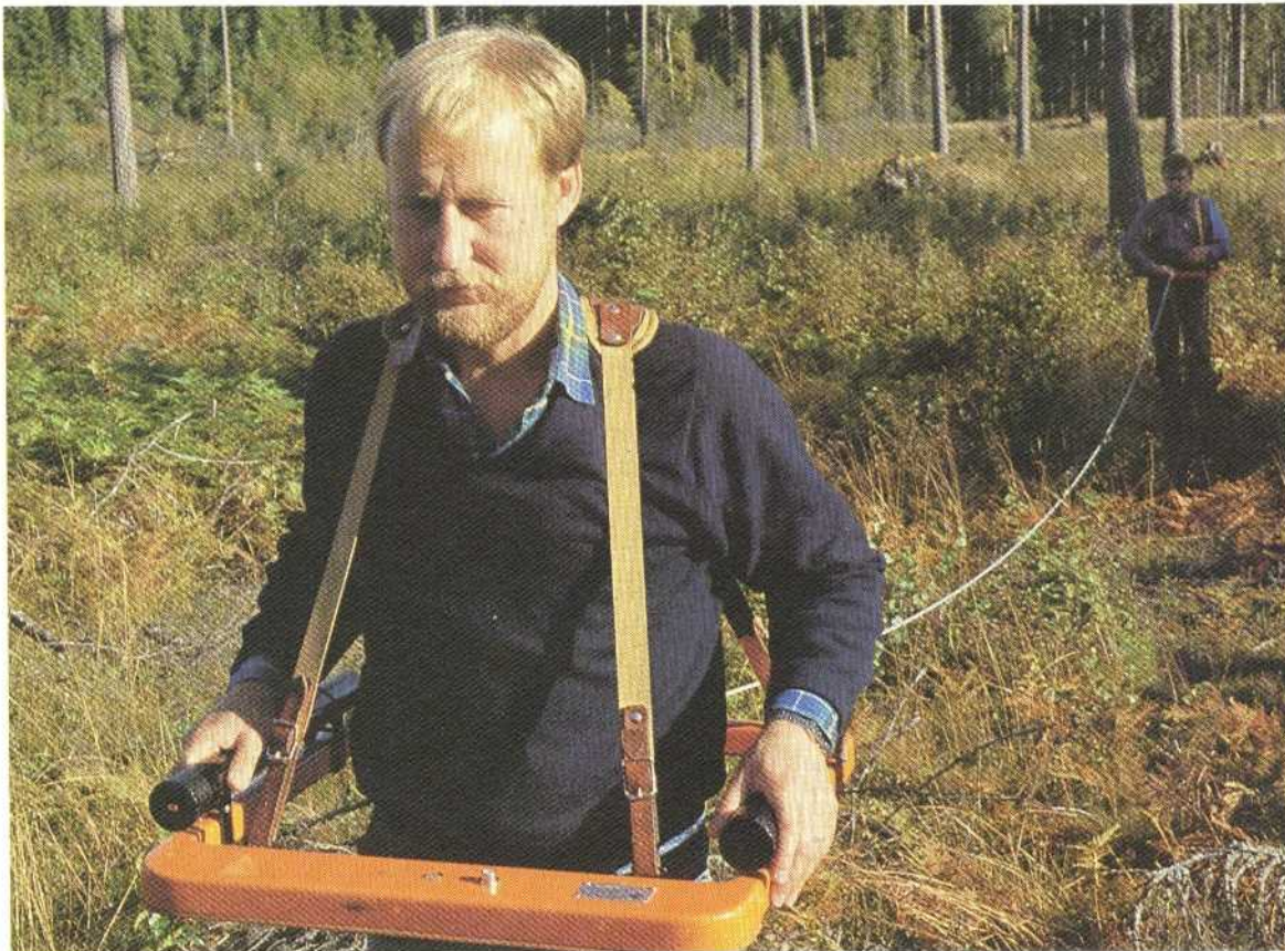
Figure 3.6 Measurements with the ABEM EMAC (Slingram), a horizontal Loop EM system.
