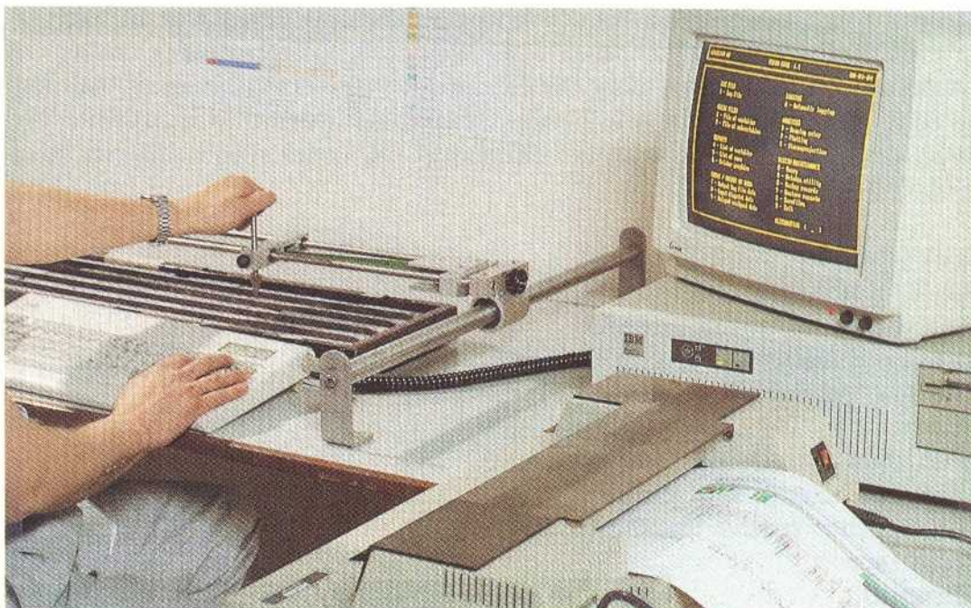
Figure 5.2 Core logging with the PetroCore system.
