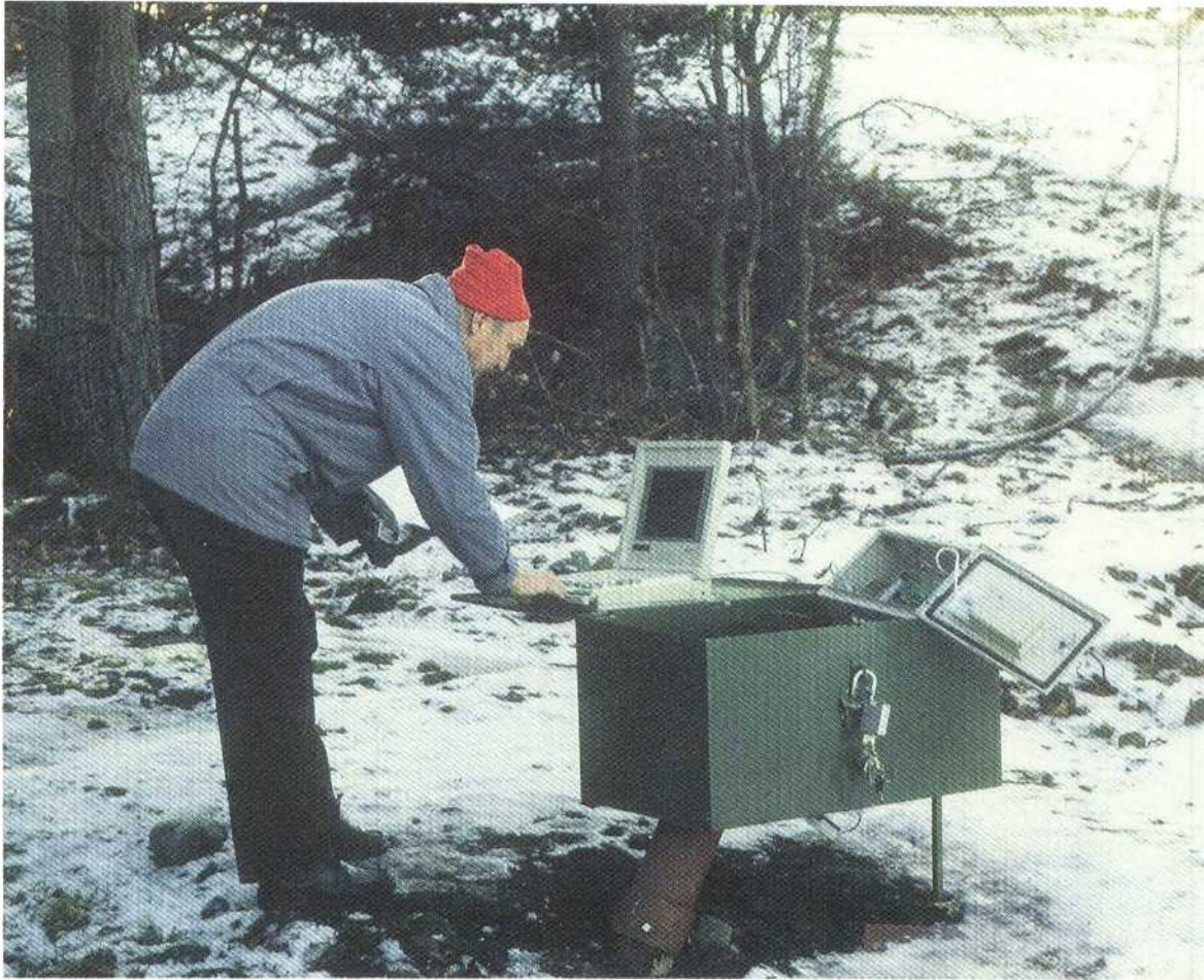
Figure 8.13 Data transfer from a Borre datalogger to the site office, via a laptop computer.
