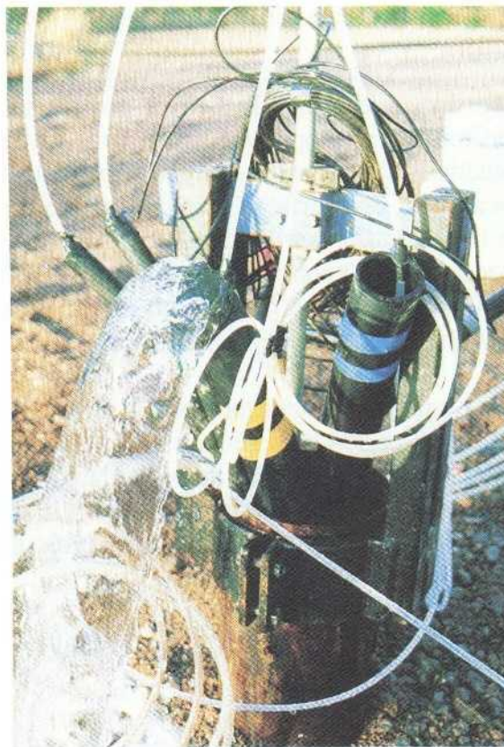
Figure 8.6 Airlift pumping of stand-pipes, for water sampling and determination of the density of the water column.
