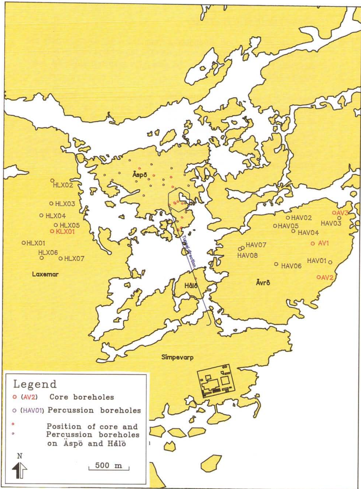
Figure 3-1. Overview of the borehole locations in the pre-investigation area.
