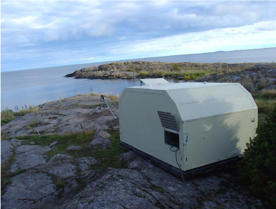
Figure 5-1. Example of a borehole location, in this case HAV11. The location close to the shore-line gives most certainly a conductive environment due to salt-water intrusion.
