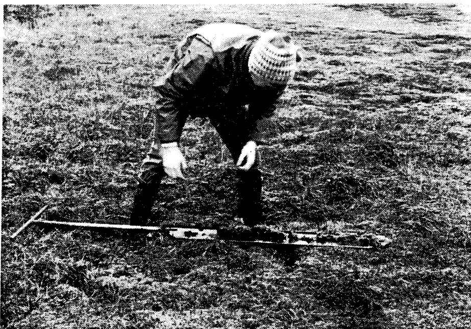
Figure C.2.3 Peat profile sampling, with a standard Russian peat sampler.
