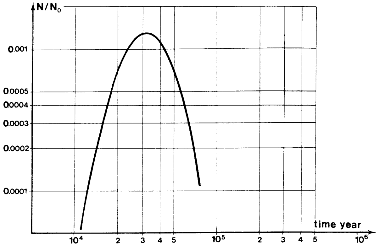
Figure 5. Breakthrough curve for \text{Am}^{243} D_a = 1.4 \cdot 10^{-14} \text{ m}^2/\text{s} , z_o = 0.375 \text{ m}
