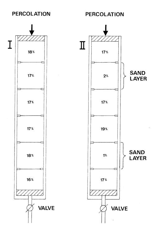
Fig. 10. Clay content distribution in Test 2. Mean values given for each section.
