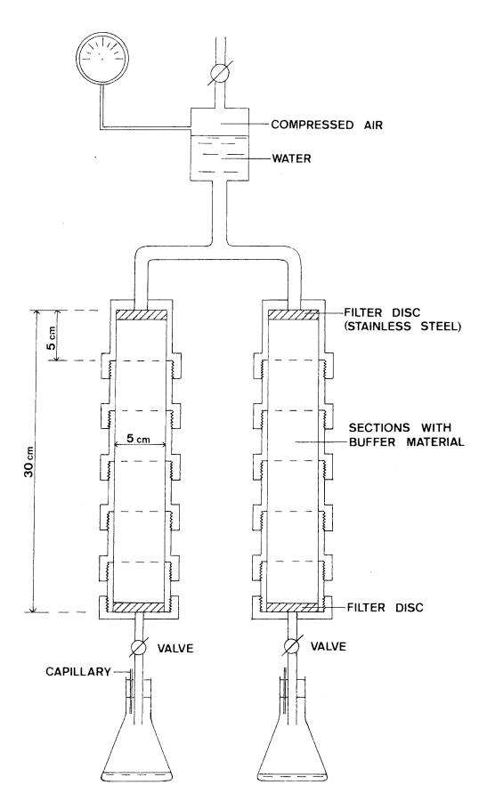
Fig. 6. Schematic view of test device.
