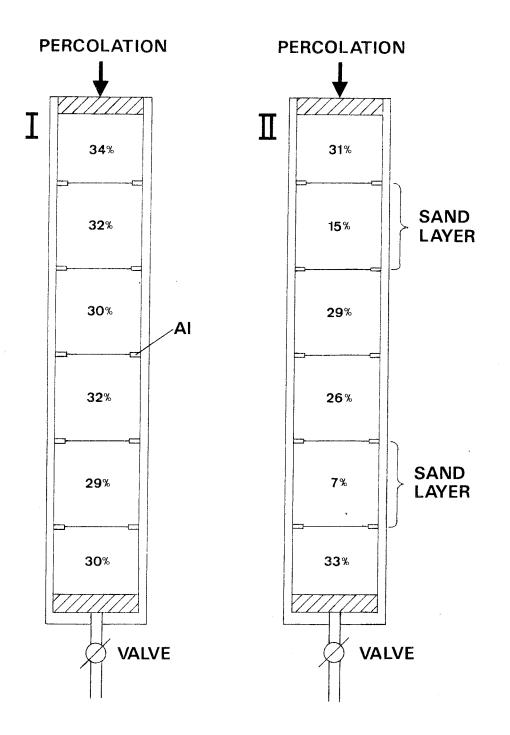
Fig. 9. Water content distribution in Test 2. Mean values given for each section. Al stands for aluminium rings which were inserted between the sections in order to prevent piping by extending the flow path along the walls.
