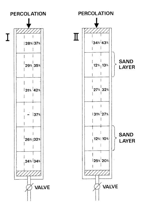
Fig. 7. Water content distribution in Test 1. Mean values for peripheral and central elements given for each section. I stands for test with 20% Na bentonite and 80% quartz powder. II stands for test with two quartz sections.
