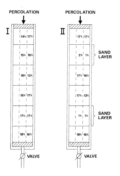
Fig. 8. Clay content distribution in Test 1. Mean values for peripheral and central elements given for each section. The sand contains a minor amount of clay also before the test. Its distribution after the test is shown in Fig. 8. No significant tendency of washing out or enrichment of clay-sized particles can be observed even in the column with sand layers where piping occurred.
