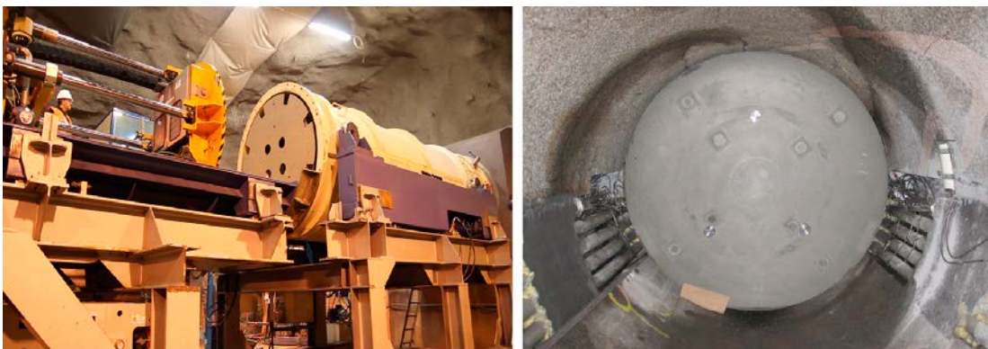
Figure 4-16. To the left the deposition machine is about to pick up a component in the transport tube and to the right a picture of a distance block in place in the drift with all its sensors connected.
