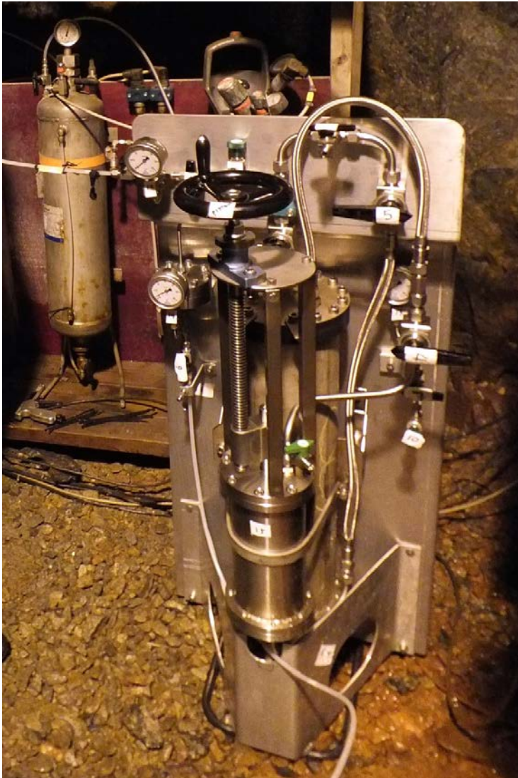
Figure 7-18. Sampling vessel for preservation of RNA from borehole water maintained under in situ conditions.
