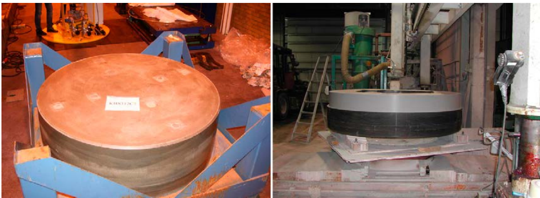
Figure 4-11. To the left a recently compacted distance block and to the right machining to the required dimensions.
