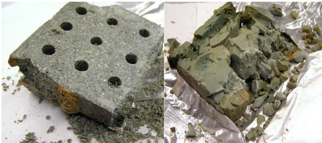
Figure 8-1. Examples for perfect blocks which were sampled in 1 mm, 2 cm, 5 cm, and 8 cm distance from the contact to the tube (left) and disintegrating blocks which were difficult to sample (right, block 26).
