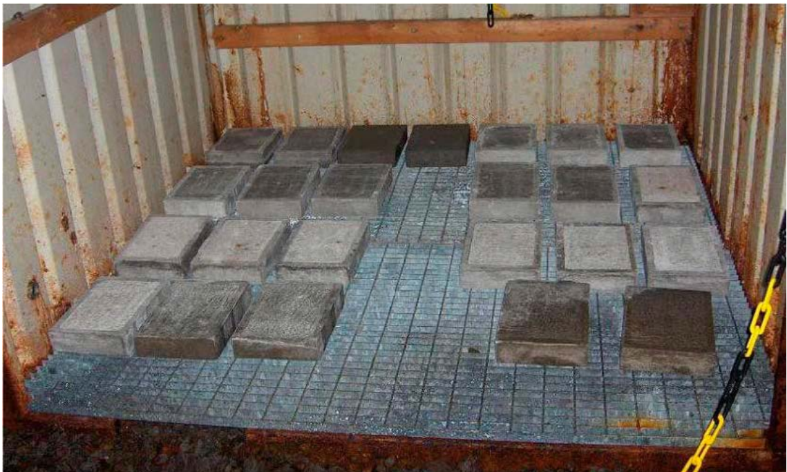
Figure 4-32. Container in Äspö HRL with corrosion tests samples.
