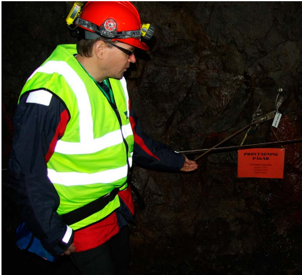
Figure 7-3. Sampling of fracture groundwater for characterisation of dissolved concentrations of lanthanoids. Photo: Tobias Berger.
