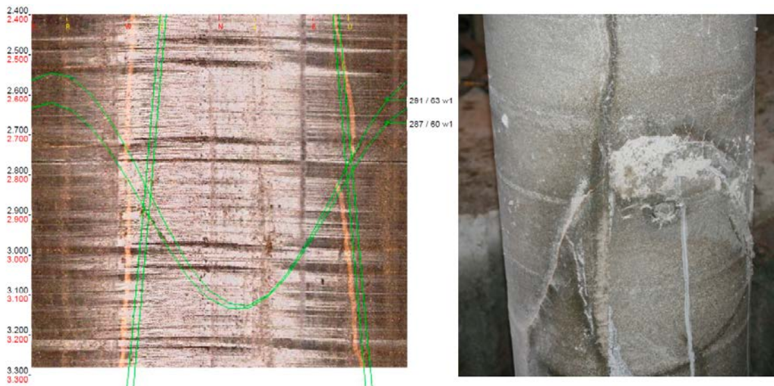
Figure 3-2. BIPS-image from Hole 17 which shows the fracture at 2.6–3.1 m and the pegmatite vein (left), and photo from the dismantling of the parcel in Hole 17 (right) which shows markings from the same fracture.
