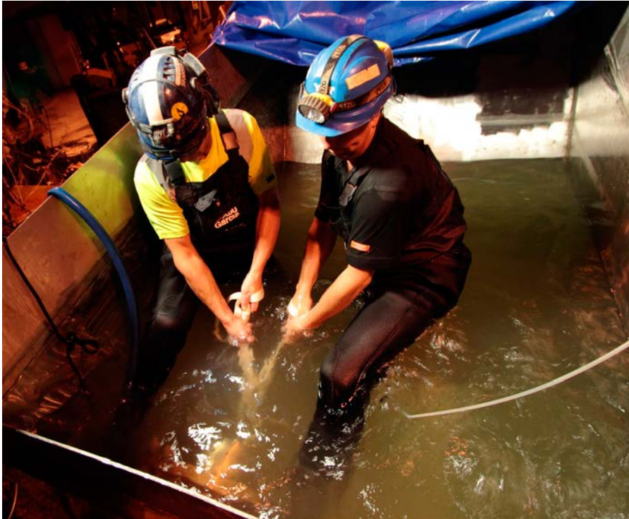
Figure 4-23. Stefan Grandin Svärth and Jonas Hallberg pulling out the steel cage from the KA3386A04 bore hole.
