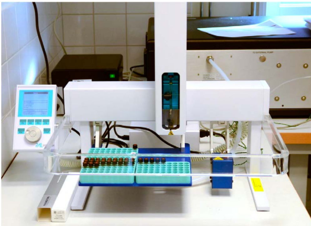
Figure 2-8. Liquid isotope analyzer and its inlet system.
