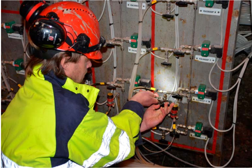
Figure 2-7. Borehole sections connections to the on-line experiment device in the tunnel.
