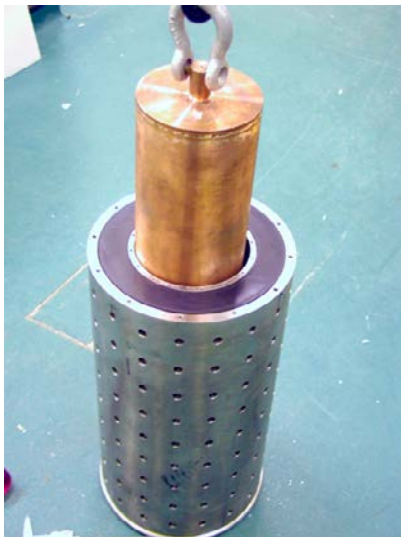
Figure 4-21. Model canister being lowered into support cage containing bentonite pellets in annulus.
