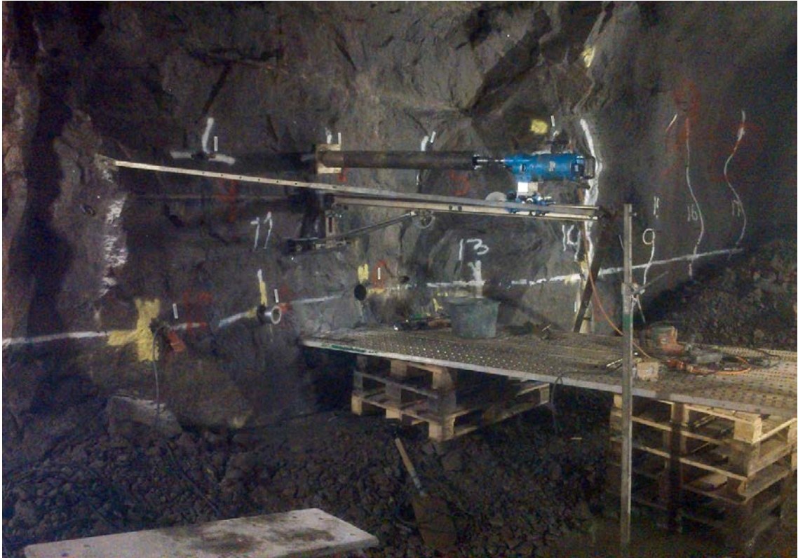
Figure 4-34. Overcoring of a horizontally emplaced rock bolt.
