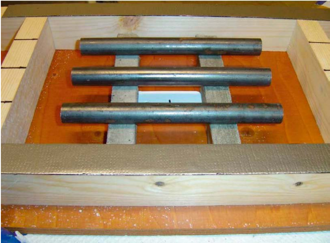
Figure 4-31. Mould and steel bars on support before casting.
