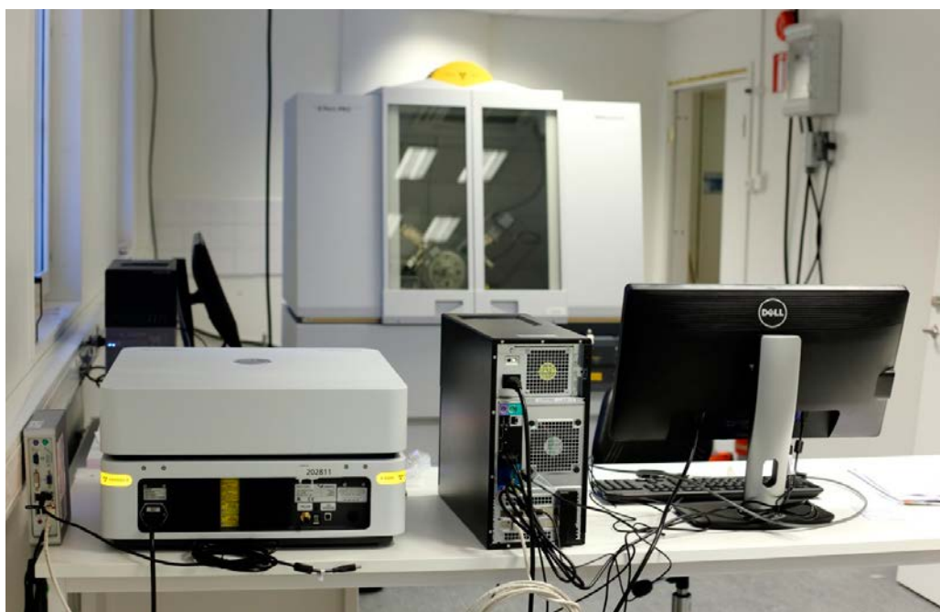
Figure 6-3. X-ray fluorescence spectroscopy and X-ray diffraction equipment in the material chemistry lab at Äspö for bentonite research and method development.
