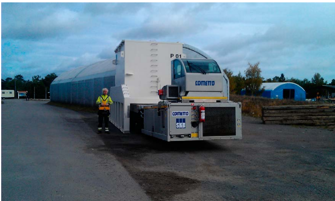
Figure 5-7. Ramp Vehicle carrying the modified ATB.
