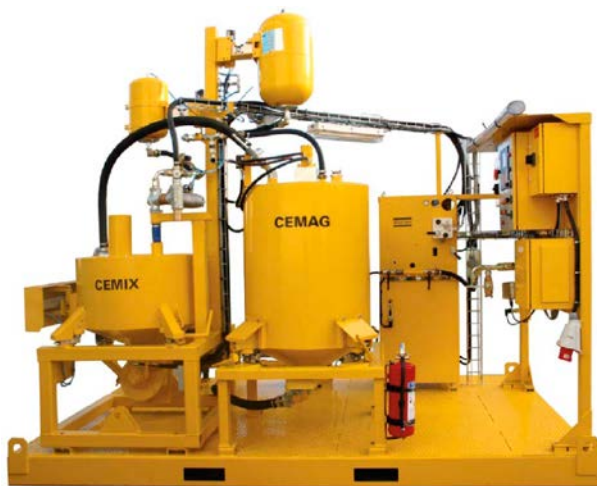
Figure 5-5. The Unigrout Equipment (EH22 200-140 AWB-SS) used in the Äspö Expansion.
