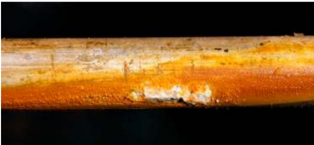
Figure 6-16. Local pitting in the outer aerobic part (KA3385A, area 3, outside section 2).
