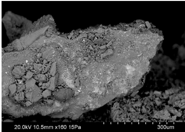
Back-scattered SEM image showing calcite with fine-grained FeS (bright) on the crystal surface.
