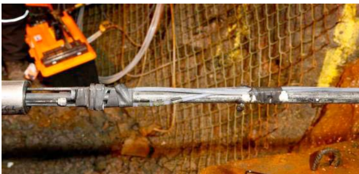
Figure 6-1. Photograph of rod, tubing, tape and stainless steel part of a packer in borehole KA3385A.
