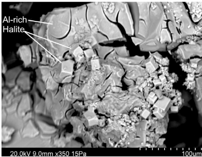
Back-scattered SEM image showing euhedral halite ( \text{NaCl} – cubic) on an Al-rich substance.
