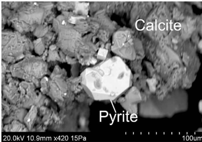
Back-scattered SEM image showing pyrite with calcite.
