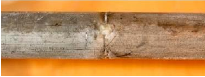
Figure 6-18. Local pitting in the inner anaerobic zones (KA3385A, area 2, section 2).
