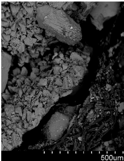
Back-scattered SEM image showing calcite (with variable c-axis to a-axes ratio).
