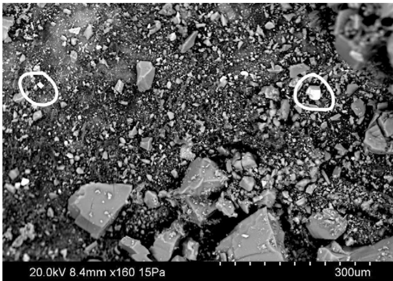
Back-scattered SEM image showing euhedral pyrite crystals (encircled) on the tape.
