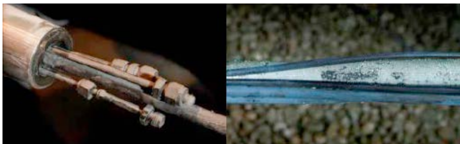
Figure 6-4. (Left) Photograph of grey precipitates (calcite-dominated) on packer steel connections. Sample 22111 (KA3385A). (Right) Photograph of grey precipitates (calcite-dominated) and black precipitates (sulphide-rich) on the Al-rod. Sample 22131 (KA3105A).
