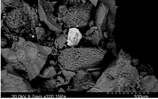
Back-scattered SEM image showing cubic pyrite (bright) with calcite.
