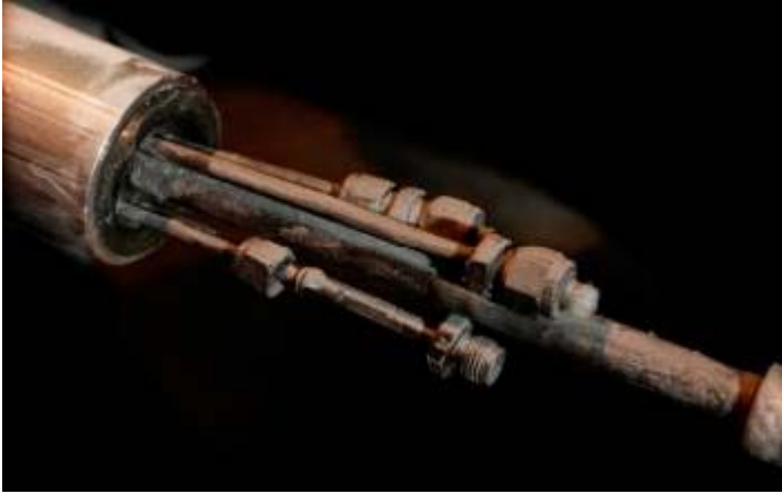
Photograph of location of sample 22111 (scraped off from packer connections).
