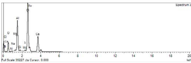
Spectrum 1: Gypsum, Spectrum 2: Gypsum+AlCl, Spectrum 3: Al-rich precipitate.
