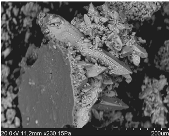
Back-scattered SEM image showing euohedral calcite.
