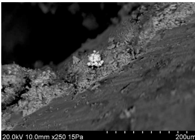
Back-scattered SEM image showing cubic pyrite (bright) on calcite.
