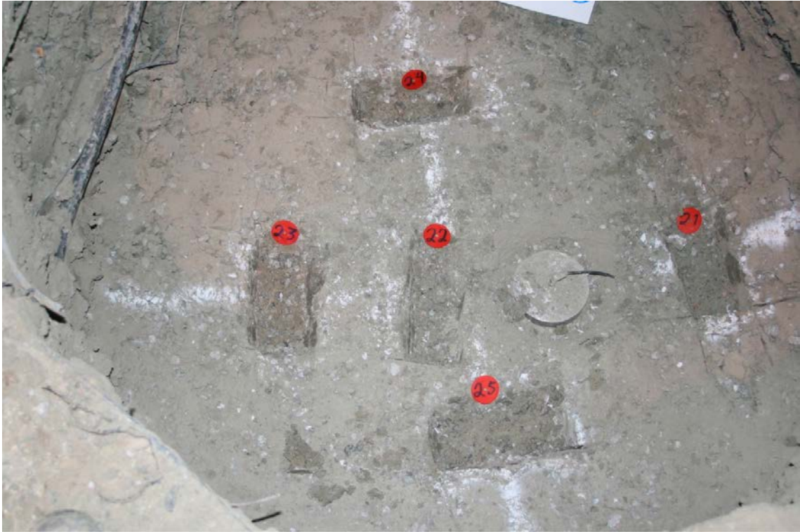
Figure 3-6. Samples taken from the tunnel backfill inside a deposition hole together with an installed sensor.
