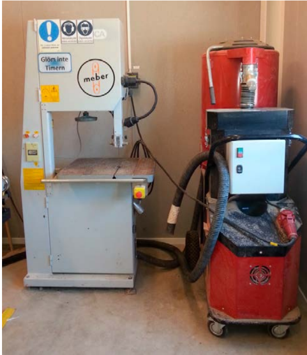
Figure 6-2. The band saw used for sawing the samples.
