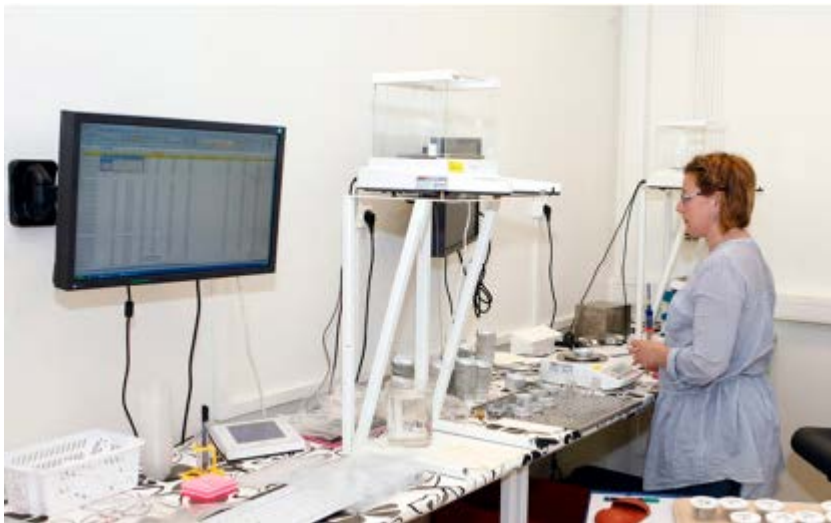
Figure 6-3. The equipment used for determining the density of the samples.
