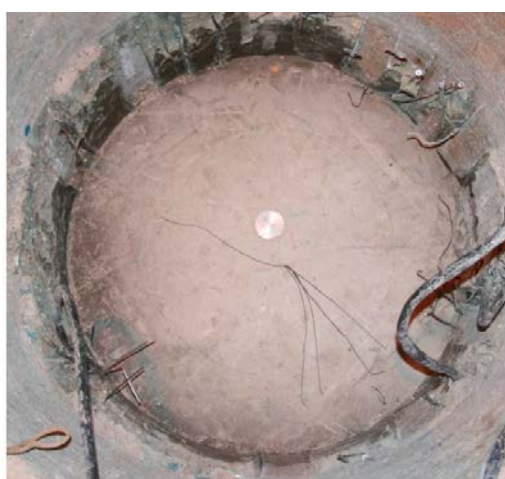
Figure 7-1. a) A total pressure sensor placed in block C3 in deposition hole 5. b) The vessel filled with water used for validating the total pressure sensors.
