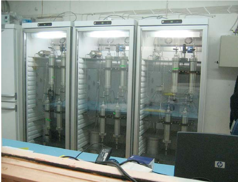
Figure 2-11. Three new circulation systems with stainless steel tubing were added to the Microbe laboratory in 2006.
