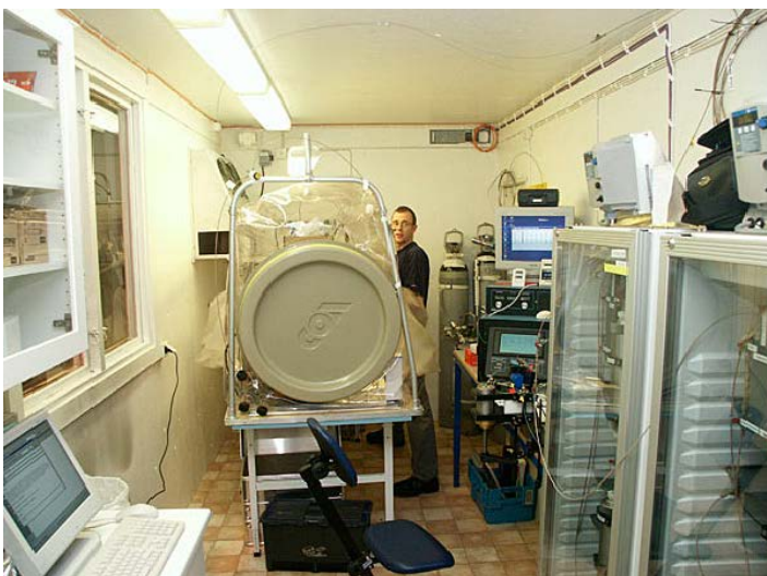
Figure 2-10. The microbiology laboratory environment at the 450-m site was originally equipped with three circulation systems with PEEK tubing (right), an anaerobic box (centre-left), an in situ gas extractor, and a Kappa 5 gas chromatograph (right of the anaerobic box).
