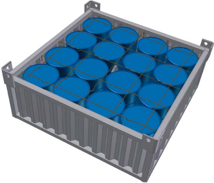
Figure 5-5. 3D-view of waste containers loaded with four trays with four drums each. Reinforcement bars on top of the drums also shown.
