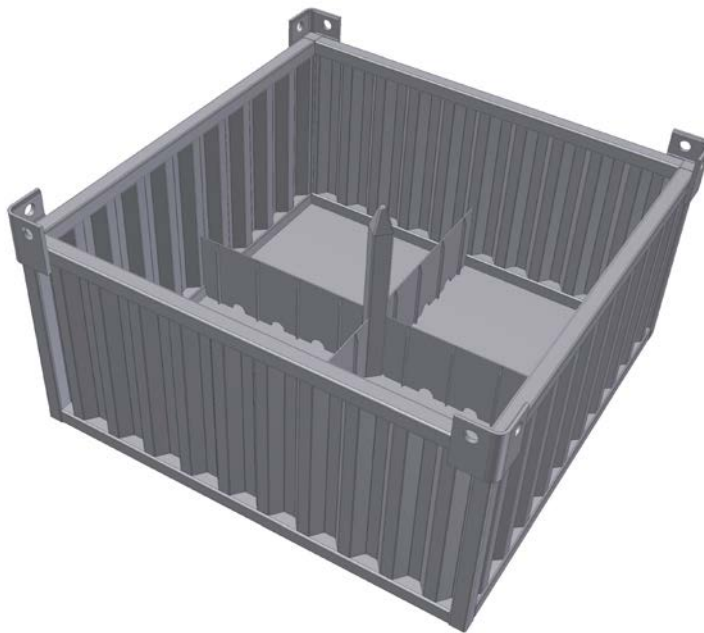
Figure 5-4. 3D-view of waste container for standard moulds when empty. The stiffening plates for the bottom plate and guides for the moulds are visible.
