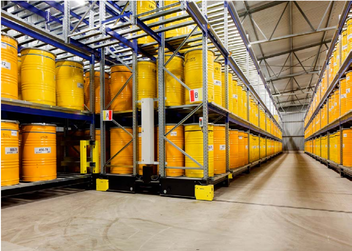
Figure 2-2. Current storage of drums at AB SVAFO after rebuilding of the storage and placing drums into 280-litre protection drums (Photo: SVAFO/Fredrik Ekenborg).
