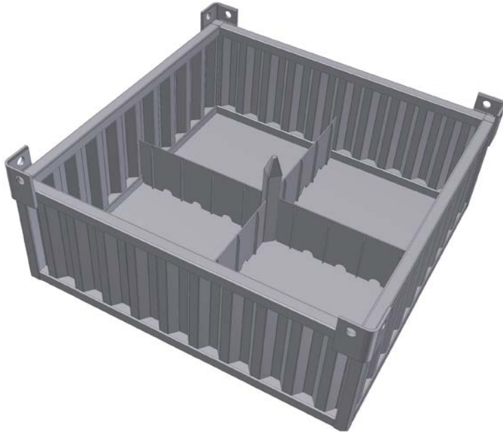
Figure 5-6. 3D-view of an empty waste container for standard 200-litre drums, showing the stiffening plates for the bottom plate and guides for the trays.
