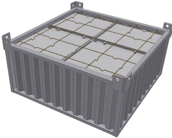
Figure 5-3. 3D-view of waste container loaded with standard moulds. Reinforcement bars on top of the moulds also shown.
