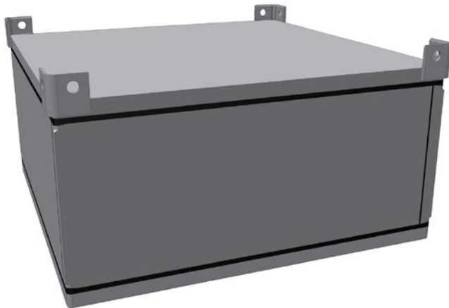
Figure 6-1. 3D-view of the long-term durable waste container with lid. The welds are shown (black).
