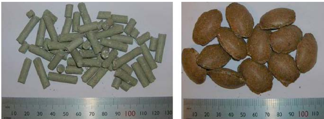
Figure 2-2. Left: IBECO extruded 6 mm diameter rods. Right: ASHA compacted almond shaped pellets.
