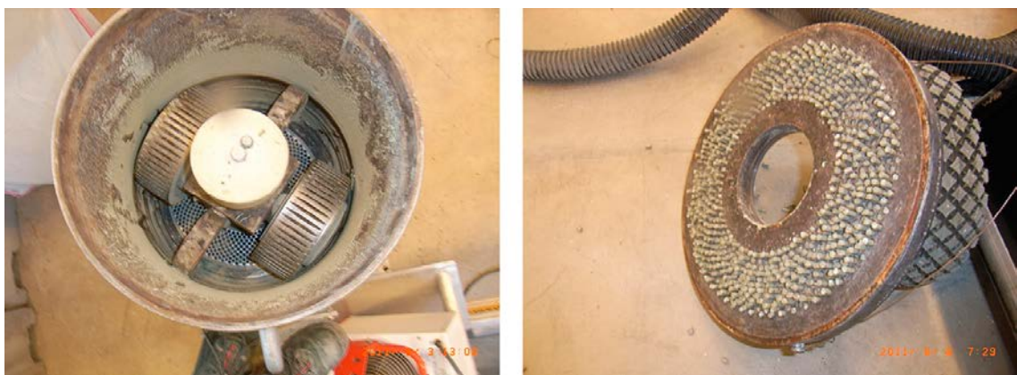
Figure 2-1. Left: pan grinder rolls over die. Right: die with material.
