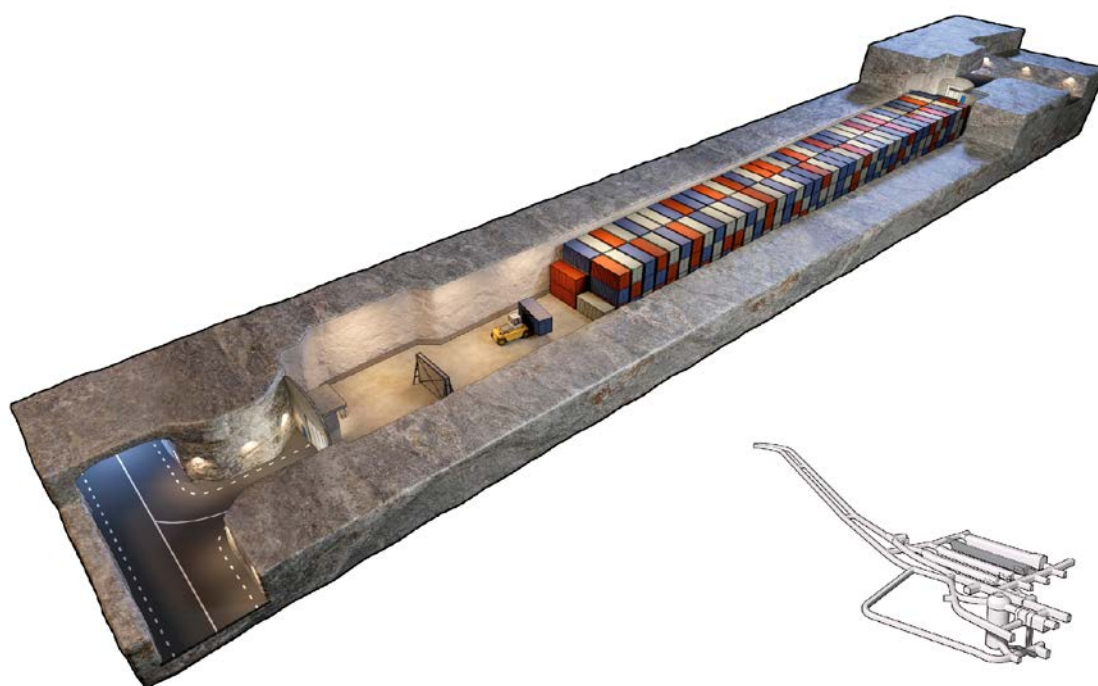
Figure 2-5. Picture showing the BLA vault.
