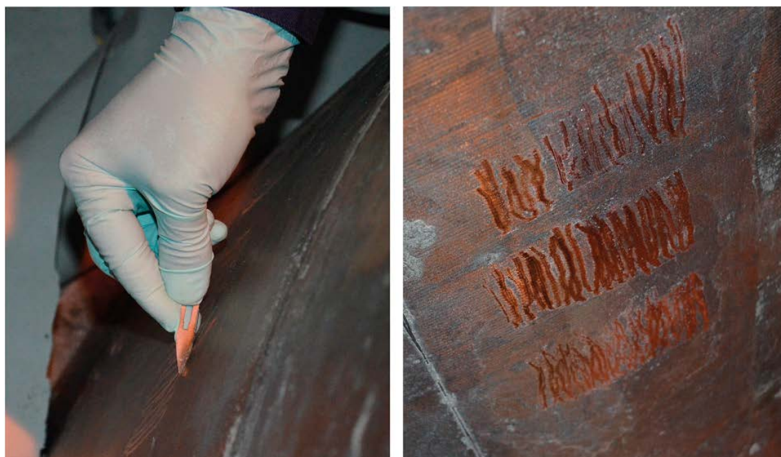
Figure 2-3. Left: The method whereby samples are scraped off the canister surface with a sterile scalpel. Right: The sampled area on the canister surface.
