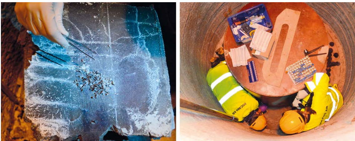
Figure 2-2. Left: The method whereby, using a sterile scalpel, bentonite samples are scraped off the buffer surface that had been in close contact with the copper canister. Right: The sampling site in deposition hole 6.
