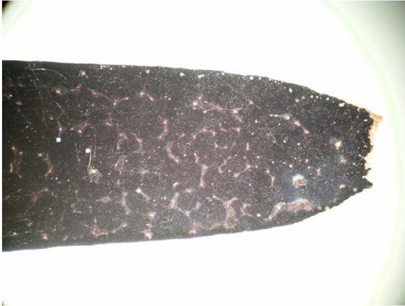
Figure A-1. Apparent granular network on the polished, unetched surface of sample SSRT-1 described in Table A-1. The gauge diameter was 3 mm.
