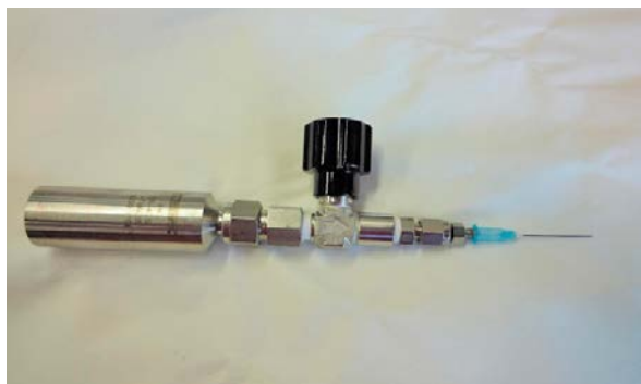
Figure 5-1. Cylinder used for transport of the gas sample. With courtesy of Ramboll Oy.
