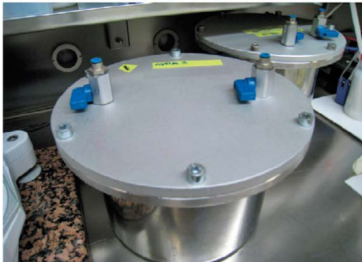
Figure A1-1. The test E-flasks are stored in a closed metallic vessel in the glove box.
