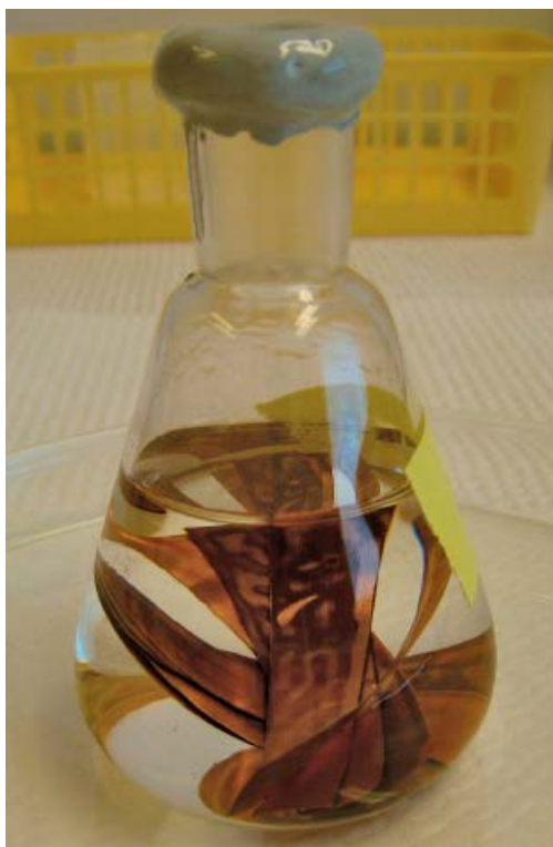
Figure A1-10. Cu5 test vessel after 116 days' reaction time (left), and after 344 days' reaction time (right) in air atmosphere.
