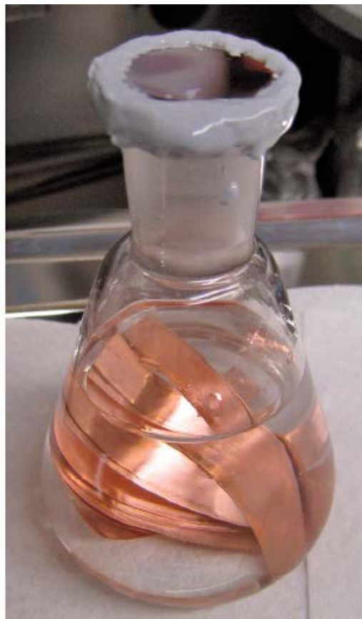
Figure A1-9. Cu2 (with glass stopper) and Cu3 (with Pd foil) test vessels after 292 days' reaction time N_2 atmosphere.
