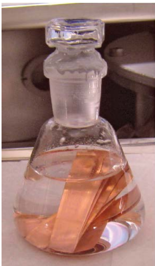
Figure A1-9. Cu2 (with glass stopper) and Cu3 (with Pd foil) test vessels after 292 days' reaction time N_2 atmosphere.
