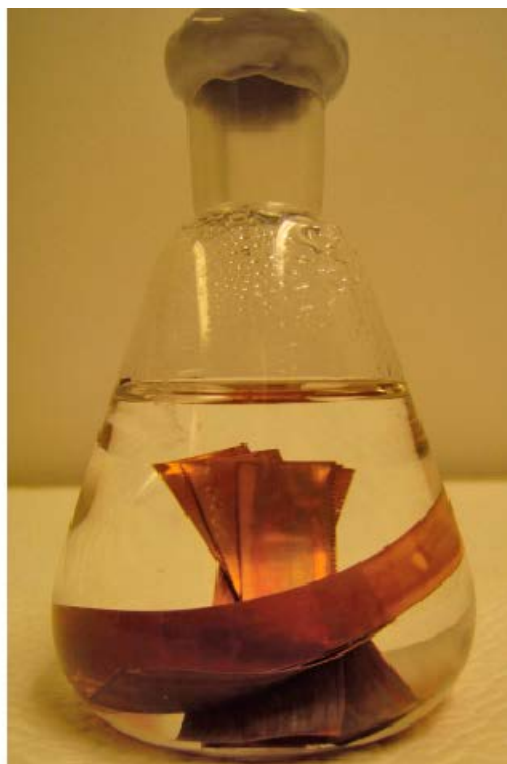
Figure A1-10. Cu5 test vessel after 116 days' reaction time (left), and after 344 days' reaction time (right) in air atmosphere.
