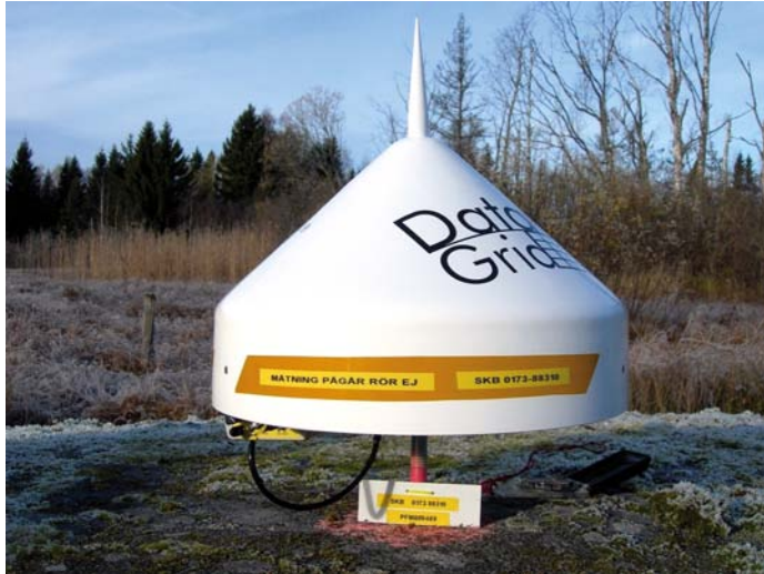
Figure 2-2. Sampling station at Forsmark with a choke ring antenna and GPS receiver mounted to the lower left. All stations are attached to a short steel rod anchored to the rock for good mechanical and thermal stability. From Gustafson and Ljungberg (2010, Figure 3-1).
