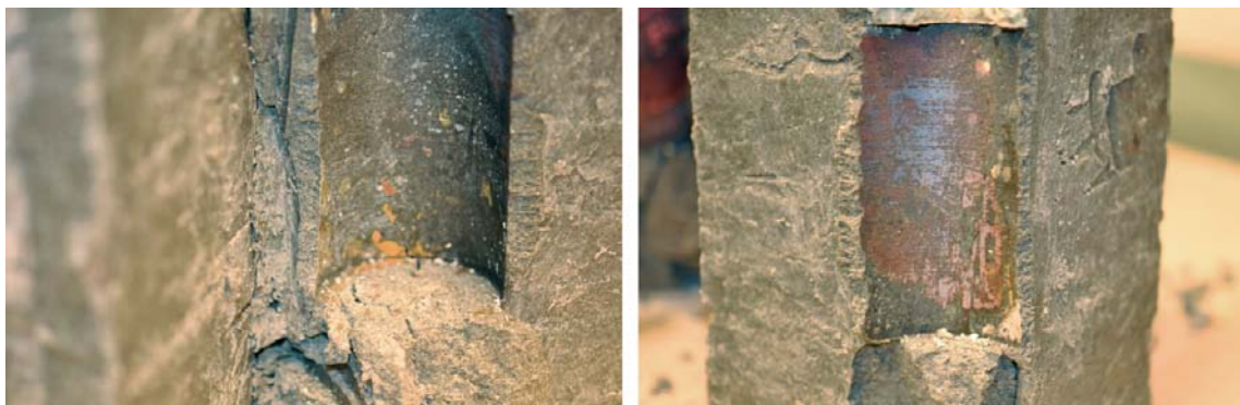
Figure 3-1. Corrosion products still remaining on adjacent bentonite after removal of the electrode.
