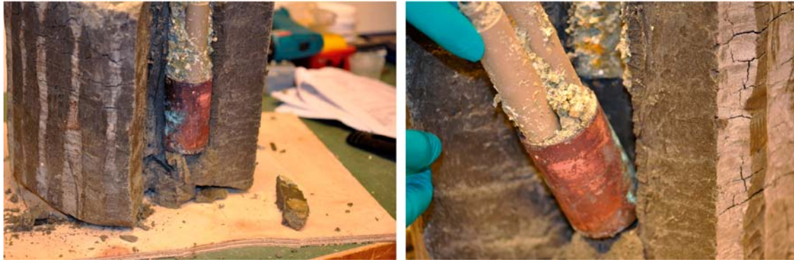
Figure 2-3. Removal of the copper electrode from the bentonite block. (Left) The copper electrode just about to be removed, and (right) being removed from the bentonite block.
