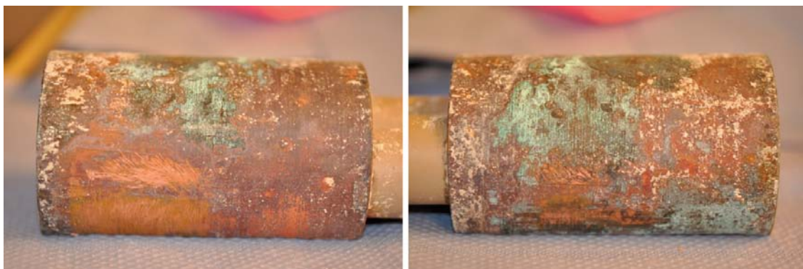
Figure 2-5. The two photographs show where corrosion products were scraped off from the copper electrode. (Left) Sample area H with mainly brownish and (right) sample area V with also blue-green corrosion products.
