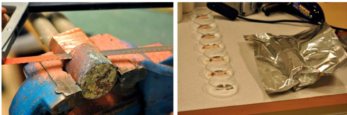
Figure 2-4. (Left) Cutting out samples from the copper electrode, and (right) temporary storage of samples from the copper electrode.
