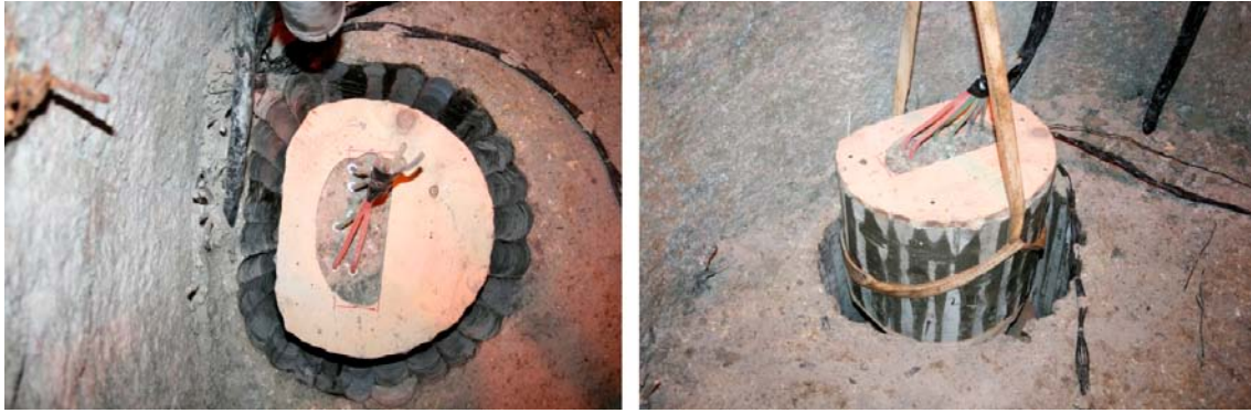
Figure 1-2. End result of stitch drilling around the copper electrodes in bentonite block C4 and uplift of the released smaller bentonite block.
