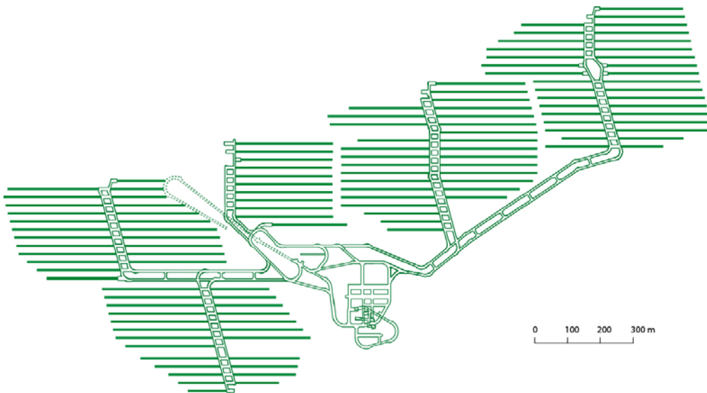
Figure 8-3. KBS-3H layout adaptation to the Olkiluoto site (Kirkkomäki and Rönqvist 2011). The layout area shown is between fracture zones R20 and R21, see Figure 8-4.
