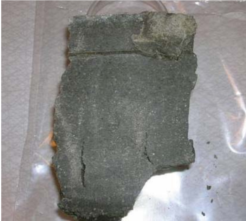
Figure 5-58. Photo of a sample showing the outer surface which has been in contact with the “rock”. Some small cracks can be seen.
