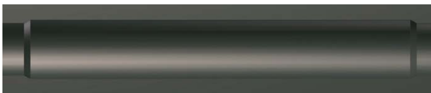
Figure 4-43. The drift would need to be reamed at the structural sealing position. The diameter would be increased from Ø1,850 millimetre to Ø2,075 millimetre.
