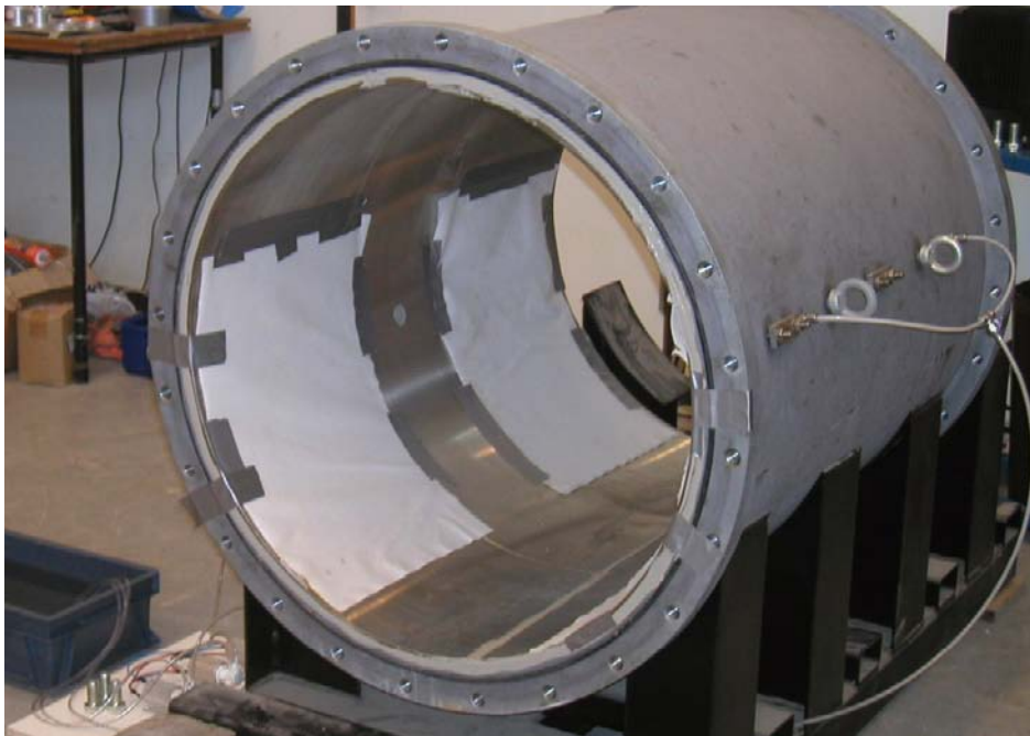
Figure 5-10. Four filter mats were positioned on the simulated drift surface. Each of the filter mats was connected to a tube into which a constant flow was applied.
