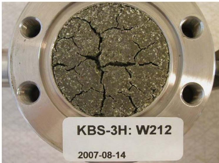
Figure 5-46. Photo taken after lifting the lid but with the specimen still inside the oedometer ring. (Initial water content 20% in the bentonite, slot width 5 mm and a salt content of 3.5% in the added water).
