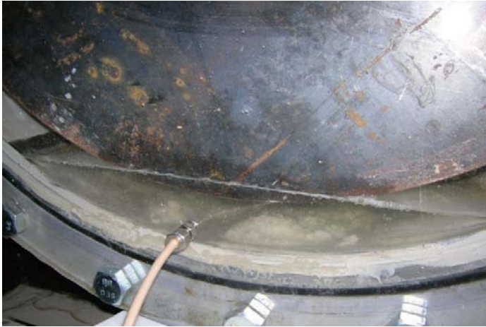
Figure 5-17. Picture taken before termination of the test. View from the water inlet side. The amount of bentonite on the drift floor had increased after two weeks so much that the outlet pipe was clogged and the water level rose above the Supercontainer base.
