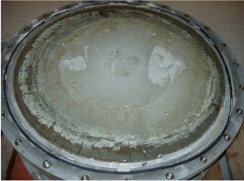
Figure 5-26. Desiccation of distance block in the BB experiment simulating the behaviour of distance block (using buffer with 10% water content, which is lower than nominal value for distance blocks) in a dry drift section. Photo shows one side of BB test set-up immediately after removing the lid. The radial desiccation cracking is seen clearly adjacent to the surface of the steel cylinder corresponding drift surface. Note that the block in this figure has first swollen and then desiccated when the water has been absorbed into the block. This has led to reduced water content at the periphery with cracking as a result.
