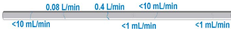
Figure 4-12. Case KBS-3H Median inflows drift of length 300 m. Inflows and inflow positions are shown.
