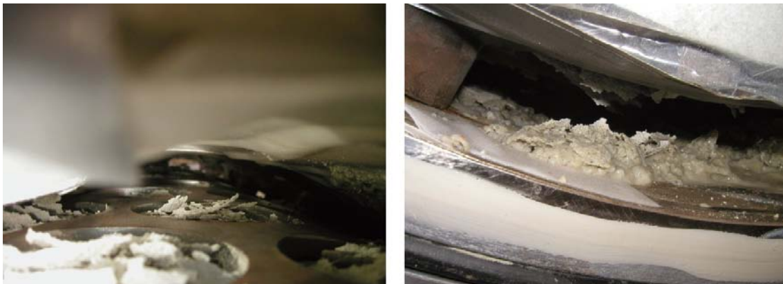
Figure 5-13. Flaking and accumulation of flakes of bentonite from the Supercontainer on the test cylinder floor. The pictures show the situation three days after starting the water circulation.
