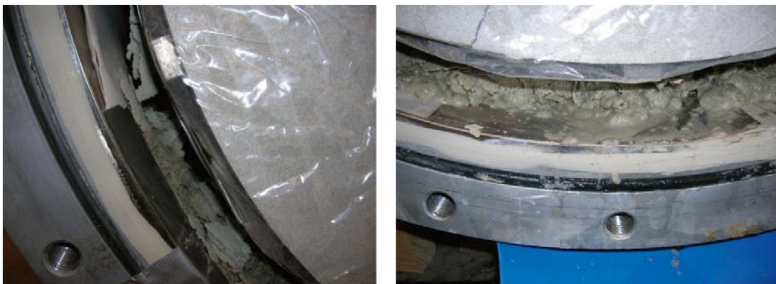
Figure 5-16. View of the slot between Supercontainer and “drift” after nine days of testing (note the large amount of material that had fallen into the slot).
