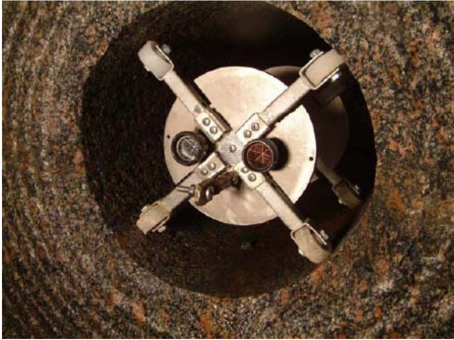
Figure 9-6. Device used for measuring the straightness of the pilot hole in the demonstration at Äspö.
