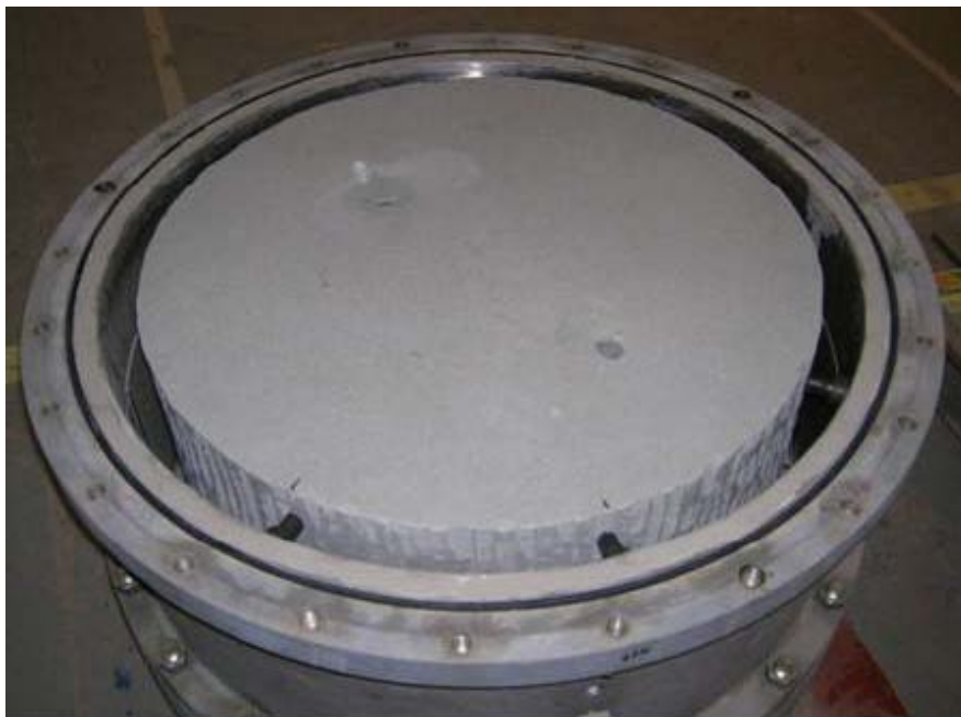
Figure 5-54. Bentonite block centred in the steel “drift” through the use of strong bolts.
