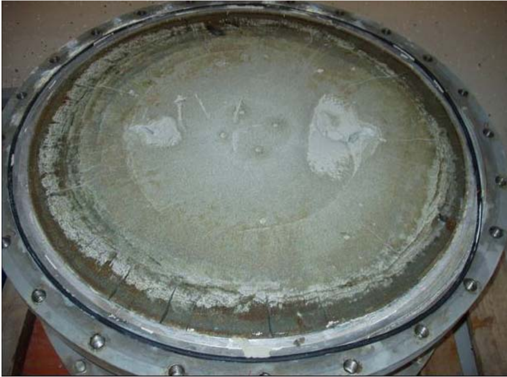
Figure 5-56. Photo showing one of the sides of the distance block immediately after removing the lid. The former slot is completely filled with bentonite.
