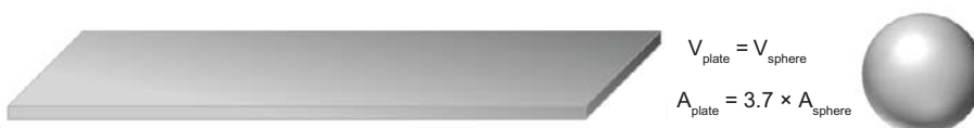
Figure 3-1. Schematic illustration of surface to volume ratio reduction of a cuboid shape ( 2 \times 20 \times 100 cm) to a spherical shape (radius = 9.8 cm). Note that the volumes of the objects are the same while the spherical object has a smaller surface area.
