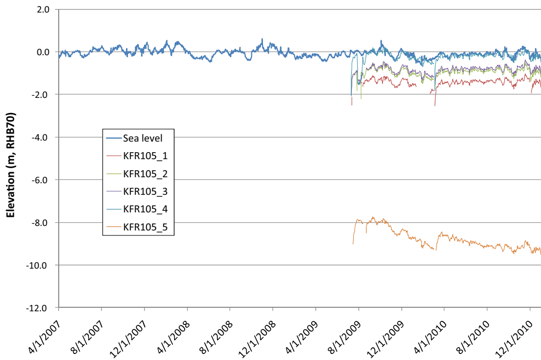
Figure F-10. Sea level fluctuation and calculated fresh -water head* for monitored sections in KFR105.
