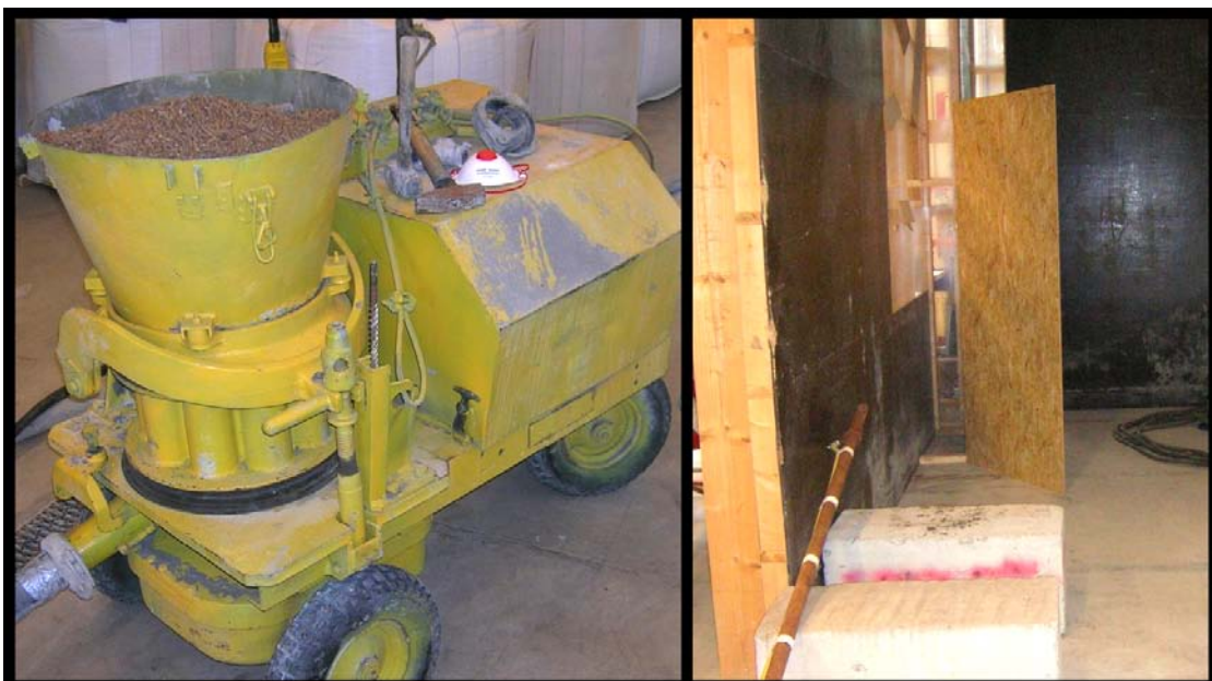
Figure 7-1. The shotcrete-equipment to the left and the shotcrete nozzle and the artificial slot to the right.
