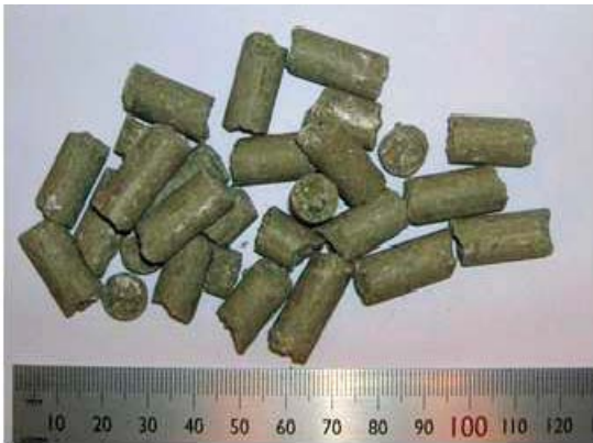
Figure 2-7. IBECO-14: 10 mm diameter extruded rods.
