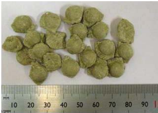
Figure 2-11. Posiva spec.-B compacted pillow-shaped pellets.
