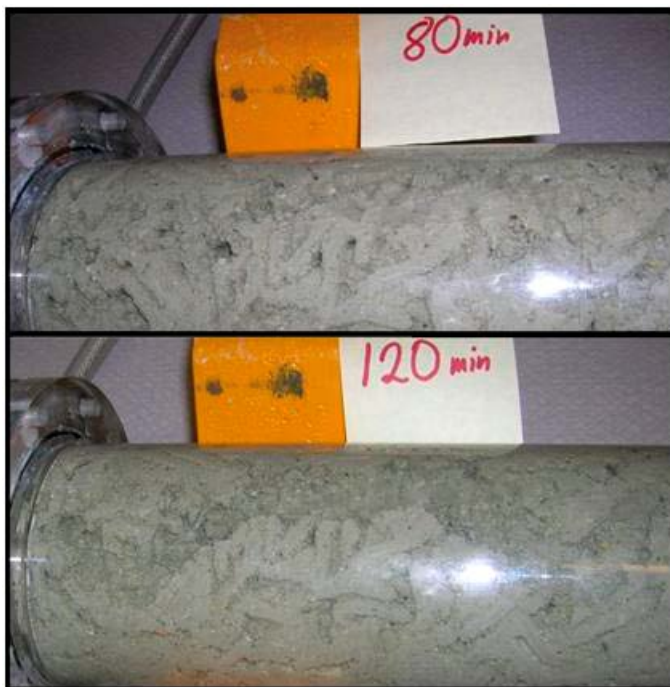
Figure 4-7. 6 mm extruded IBECO pellets at 1 l/min and 1% water salinity. In this test the flow channels are formed and stabilized after about 80 minutes, which corresponds to 80 liters accumulated flow.
