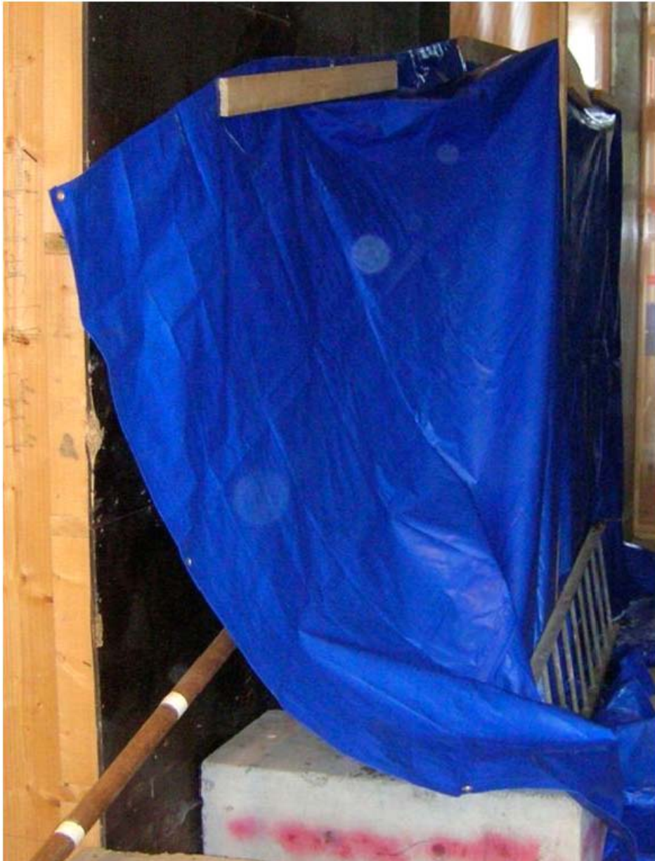
Figure 7-2. The arrangement was covered with a tarpaulin to avoid spreading of recoiling pellets fractions and dust.
