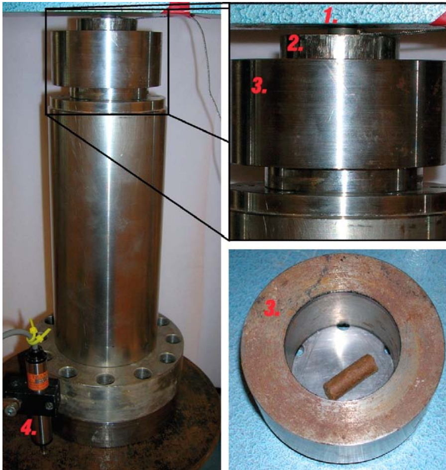
Figure 3-2. Test arrangement for the CRS-test on the individual pellets. The sample was placed in a steel cylinder (3). A piston (2) was placed on top of the sample. Load and deformation was logged with a load cell (1) and a deformation gauge (4).
