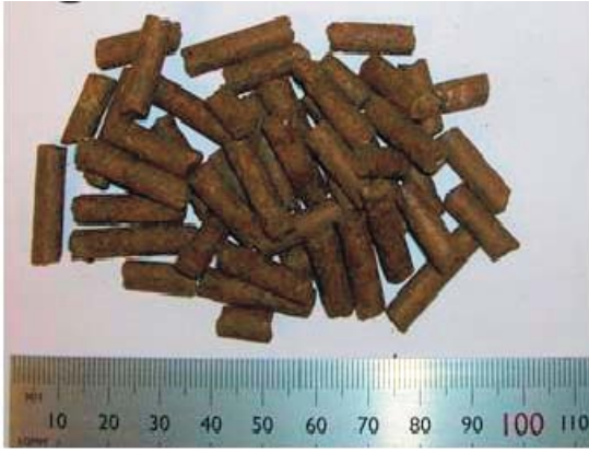
Figure 2-3. ASHA-13 extruded 6 mm diameter rods.
