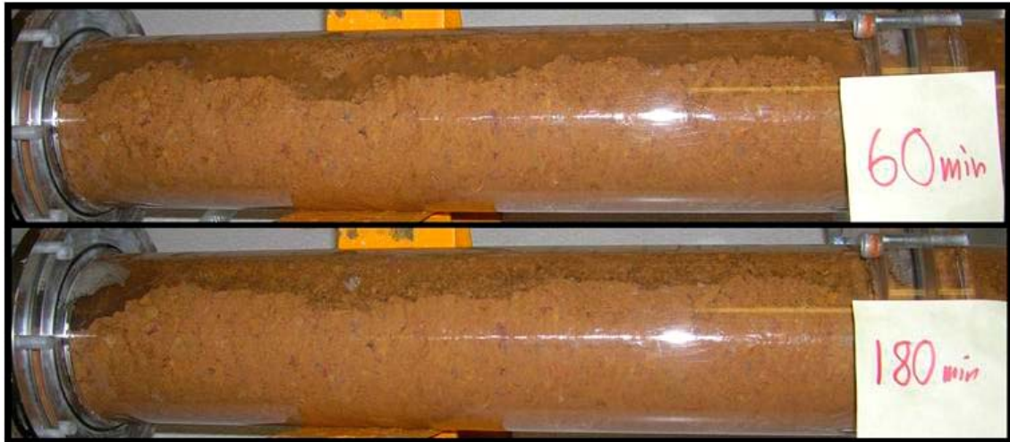
Figure 4-8. 6 mm extruded ASHA pellets at 1 l/min and 1% water salinity. A main flow channel is formed early and stays unchanged for the remainder of the test.
