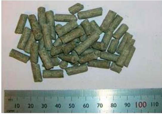
Figure 2-9. MX-80-13 extruded 6 mm diameter rods.
