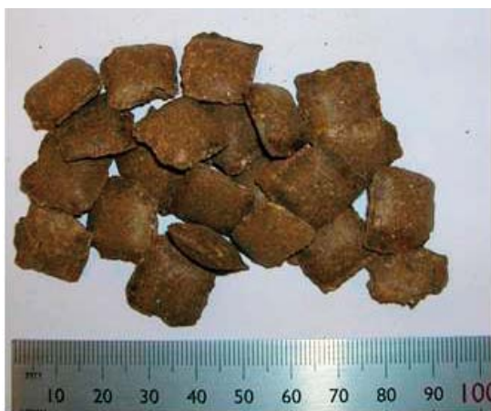
Figure 2-1. ASHA-11 compacted pillow-shaped pellets.
