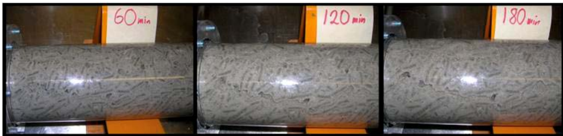
Figure 4-9. 6 mm extruded MX-80 pellets at 1 l/min and 1% water salinity. Several minor flow channels are formed early and stay unchanged for the remainder of the test.
