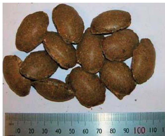
Figure 2-2. ASHA-12 compacted almond-shaped pellets.
