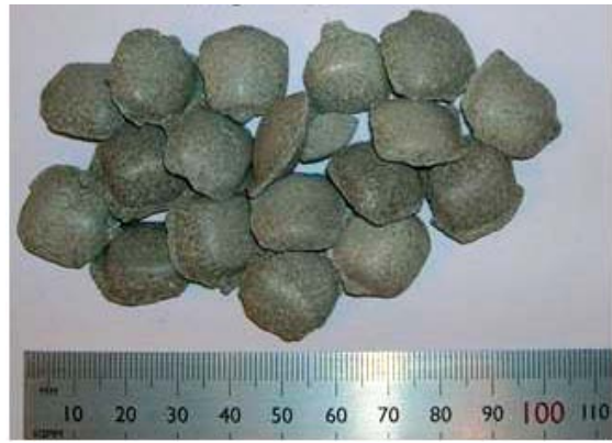
Figure 2-8. MX-80-11 compacted pillow-shaped pellets.
