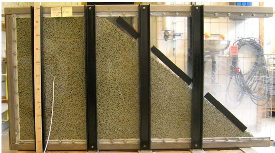
Figure 6-1. The slot used for the water storing capacity 2 tests. A point inflow was applied to the pellet filling in the slot at mid height. The wetting behavior, the inflow-outflow linkage and the water pressure was then registered.
