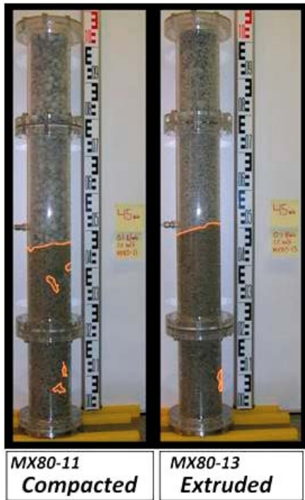
Figure 5-8. Comparison of extruded and compacted MX-80 at 0.1 l/min flow and 1% salinity after 45 minutes of water inflow.
