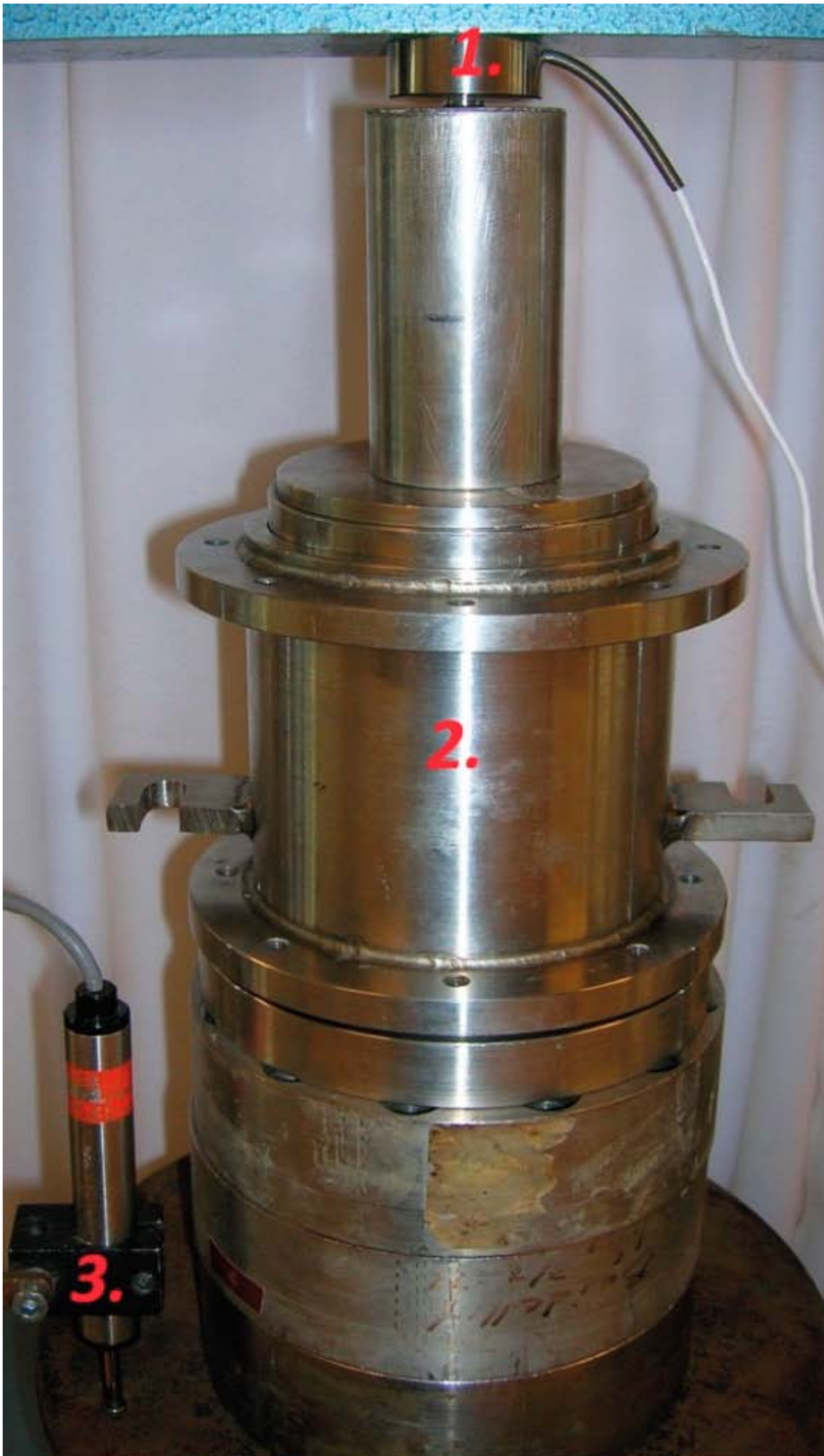
Figure 3-1. The arrangement of the CRS-tests. The load cell (1.) was placed at the top, the steel cylinder containing the pellets (2.) in the middle and the deformation gauge (3.) on the left side.
