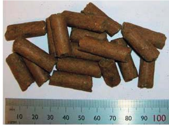
Figure 2-4. ASHA-14 extruded 10 mm diameter rods.
