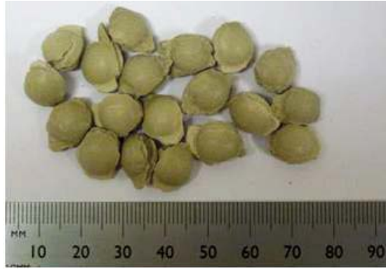
Figure 2-10. Posiva spec.-A compacted pillow-shaped pellets.
