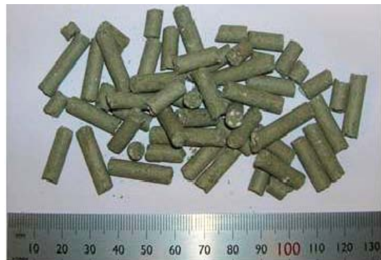
Figure 2-6. IBECO-13 extruded 6 mm diameter rods.
