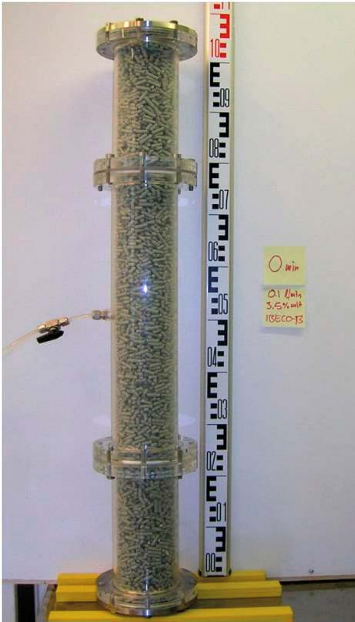
Figure 5-1. Arrangement for the water storing capacity type I tests. A point inflow was applied at mid-level. The inflow tube was led through the connector ending at the tube cross-section center in the middle of the pellet filling. The wetting of the pellet filling was visually surveyed and the water pressure logged by a transducer.
