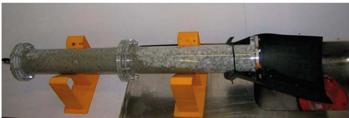
Figure 4-1. The arrangement of the erosion tests. A Plexiglas tube was filled with bentonite pellets. A constant inflow was applied from left to right. Samples were collected at the outflow and the amount of eroded material was determined through evaporation of the water in the samples.
