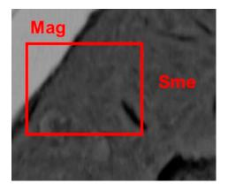
Figure 4-8. SEM observation image for case B (sample KINA 2-3). Mag: Magnetite, Sme: Smectite.
