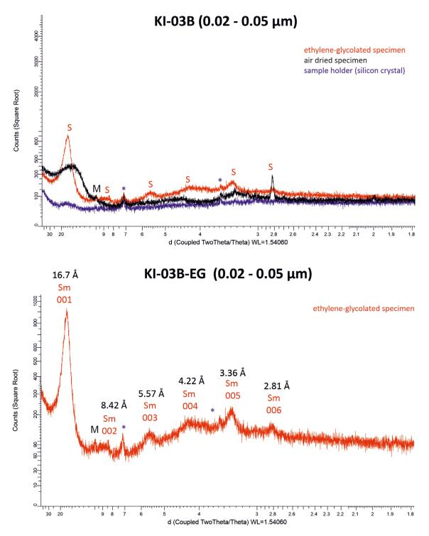
**Figure E-8.** X-ray diffractogram of air-dried and ethylene-glycolated oriented specimen of sample KI-03B and d-value of 00l peaks of montmorillonite (S, Sm). M = mica, \* = peaks from sample holder.
