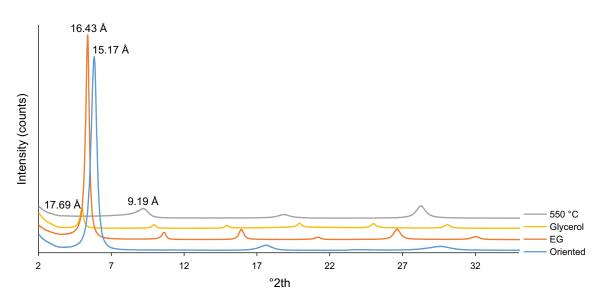
Figure 3-4. X-ray diffraction patterns of c65f8c clay-fraction and smectite d[001] peak positions.
