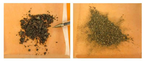
Figure H-2. Sample MD-2256 (LKAB 405-1194), left before drying, right after drying.
