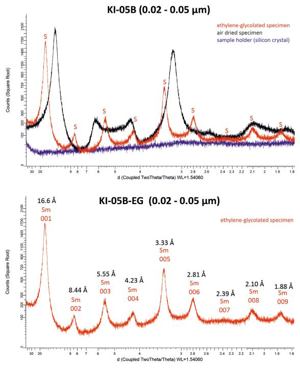
*Figure E-15.* X-ray diffractogram of air-dried and ethylene-glycolated oriented specimen of sample KI-05B and d-value of 00l peaks of montmorillonite (S, Sm).
