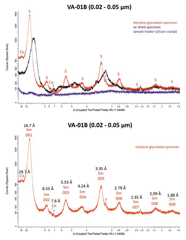
**Figure E-21.** X-ray diffractogram of air-dried and ethylene-glycolated oriented specimen of sample VA-01B and d-value of 00l peaks of montmorillonite (S, Sm). Co= corrensite, F = feldspar, \* = peak from sample holder.
