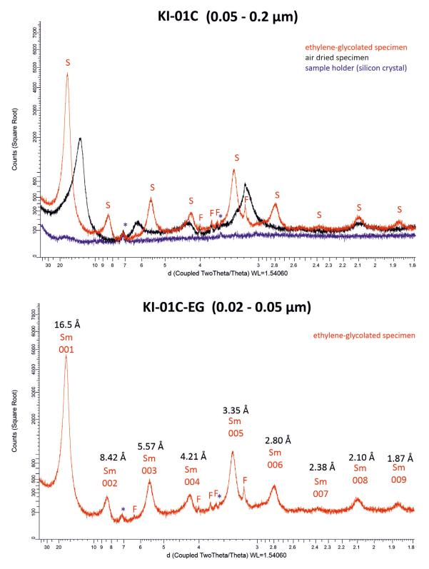
*Figure E-3.* X-ray diffractogram of air-dried and ethylene-glycolated oriented specimen of sample KI-01C and d-value of 00l peaks of montmorillonite (S, Sm). F = feldspar; \* = peaks from sample holder.
