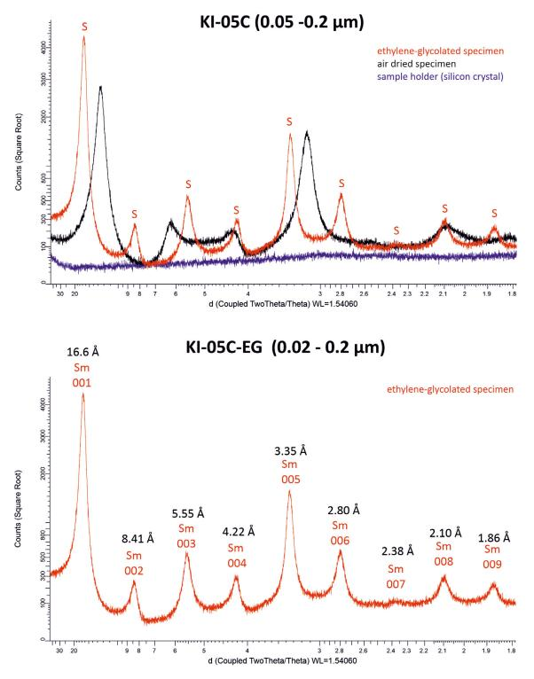
*Figure E-16.* X-ray diffractogram of air-dried and ethylene-glycolated oriented specimen of sample KI-05C and d-value of 00l peaks of montmorillonite (S, Sm).
