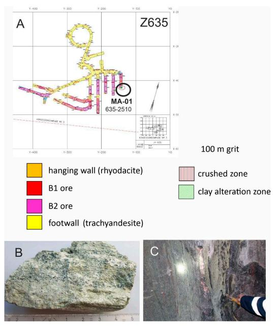
*Figure A-6.* Sample MA-01, a clay-altered gneiss from the Johannes ore body, Malmberget mine a) location, b) hand specimen and c) outcrop (images H.A. Gilg).
