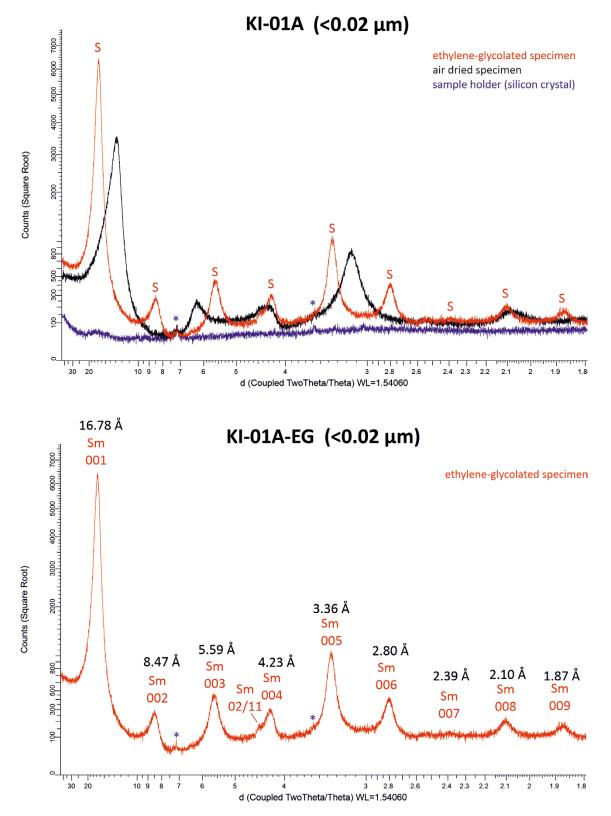
*Figure E-1.* X-ray diffractogram of air-dried and ethylene-glycolated oriented specimen of sample KI-01A and d-value of 00l peaks of montmorillonite (S, Sm). \* = peaks from sample holder.
