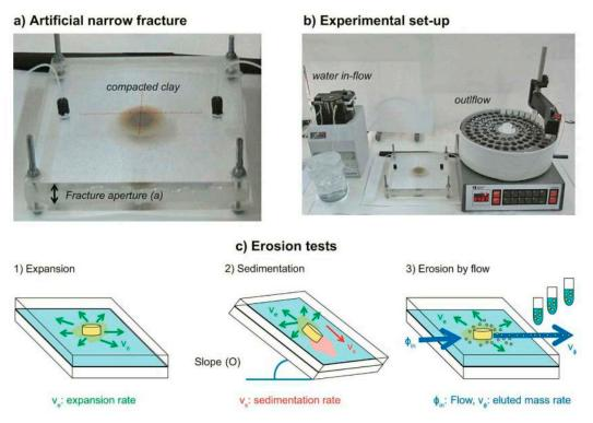
Figure 6-1. Experimental set-up of the erosion tests.
