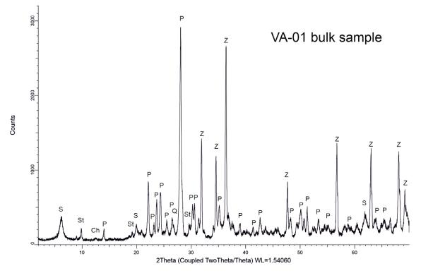
*Figure D-7. XRD* pattern of bulk sample VA-01. Ch: chlorite, P: albite, Q: quartz, S: montmorillonite, St: Stilbite, Z: zincite (added as internal standard at 20 wt%).
