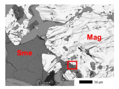
*Figure 11-2.* Magnetite-smectite boundary in sample KINA 2-2. Mag: Magnetite Sem: Smectite.
