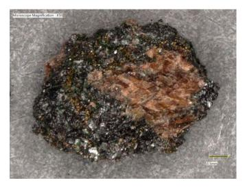
*Figure H-11.* Sample LL-1381 (LKAB 384-1137), potentially oxidised pyrite as indicated by the rust brown colouring of the sample. Scale bar bottom right.
