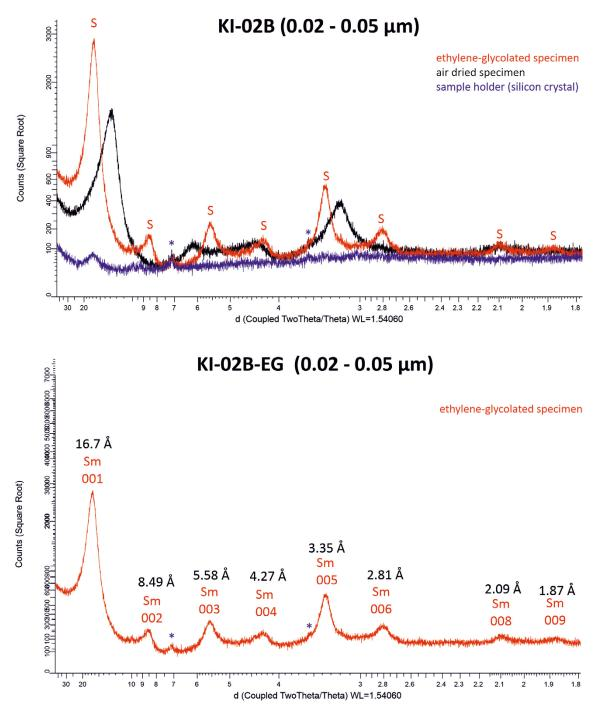
*Figure E-5.* X-ray diffractogram of air-dried and ethylene-glycolated oriented specimen of sample KI-02B and d-value of 00l peaks of montmorillonite (S, Sm). \* = peaks from sample holder.
