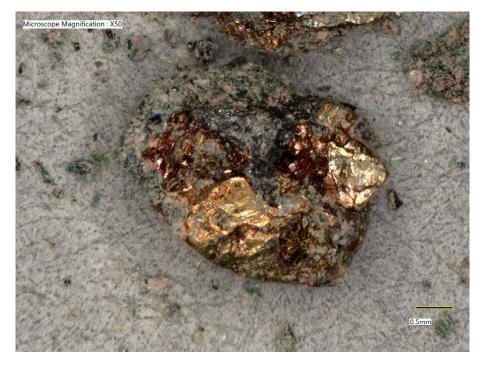
*Figure H-9.* Sample MD-2277 (LKAB 307-1165), note the clustered, aggregated nature of the sulphide (scale bar on bottom right).
