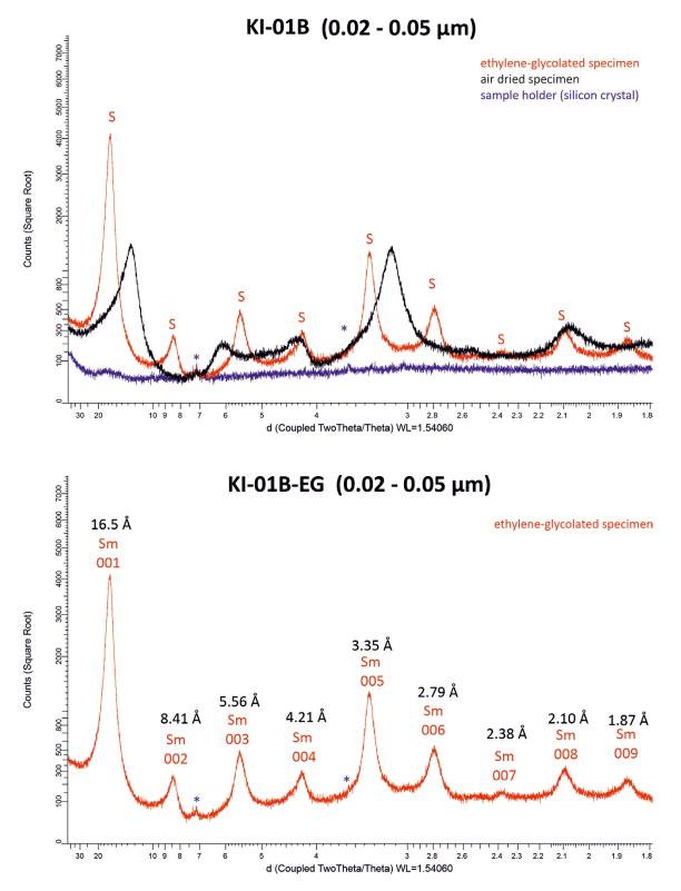
*Figure E-2.* X-ray diffractogram of air-dried and ethylene-glycolated oriented specimen of sample KI-01B and d-value of 00l peaks of montmorillonite (S, Sm). \* = peaks from sample holder.
