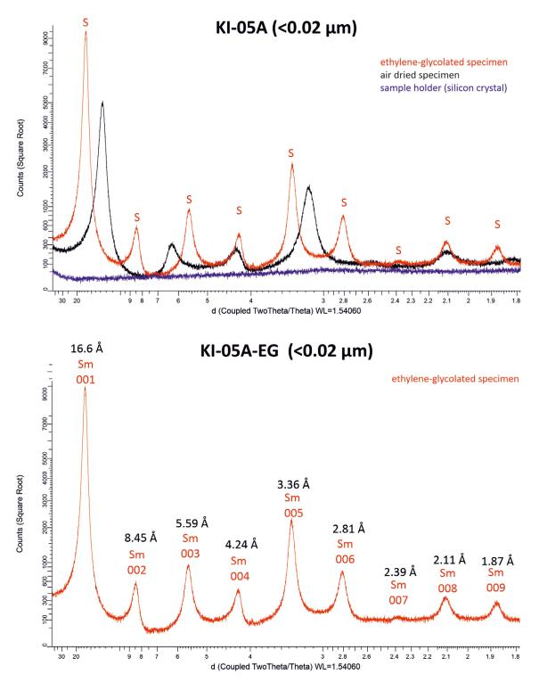
*Figure E-14.* X-ray diffractogram of air-dried and ethylene-glycolated oriented specimen of sample KI-05A and d-value of 00l peaks of montmorillonite (S, Sm).
