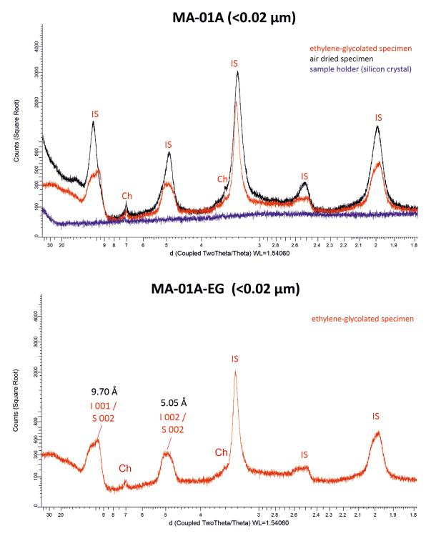
Figure E-17. X-ray diffractogram of air-dried and ethylene-glycolated oriented specimen of sample MA-01A and selected d-value of 00l peaks of R3 illite-smectite (IS). Ch = chlorite.
