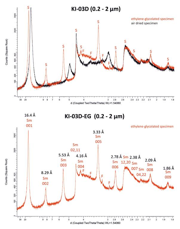
*Figure E-10.* X-ray diffractogram of air-dried and ethylene-glycolated oriented specimen of sample KI-03D and d-value of 00l peaks of montmorillonite (S, Sm). F = feldspar.
