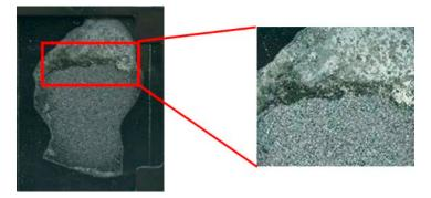
*Figure 4-3. KINA 2-2 thin section photomicrograph. Note that the iron ore (bottom half of the thin section, right) occurs as an aggregate.*
