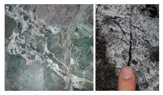
*Figure 2-5. a)* Incipient white clay alteration zone in rhyodacite of the hanging wall, level 1051 – crosscut 332, Kiirunavaara mine. Hammer in centre left of image for scale. b) Detail of clay alteration zone show-ing unaltered black magnetite veinlet. Images H.A. Gilg.
