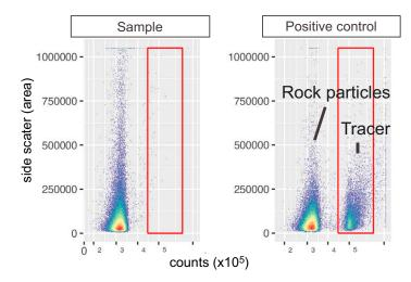
**Figure 5-5.** Flow cytometry results showing side scattering of a laser beam from all particles present in the sample against the count of the particles exhibiting fluorescence specific to the tracer used. The gate (red rectangle) indicates the area in which tracer particles could be detected (see the positive control spiked with the tracer in the figure on the right). No signal in the gate (left figure, sample) indicates that the sample is not contaminated.
