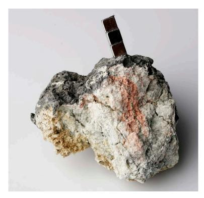
Figure 3-16. Smectite-magnetite interface in sample "Kiruna 2018" from the Kiirunavaara mine.
