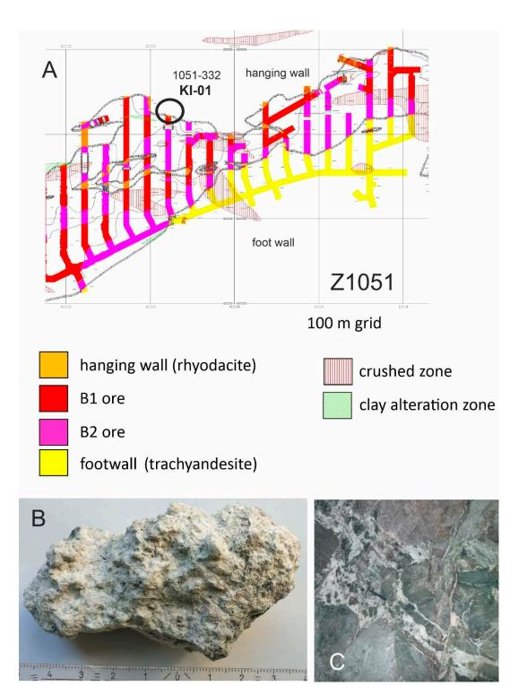
*Figure A-1.* Sample KI-01, a clay-altered hanging wall meta-rhyodacite a) location, b) hand specimen and c) outcrop (all images H.A. Gilg).
