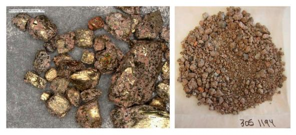
*Figure H-5.* Sample LL-1382 (LKAB 386-1194), left showing large single pyrite crystals (magnification note at top left), right wider view (NB no scale provided).
