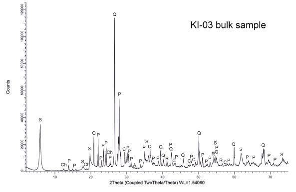
*Figure D-3.* XRD pattern of bulk sample KI-03. A: fluor-apatite, C: calcite, Ch: chlorite, P: albite, Q: quartz, R: rutile, S: montmorillonite.
