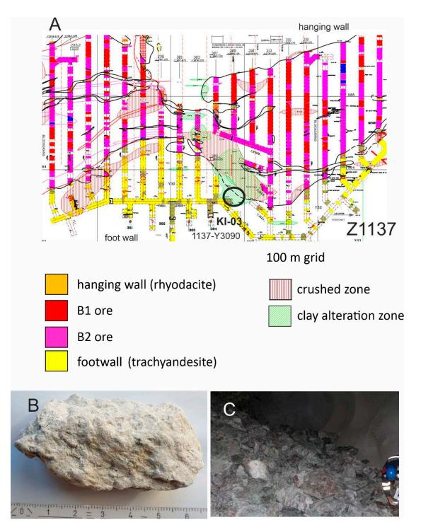
*Figure A-3.* Sample KI-03, a clay-altered footwall trachyandesite a) location, b) hand specimen and c) outcrop (images H.A. Gilg).
