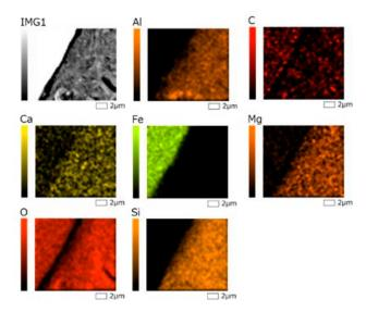
Figure 4-9. Elemental mapping analysis Results for case B (sample KINA 2-3).
