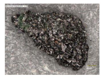
Figure H-12. Sample LL-1381 (LKAB 384-1137), magnetite in the bulk sample.
