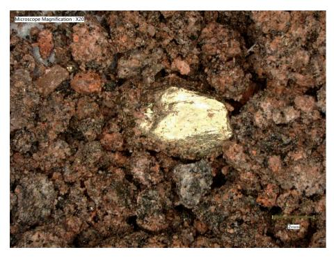
Figure H-4. Sample LL-1382 (LKAB 386-1194) showing large single pyrite (scale bar on bottom right).
