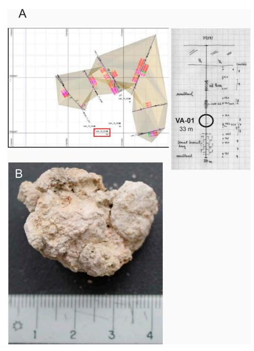
*Figure A-7.* Sample VA-01, a clay-altered metaandesite from the drill core 79001, Vahtanvaara prospect a) location and b) hand specimen (image H.A. Gilg).
