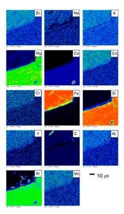
Figure 4-11. Elemental mapping analysis results for case B (sample KINA 2-3). Sme: Smectite, Mag: Magnetite.
