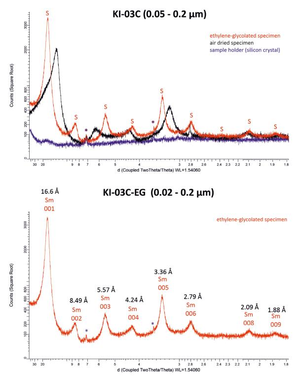
*Figure E-9.* X-ray diffractogram of air-dried and ethylene-glycolated oriented specimen of sample KI-03C and d-value of 00l peaks of montmorillonite (S, Sm). \* = peaks from sample holder.
