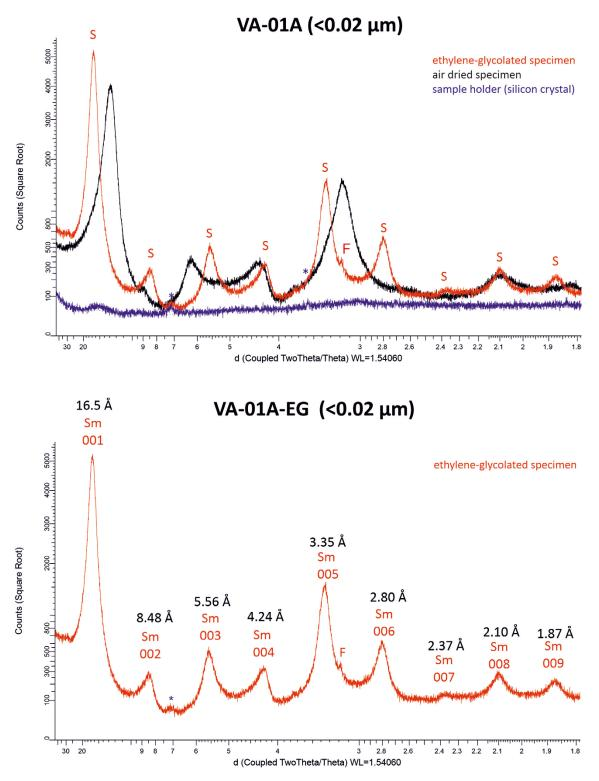
**Figure E-20.** X-ray diffractogram of air-dried and ethylene-glycolated oriented specimen of sample VA-01A and d-value of 00l peaks of montmorillonite (S, Sm). F = feldspar, \* = peak from sample holder.
