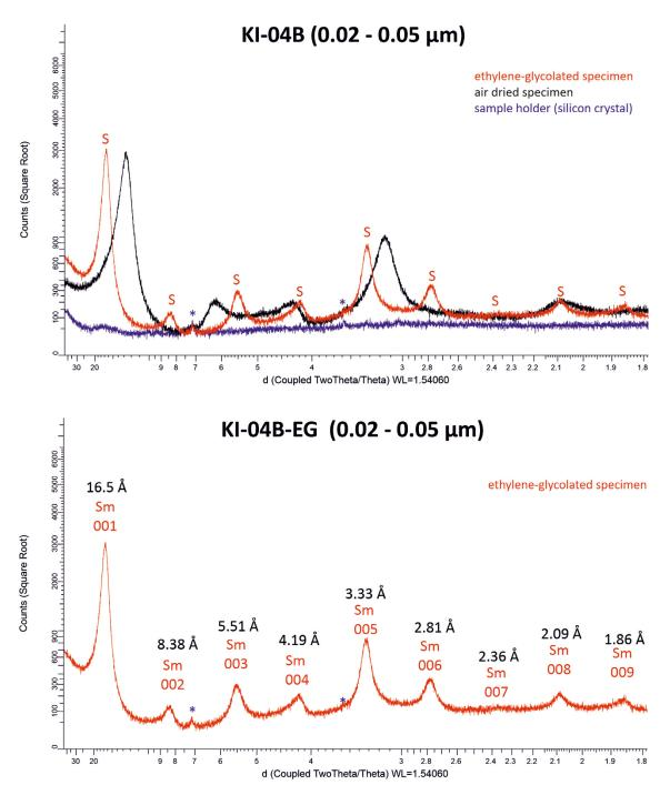
*Figure E-12.* X-ray diffractogram of air-dried and ethylene-glycolated oriented specimen of sample KI-04B and d-value of 00l peaks of montmorillonite (S, Sm). \* = peaks from sample holder.
