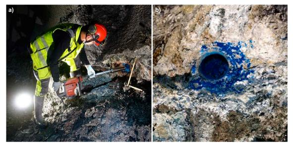
*Figure 5-1. a)* hand drilling short cores for clay samples, *b)* fluorescent tracer applied to the surface of the clay at the drilling location.
