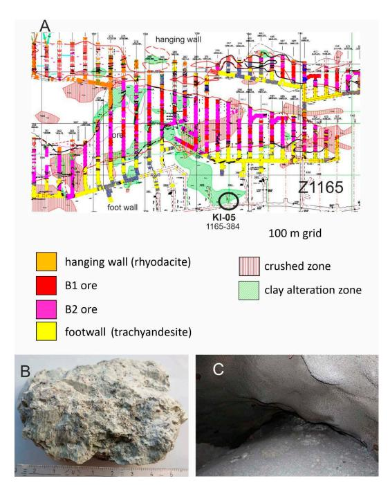
*Figure A-5.* Sample KI-05, a clay-altered footwall trachyandesite a) location, b) hand specimen and c) outcrop (images H.A. Gilg).
