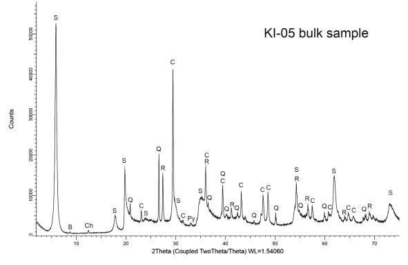
*Figure D-5. XRD pattern of bulk sample KI-05. B: phlogopite, C: calcite, Ch: chlorite, Q: quartz, R: rutile, S: montmorillonite.*
