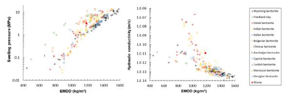
**Figure 3-5.** Comparison of swelling pressure and hydraulic conductivity of clay sample c65f8c (red dot) with bentonites and smectite clays of similar EMDD's and saturating solutions (0–11 gL<sup>-1</sup> TDS). Data for other bentonites and smectite clays are taken from Kiviranta et al. (2018) and references therein.
