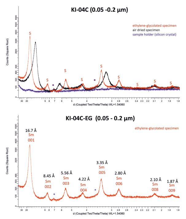
Figure E-13. X-ray diffractogram of air-dried and ethylene-glycolated oriented specimen of sample KI-04C and d-value of 00l peaks of montmorillonite (S, Sm). \* = peaks from sample holder.
