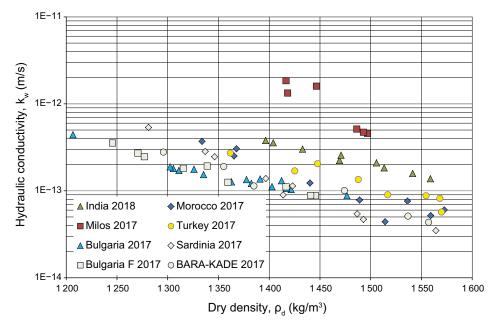
*Figure 3-14.* Determined hydraulic conductivity, measured with deionised water, as function of dry density for eight previously investigated bentonites (Svensson et al. 2019).
