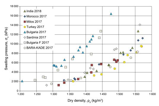
*Figure 3-15.* Determined swelling pressure, measured with deionised water, as function of dry density for 8 investigated bentonites (Svensson et al. 2019).
