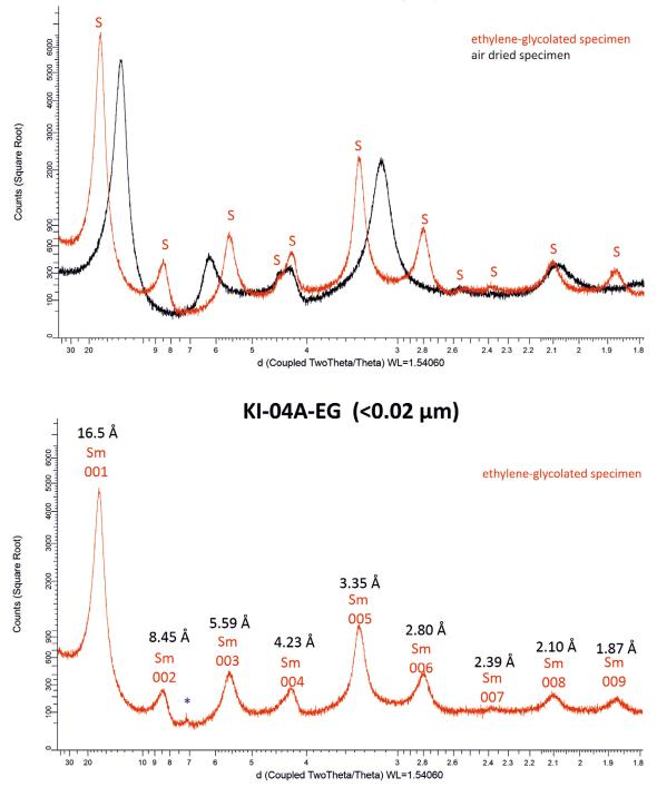
*Figure E-11.* X-ray diffractogram of air-dried and ethylene-glycolated oriented specimen of sample KI-04A and d-value of 00l peaks of montmorillonite (S, Sm). \* = peak from sample holder.
