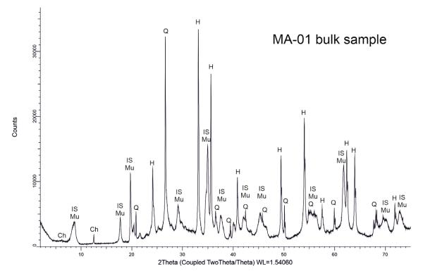
*Figure D-6.* XRD pattern of bulk sample MA-01. Ch: chlorite, IS: R3 illite smectite, H: hematite, Mu: muscovite, Q: quartz.
