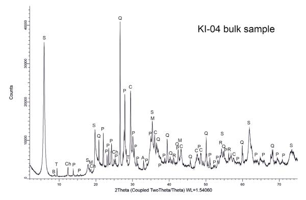
*Figure D-4.* XRD pattern of bulk sample KI-04. A: fluor-apatite, B: phlogopite, C: calcite, Ch: chlorite, M: magnetite, P: albite, Q: quartz, S: montmorillonite, T: talc.
