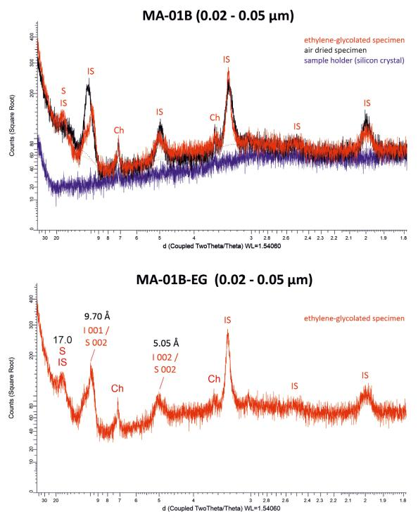
*Figure E-18.* X-ray diffractogram of air-dried and ethylene-glycolated oriented specimen of sample MA-01B and selected d-value of 00l peaks of R3 illite-smectite (IS). Ch = chlorite.
