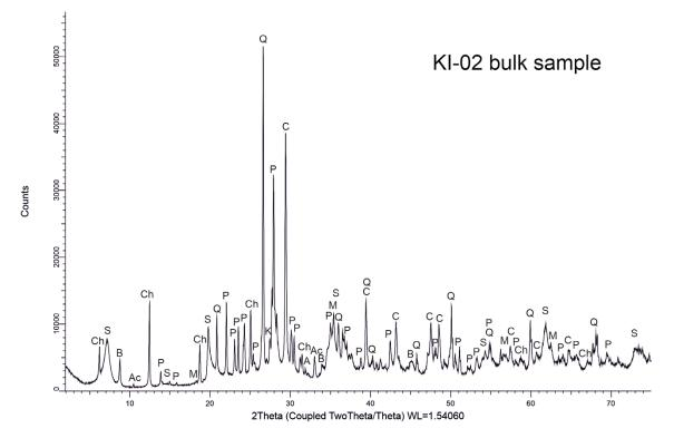
*Figure D-2.* XRD pattern of bulk sample KI-02. A: fluor-apatite, Ac: actinolite, B: phlogopite, C: calcite, Ch: chlorite, K: microcline, M: magnetite, P: albite, Q: quartz, S: montmorillonite.
