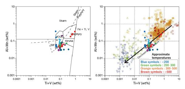
**Figure 4-12.** Discrimination diagram using trace element composition of magnetite with the trace element analysis results plotted in (Ti + V) vs (Al + Mn). After Nadoll et al. (2014). Note that the solid circles are the analytical results from this study, all other symbols are from Nadoll et al. (2014).
