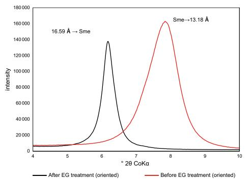
Figure 4-6. XRD results before and after EG treatment (oriented sample) for KINA 3-1.
