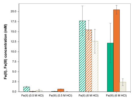
*Figure 5-3.* HCl extractable Fe (0.5M and 6M measured as ferrous or ferric Fe for the three types of clays. Figure colour coding is grayish white for sample 405-1194 (white clay), brown for 307-1223 (red clay) and green for 307-1165 (green clay).
