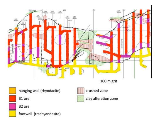
*Figure 2-4.* Geological map with outline of clay alteration within the iron ore body in an area of the southern part of the Kiirunavaara mine at level 1022 m. Block 30, level 1022.
