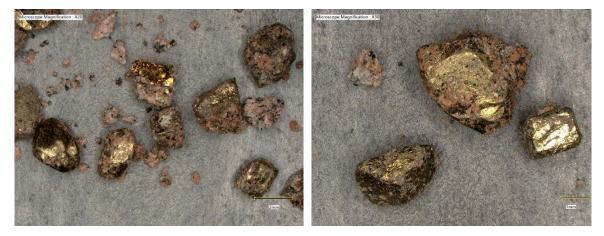
Figure H-6. Pyrite separates from sample MD-2278 (LKAB 386-1194). Scale bar bottom right.
