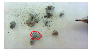
*Figure H-8.* Sample MD-2277 (LKAB 307-1165) indicating material used in the analysis (all but that piece circled in red). No scale bar, see picker tool on right.
