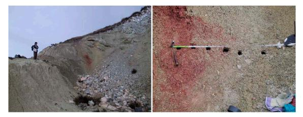
*Figure 1-2.* View of the bentonite sampling site at Cortijo del Aire, Almería, Spain (left). The red staining of the bentonite is clear during sampling (right). From Marcos (2004)
