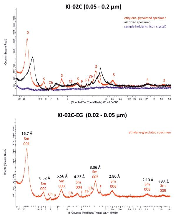
*Figure E-6.* X-ray diffractogram of air-dried and ethylene-glycolated oriented specimen of sample KI-02C and d-value of 00l peaks of montmorillonite (S, Sm). Ch = chlorite, F = feldspar.
