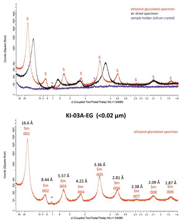
*Figure E-7.* X-ray diffractogram of air-dried and ethylene-glycolated oriented specimen of sample KI-03A and d-value of 00l peaks of montmorillonite (S, Sm). \* = peak from sample holder.
