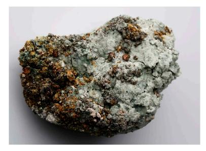
Figure 3-17. Kiruna smectite-pyrite interface (pyrite confirmed by XRD).
