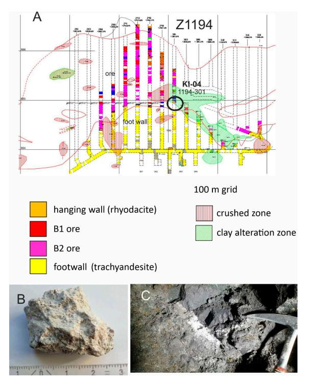
*Figure A-4.* Sample KI-04, a clay-altered footwall trachyandesite at contact to magnetite ore a) location, b) hand specimen and c) outcrop situation of (images H.A. Gilg).
