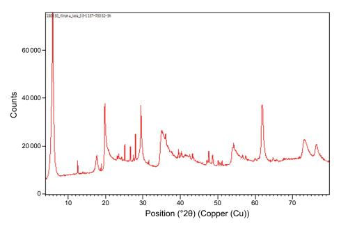
Figure 3-11. XRD pattern from a dry sample of the first batch of the Kiruna smectitic clay.
