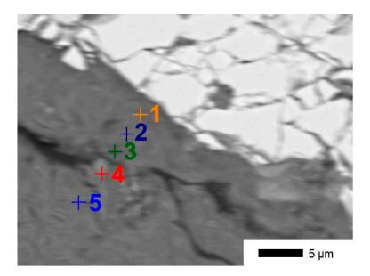
*Figure I1-3.* Sample KINA 2-2. SEM-EDS point analysis for smectite at the magnetite-smectite interface (analysis position).
