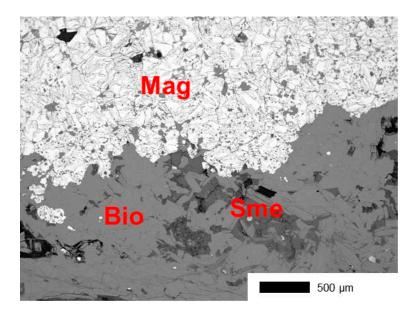
*Figure I1-1. Magnetite-clay interface in sample KINA 2-2. Mag: Magnetite Bio: Biotite Sem: Smectite.*
