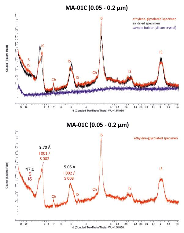
*Figure E-19.* X-ray diffractogram of air-dried and ethylene-glycolated oriented specimen of sample MA-01C and selected d-value of 00l peaks of R3 illite-smectite (IS). Ch = chlorite.
