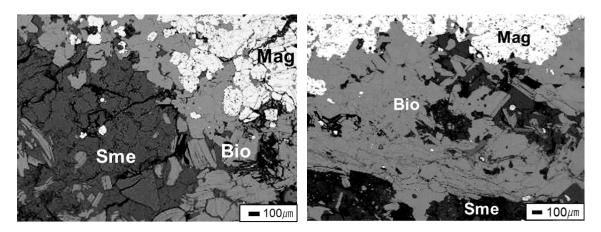
Figure 4-7. SEM observation image for case A (sample KINA 2-2). Mag: Magnetite, Sme: Smectite, Bio: Biotite.
