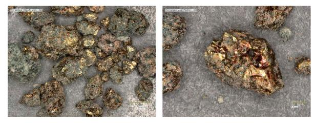
Figure H-7. Sample LL-1383 (LKAB 307-1165) showing variable pyrite habit. Scale bars bottom right.
