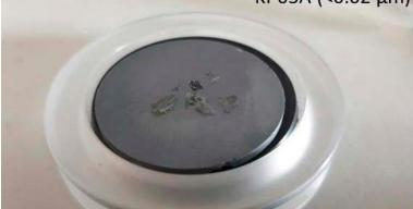
*Figure 3-1.* Photograph of XRD specimen with mounted flakes of sample KI-03A ( $< 0.02 \mu m$ ) on a Si single crystal (image H.A. Gilg).
