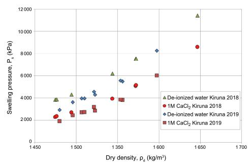
Figure 3-13. Swelling pressure in two sample batches (Kiruna 2018 and Kiruna 2019) of Kiruna clay.
