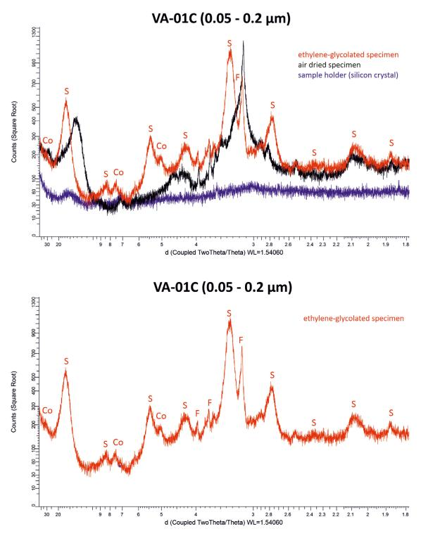
*Figure E-22.* X-ray diffractogram of air-dried and ethylene-glycolated oriented specimen of sample VA-01C. Co= corrensite, F = feldspar, S = montmorillonite, \* = peak from sample holder.
