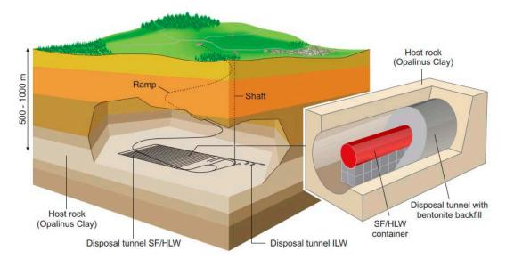
*Figure 1-1. Example of the multiple engineered barrier concept for radioactive waste disposal in steel canisters, with a bentonite backfill (Nagra 2002).*
