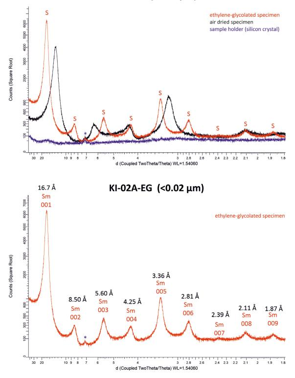
**Figure E-4.** X-ray diffractogram of air-dried and ethylene-glycolated oriented specimen of sample KI-02A and d-value of 00l peaks of montmorillonite (S, Sm). \* = peak from sample holder.
