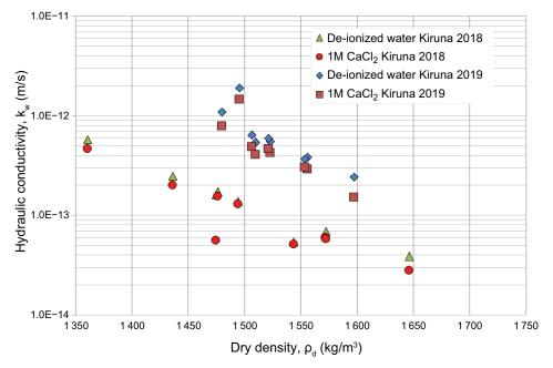
Figure 3-12. Hydraulic conductivity in two sample batches (Kiruna 2018 and Kiruna 2019) of Kiruna clay.
