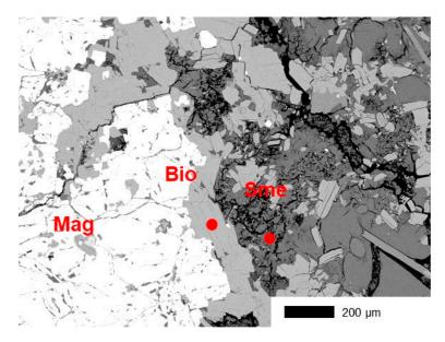
*Figure I1-4.* Sample KINA 2-2. SEM-EDS point analysis of biotite and smectite at the magnetite-biotite boundary at the magnetite-biotite boundary (red dots indicate positions of analyses). Bio: Biotite Mag: Magnetite Sem: Smectite.
