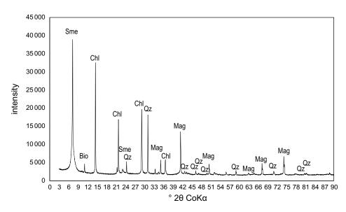
*Figure 4-5.* XRD results (random oriented sample) for KINA 3-1. Bio: Biotite, Ca: Calcite, Chl: Chlorite, Mag: Magnetite, Qz: Quartz, Sme: Smectite
