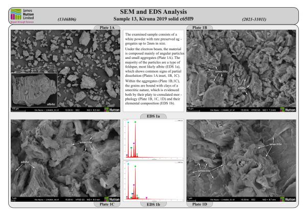
Figure 3-6. SEM images and EDS spectra of smectite-rich sample 134806 (KINA ID Kiruna 2019 solid c65ff9).
