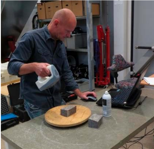
Figure C-5. Scanning a joint surface (not cast in formwork) using a hand-held scanner.
