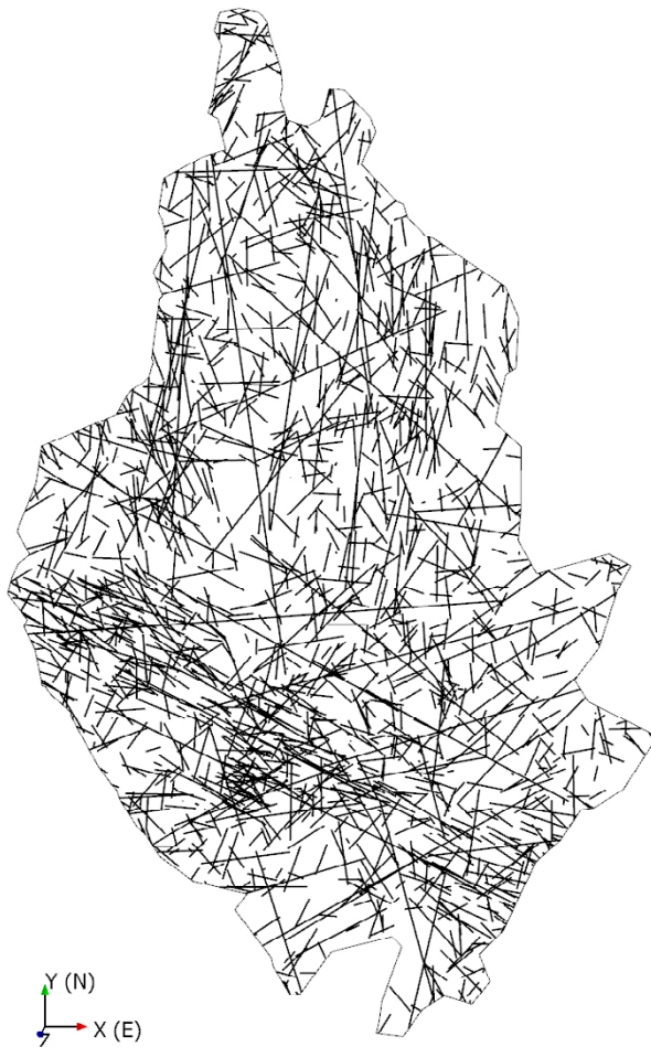
Figure 8-4. Example realisation of fracture traces modelled at AFM001702 for comparison with Figure 8-1.
