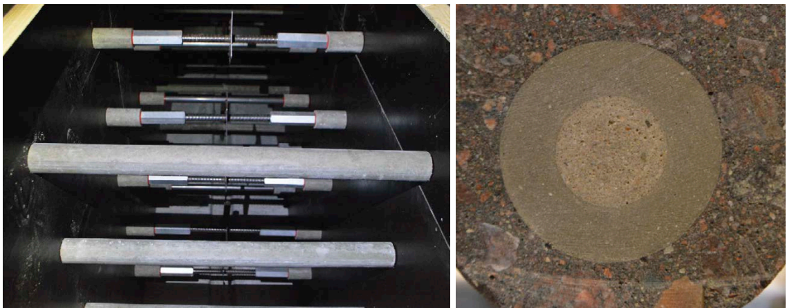
Figure 2-21. Test casting performed in order to evaluate different combinations of tie rods and protective tubes (left image) and a core extracted from this test (right image). In the right image, the filling material in the centre is surrounded by the concrete tube and the concrete used for casting of the test structure (Mårtensson 2021a).
