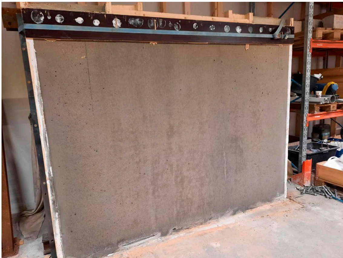
Figure 3-7. The photograph shows the New silo grout after pouring the grout into a slit with the same dimensions as the slit between the waste packages and the inner walls in the concrete silo. The distance between the container from which the grout was released and the floor shown in this picture was seven meters. (Holmberg 2021).
