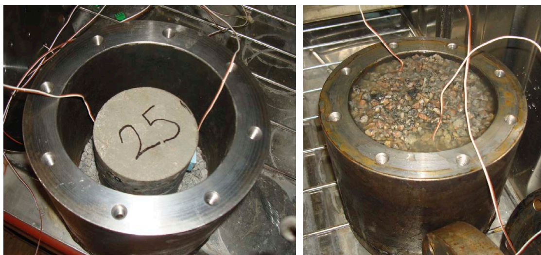
Figure 4-1. Experimental set-up for freezing of concrete samples under the influence of an external pressure. The picture on the left shows how the sample was placed in the container on a bed of gravel while the right one shows the container completely filled with water and gravel before the lid was attached.
