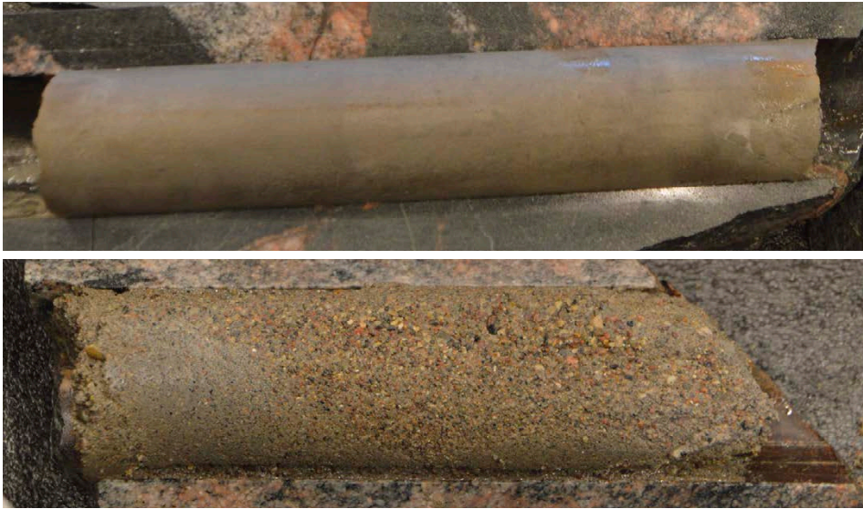
Figure 6-8. Two parts of the core made of SFR borehole concrete extracted from a depth of about 220 meters showing a zone which has been enriched in cement (upper picture) and a zone which has been depleted from cement (lower picture) (Mårtensson 2019).
