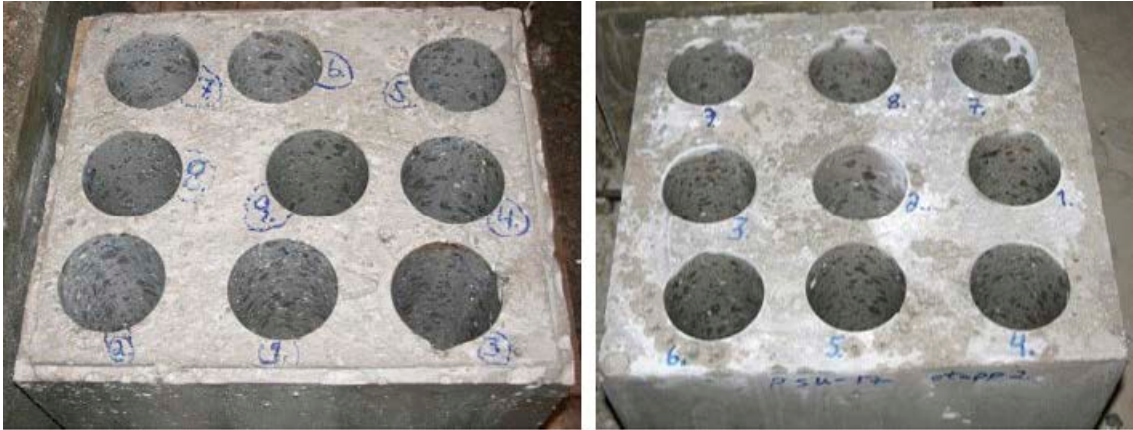
Figure 3-2. The small cubes manufactured just after finishing of the two castings performed by Mårtensson and Vogt (2019) from which cores used by Villar et al. (2019) were extracted.
