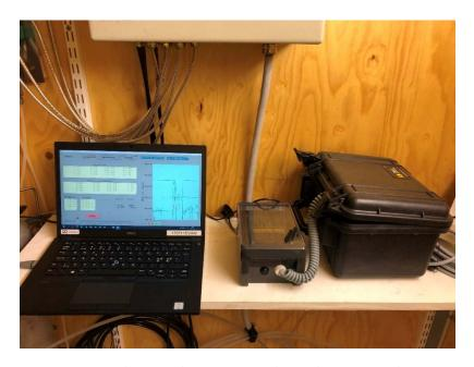
Figure 3-6. Data logger with transportation box and computer with on-measurements in the FLUO program.
