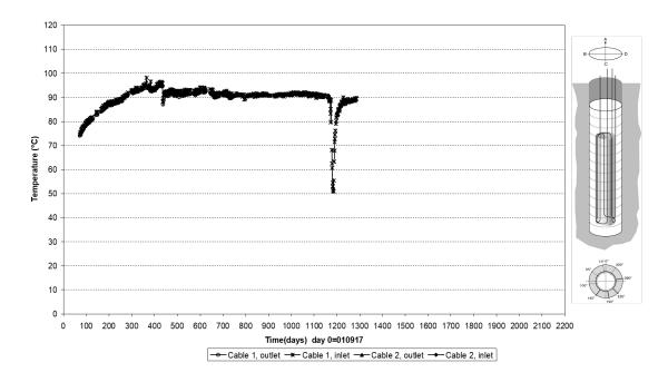
Prototype\ Hole 4\Canister (041130) Temperature profile on the canister surface - Optical fiber cables
