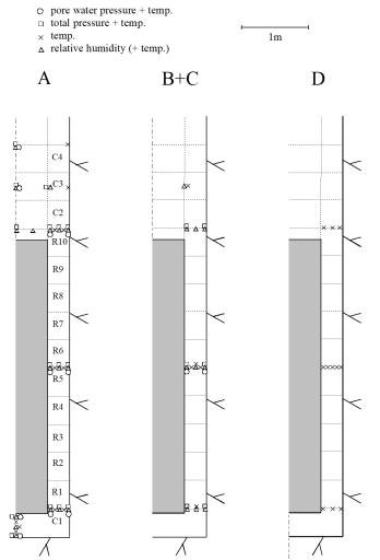
Figure 4-1 Schematic view over the instruments in four vertical sections and the block designation.
