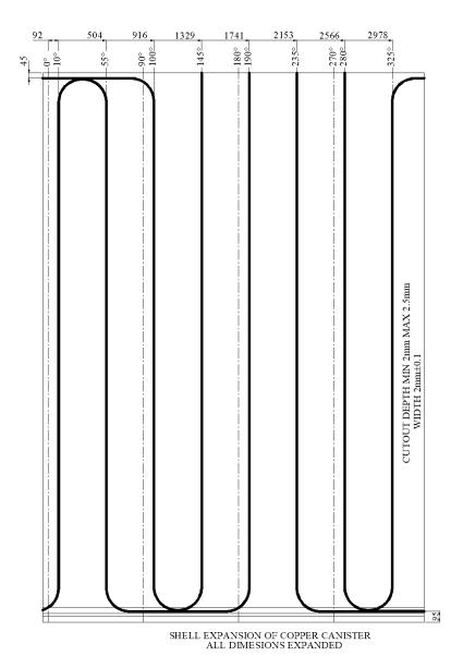
Figure 4-2 Laying of the optical fibre cables with protection tube of Inconel 625 (outer diameter 2 mm) for measurement of the canister surface temperature (surface unfolded).
