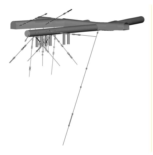
Figure A5-10-1. View of the drilled core holes in the Prototype Repository Section I. The length from the Itunnel to the end of the TBM-tunnel is 90 m. The diameter of the
