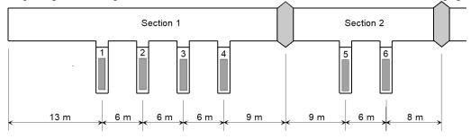
Figure 1-1 Schematic view of the Prototype Repository
