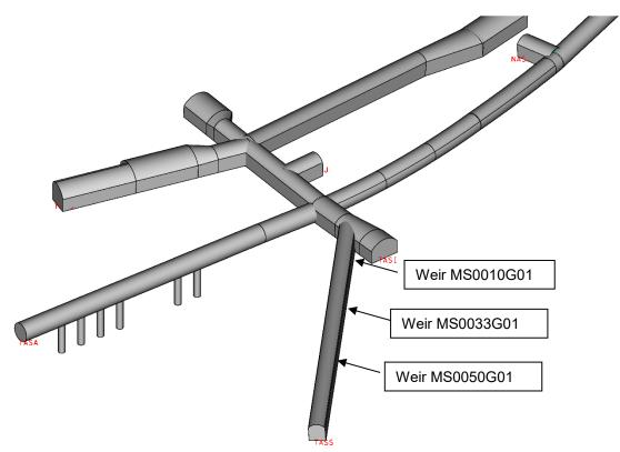
Figure A5-10-3 The tunnel-system including the TASS-tunnel with indication of the weir locations in TASS.
