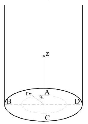
Figur 2-1 Figure describing the instrument planes (A-D) and the coordinate system used when describing the instrument positions (A headed against the end of the tunnel).
