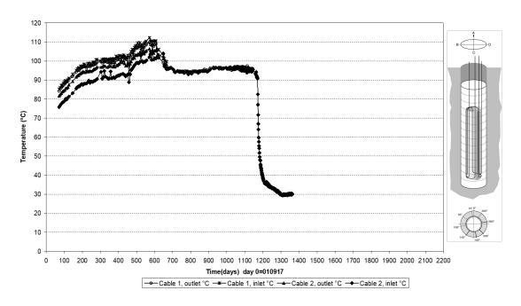
Prototype\ Hole 2 \Canister (050601) Temperature profile on the canister surface - Optical fiber cables
