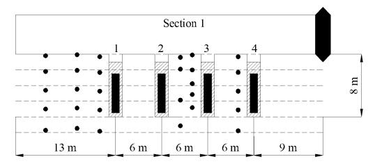
Figure 4-3 Overview of the temperature sensors in the rock. Length section.
