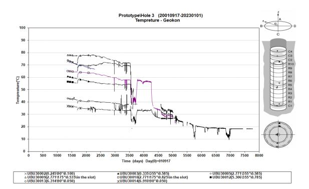
Prototype\Rock\Hole 3 (20010917-20230101) Temperature - Pentronic
