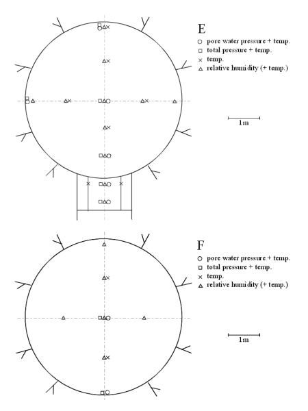
Figure 4-6 Schematic view over the sensors positions in the different sections. (Towards the end of the tunnel).
