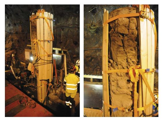
*Figure 4-12.* Left: The test package was lifted up in one piece. In order to avoid pieces from falling off during the handling, the test package was surrounded by boards and straps. Right: Photo showing the rock cover at the top.
