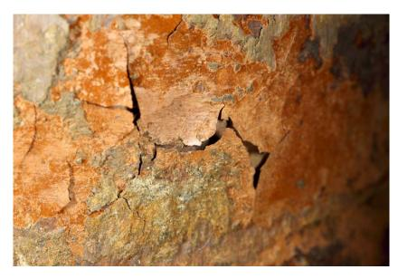
Figure 6-23. ABM2 Febex block 9. A crust on the surface of the iron heater.
