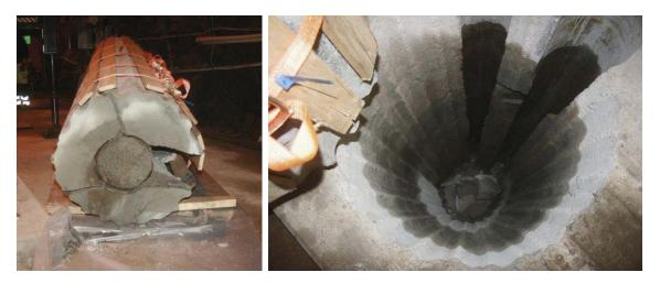
*Figure 5-10.* Left: The test package was lifted up almost in one piece. A minor rock piece close to the bottom fell off during the uplift. Right: Photo showing the rock after retrieval of the test package.
