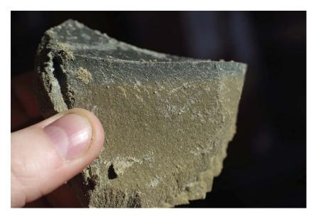
Figure 6-7. ABM2 Calcigel block 3. Showing a dark reaction zone towards the contact with the iron heater.
