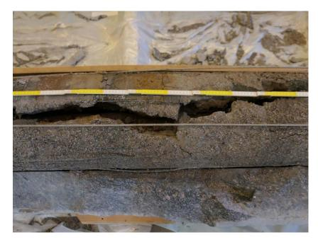
*Figure 5-13.* Large fractures in the bentonite were present along the complete test package. The photo shows the situation for block no. 20 (left) to block no. 11 (right).
