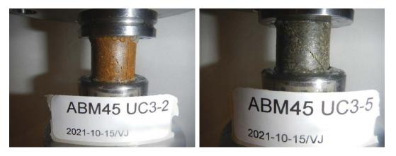
*Figure A2-9.* Photo after unconfined compression tests on ion-exchanged specimens of Asha 505 and MX-80 with dry densities  $1550 \text{ kg/m}^3$  and  $1490 \text{ kg/m}^3$  respectively.
