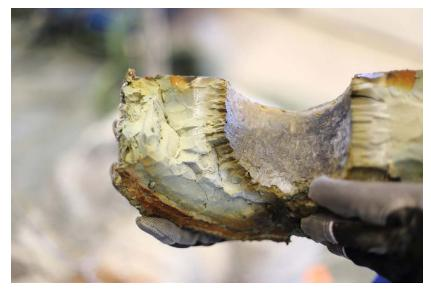
*Figure 6-10. ABM2 DepCAN. Some of the blocks showed centro-symmetrical white precipitates with a fairly constant distance to the iron heater.*
