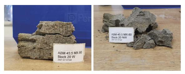
Figure A1-1. MX-80 samples from ABM 5 used for the analyses. Samples were taken from block number 20.
