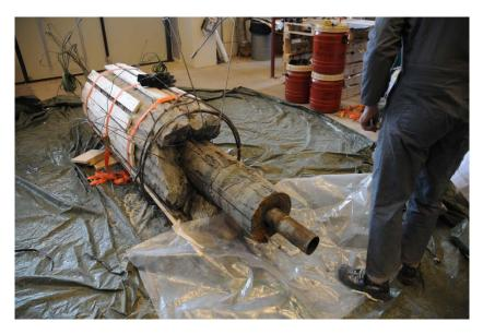
Figure 4-15. The bottom plate has been cut off from the steel tube and some of the blocks have been removed.
