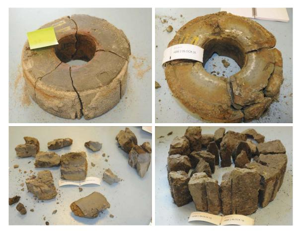
*Figure 4-17. Examples of how the different blocks could look like. Upper left: Block no. 30, MX-80. Upper right: Block no. 26, Deponit CA-N. Lower left: Block no. 22, Kunigel V1. Lower right: Block no. 16, Callovo-Oxfordian.*
