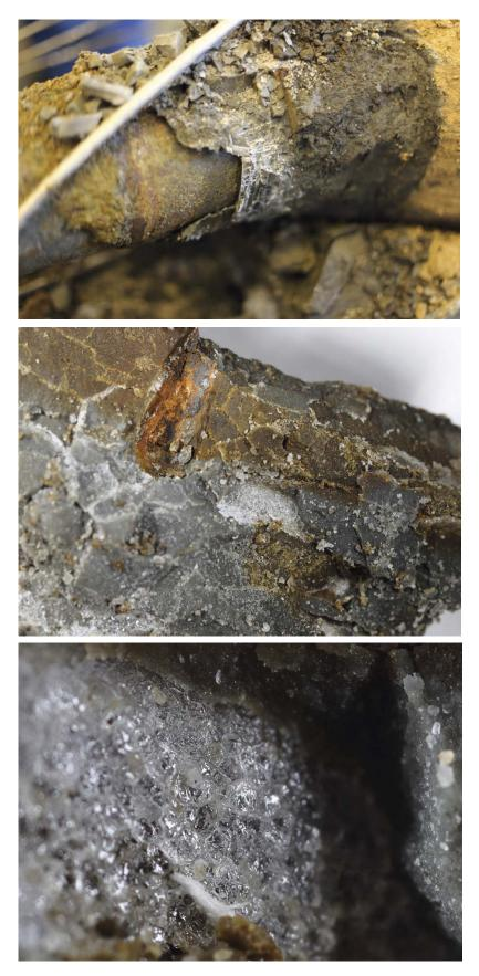
*Figure 6-19. ABM2. A highly glassy halite present in lenses of approximately*  $8 \times 4$  *mm size (Kunigel* #22).
