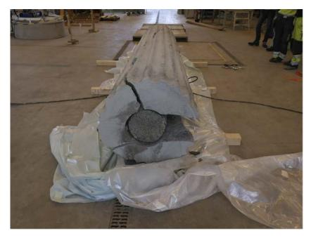
Figure 5-12. The bottom of the test package. A minor rock piece fell off during the uplift.
