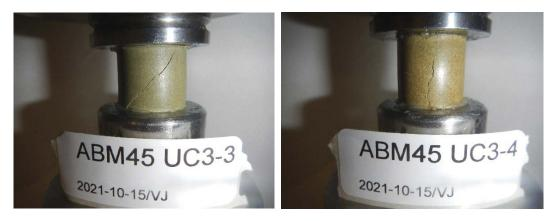
*Figure A2-10.* Photo after unconfined compression tests on ion-exchanged specimens of Deponit CA-N and Calcigel with dry densities  $1540 \text{ kg/m}^3$  and  $1480 \text{ kg/m}^3$  respectively.
