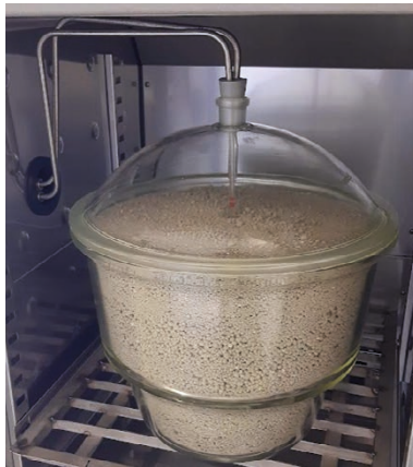
Figure 10-2. Test equipment with glass vessel in heating cabinet (left). Evolution of gas composition during heating of Milos bentonite with a water ratio of ~17 % and a temperature of 70 °C (right). From Åkesson and Laitinen (2022).
