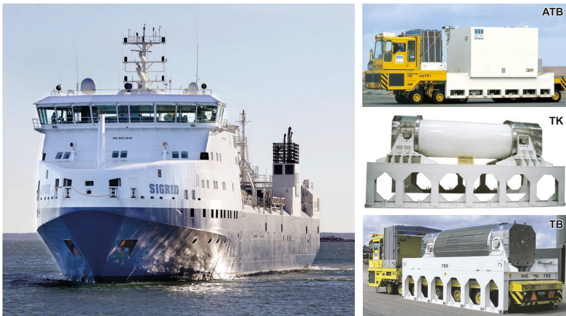
Figure 2-8. SKB's transport system currently consists of a ship, the M/S Sigrid, port terminal vehicles and waste transport casks (ATB) for short-lived radioactive waste, core components (TK), and spent fuel assemblies (TB).
