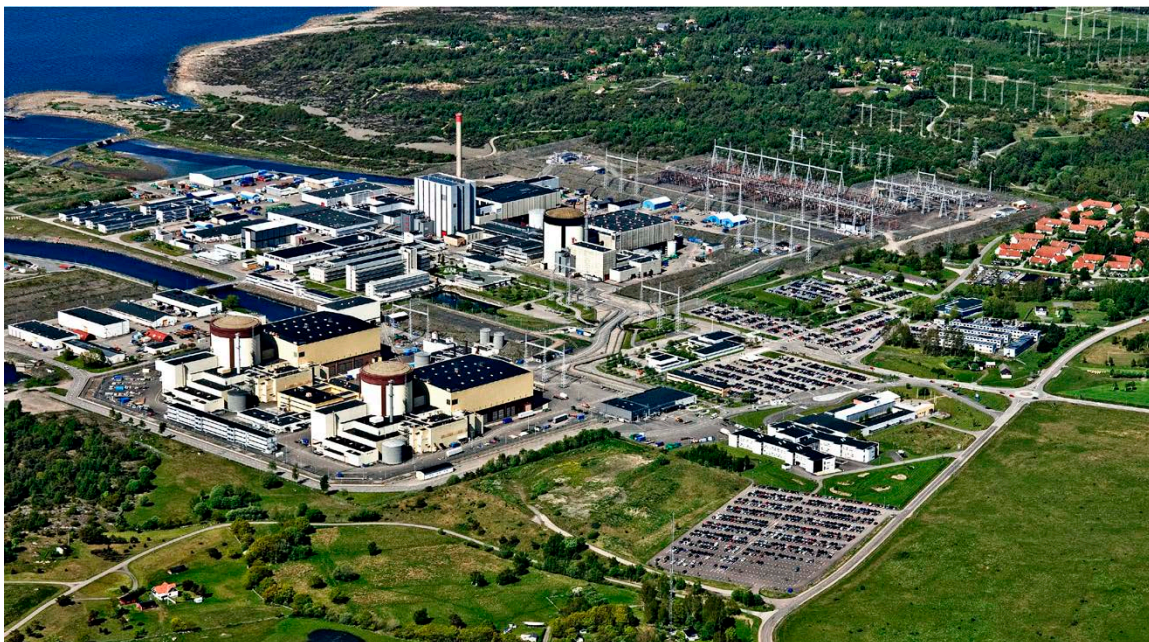
Figure 16-1. Ringhals nuclear power plant, with reactor R1 and R2 above reactor R3 and R4 in the figure. The centre of the site contains office premises and a canteen, etc. Just to the left of R1 in the figure is the plant's waste area, which includes handling, conditioning and storage of nuclear waste.
