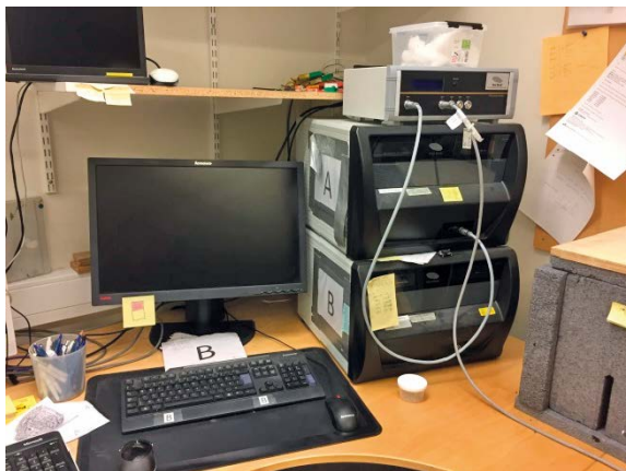
Figure 4-1. TPS-apparatus TPS 2500s with sensor switch. (The placement of the equipment was changed since the picture was taken)
