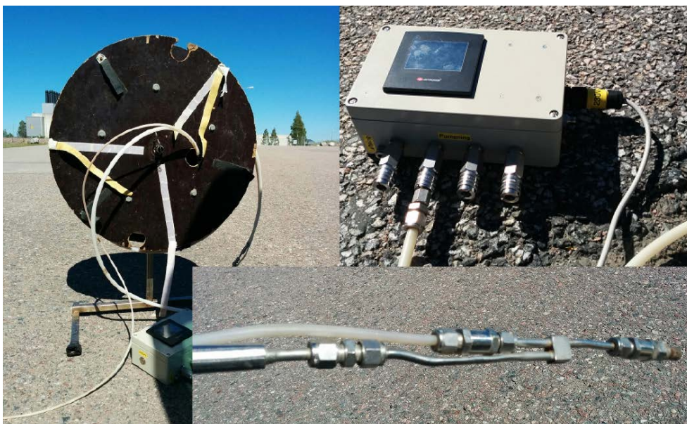
Figure 2-5. The equipment used for gas-lift pumping. On the left, the tubing lowered down the standpipe (the more narrow tube for sample water and the wider for gas) on a bobbin to simplify the lowering. To the upper right the control unit for the pumping/gas supply and lower right the end of the gas-lift pump.
