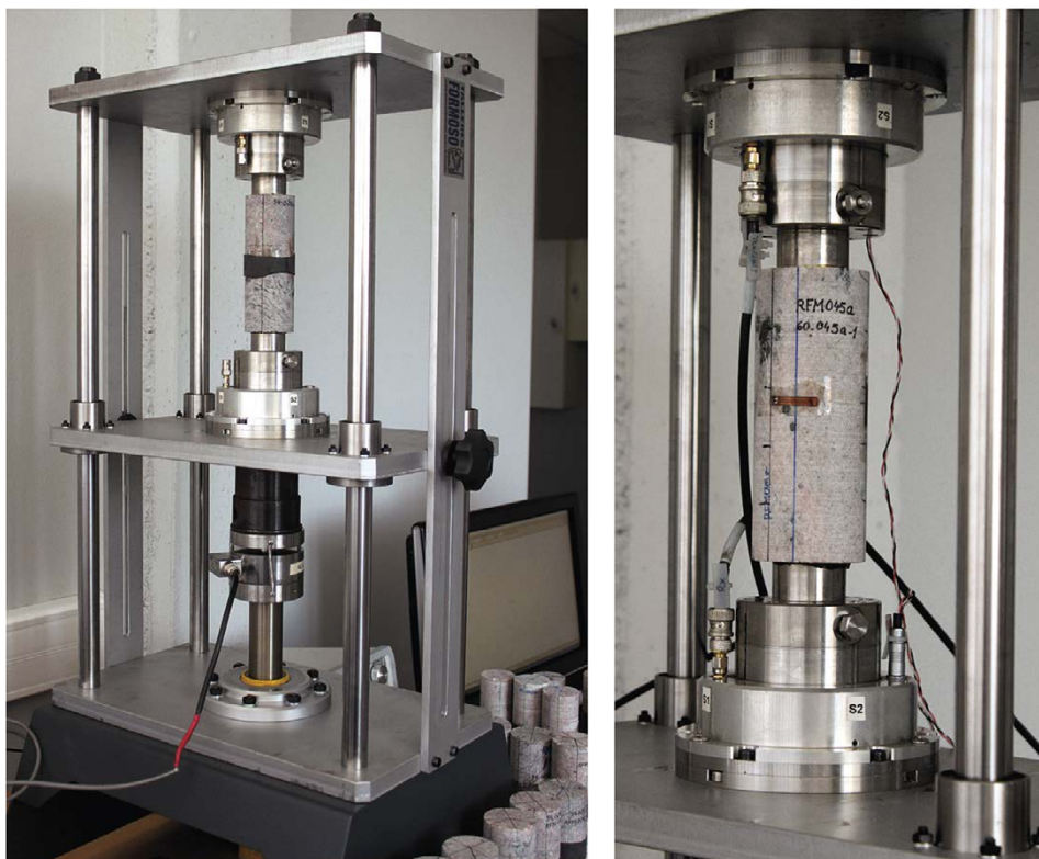
Figure 2-8. Platens and load frame used to conduct the ultrasonic pulse velocity determinations.
