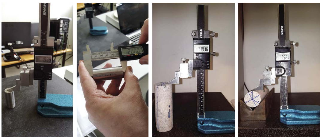
Figure 2-7. Metrological equipment used to determine the geometric compliance of plugs according to the ASTM D4543-01 (ASTM 2001) standard. Two images on the left: Precision digital height gage and Vernier calliper calibrated against a standard reference plug (2" length). Two images on the right: Plug checking over the flatness table.
