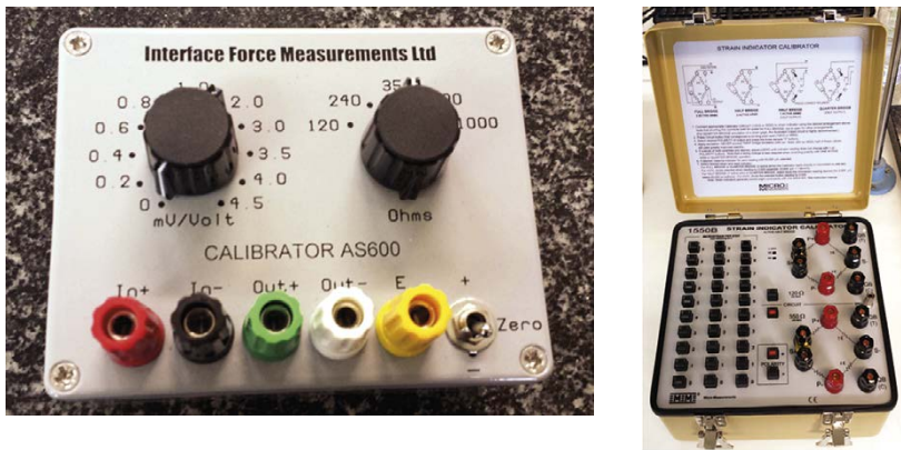
Figure 2-12. Calibration/verification instruments for checking the performance of the signal conditioning units of the load cells (left: Interface Measurements Ltd. mod. AS600) and Wheatstone bridges (right: Vishay Strain Indicator Calibrator 1550A).
