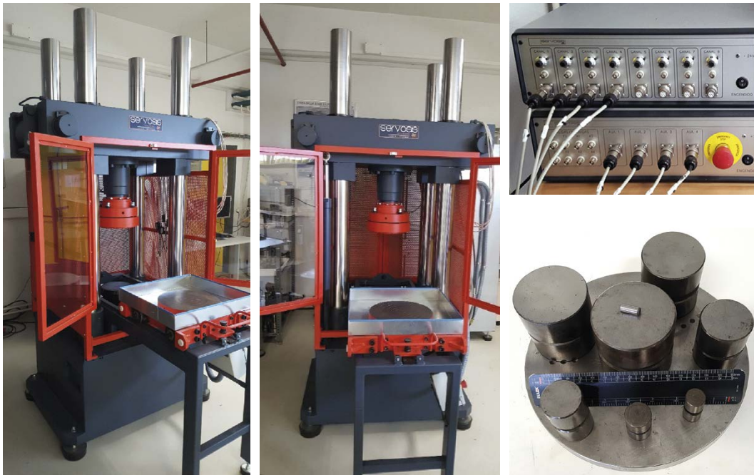
Figure 2-10. On the left side, universal load frame used to conduct the UCS tests. On the right side, strain gage and LVDT conditioning modules (top) and heat-treated load platens (bottom).
