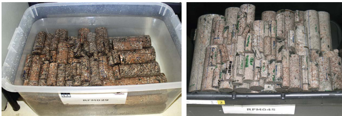
Figure 2-6. Specimens of rocks 101057 (left) and 101058 (right) submersed in tap water prior to testing.
