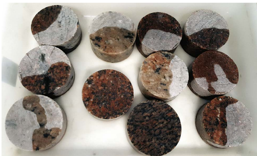
Figure 2-5. Summary view of the core plugs of rock RFM029 (101057) used in ITS tests.
