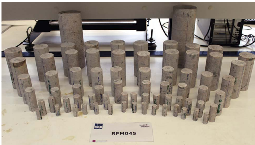
Figure 2-4. Summary view of the core plugs of rock RFM045 (101058) used in UCS tests.
