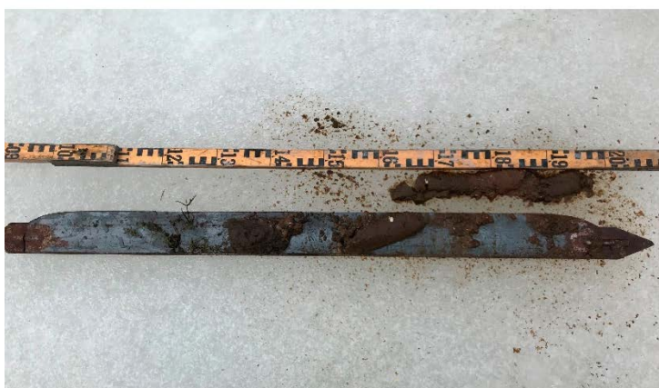
Figure 3-2. The hand driven probe (upper picture) and the Russian peat corer (lower picture) used for sampling.
