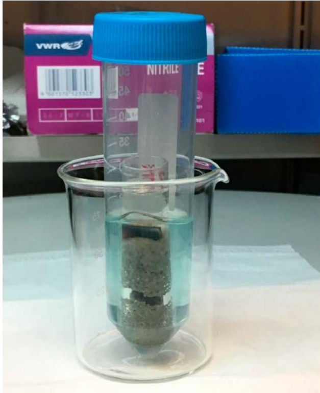
Figure 3-8. Darkening of the Ag-plate emplaced in the top part of the bentonite clay.
