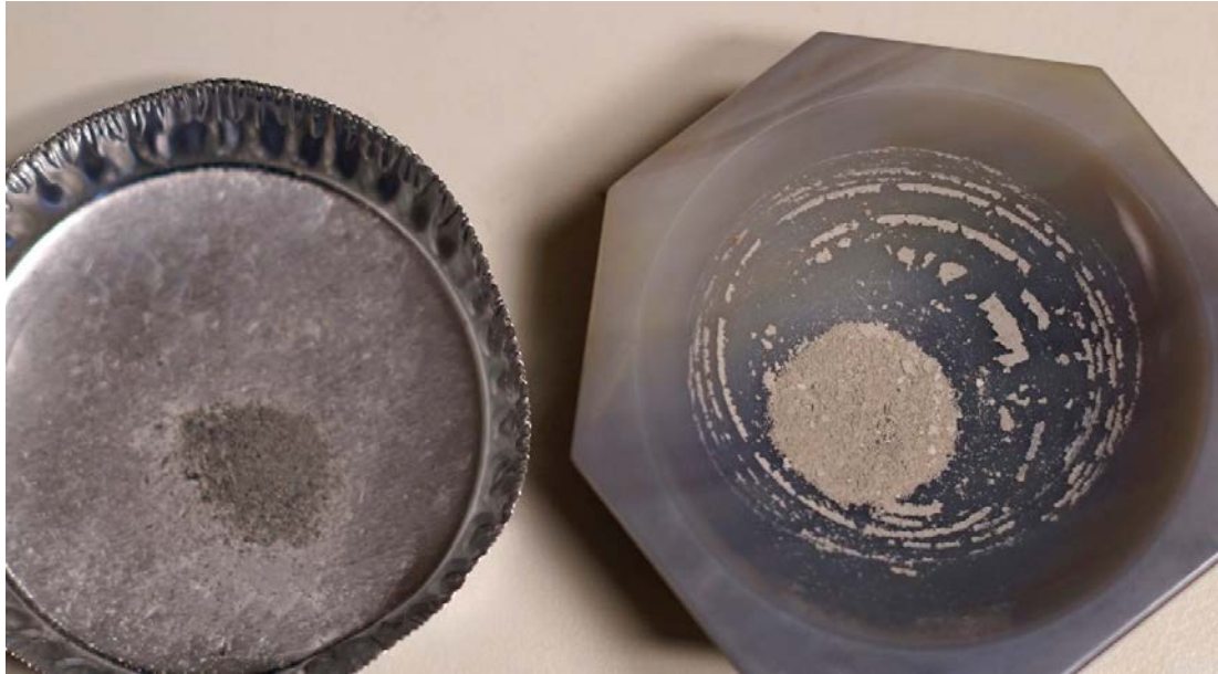
Figure 3-5. Dried and ground bentonite from S3 tube from Series #3. To the left: the dark bentonite with expected microbial matter. To the right: bright bentonite from the bottom of the tube.
