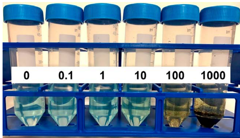
Figure 3-14. Detection limit experiment: The tubes contain \text{CuSO}_4 solution and different concentrations of sulfide solution. The numbers (0 to 1 000) represent the concentration of the added sulfide solution in \mu\text{M} . With increasing sulfide concentration a pronounced precipitation (CuS) and decolorization of the \text{CuSO}_4 solution was observed.
