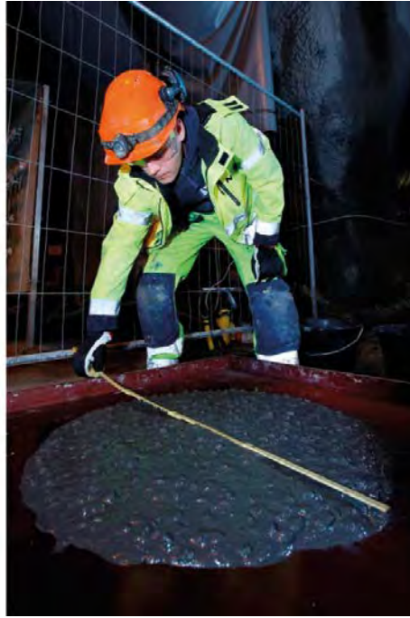
Figure 5-15. Sampling of concrete from a concrete truck (left), measuring slump flow (right).
