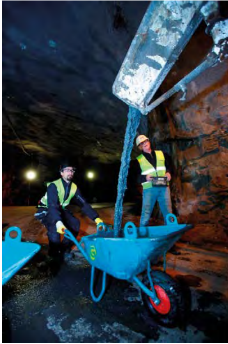
Figure 5-15. Sampling of concrete from a concrete truck (left), measuring slump flow (right).
