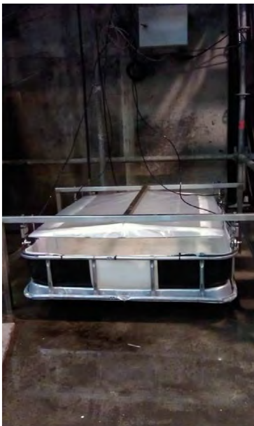
Figure 7-13. Photo showing basin for weighing of leakage water from the weir.
