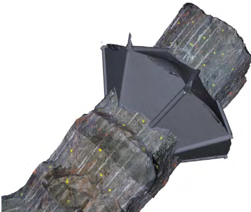
Figure 3-12. 3D-visualization, composed of data from laser scanning of TAS01 and the excavated slot abutment (seen from above).
