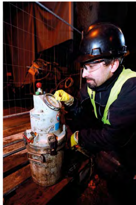
Figure 5-16. Clocking t_{500} while measuring slump flow (left), measuring air content (right).
