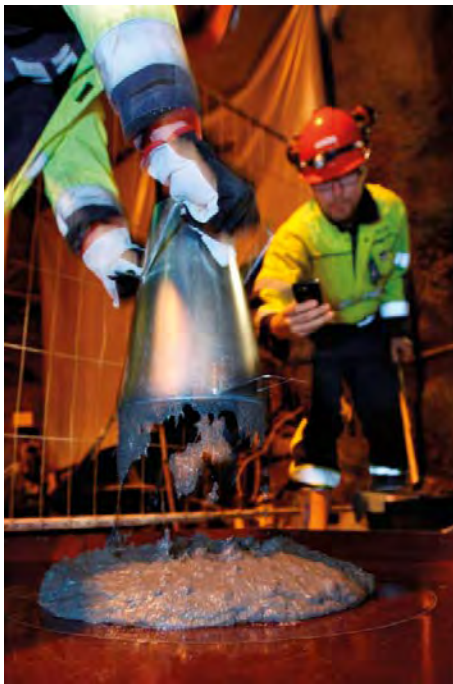
Figure 5-16. Clocking t_{500} while measuring slump flow (left), measuring air content (right).
