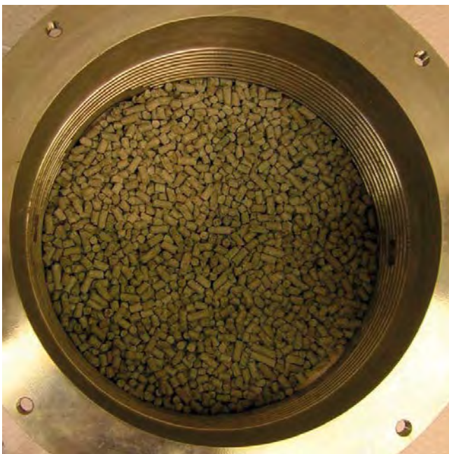
Figure 4-15. The 10 mm – thick pellet layer between the backfill and the LECA beams. Rod shaped MX-80 bentonite pellets with a diameter of 6 mm were used.
