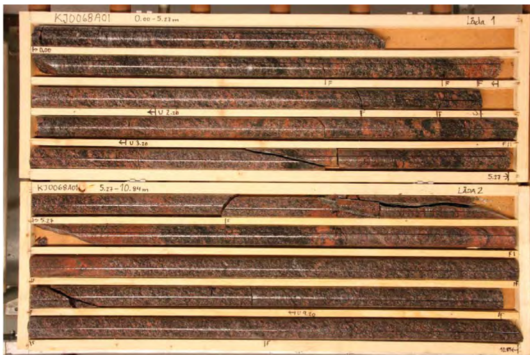
Figure 3-3. Photo of the core box for pilot hole KJ0068A01, section 0–10 m (wet core).
