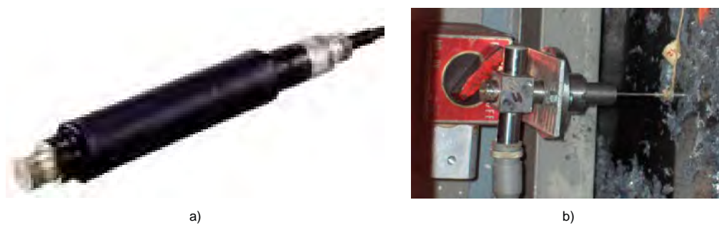
Figure 7-8. a) Joint meter (TML KJA-10A), b) LVDT sensor (HBM LVDT WA-10).
