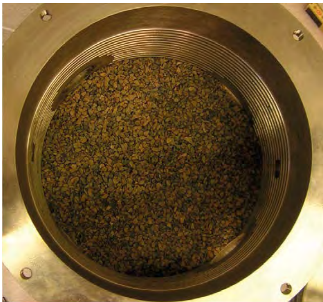
Figure 4-13. The 30 mm layer of 2–4 mm gravel from AB Sydsten emplaced in the test equipment.
