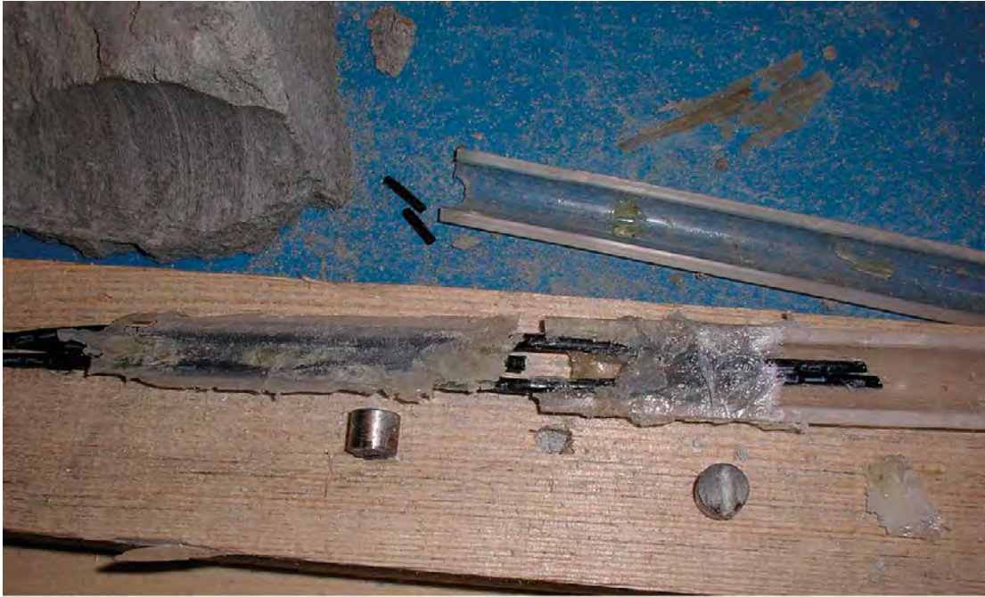
Figure 5-60. Retrieved electrode chain. (Figure 8.4 in Wiczorek et al. 2014.)
