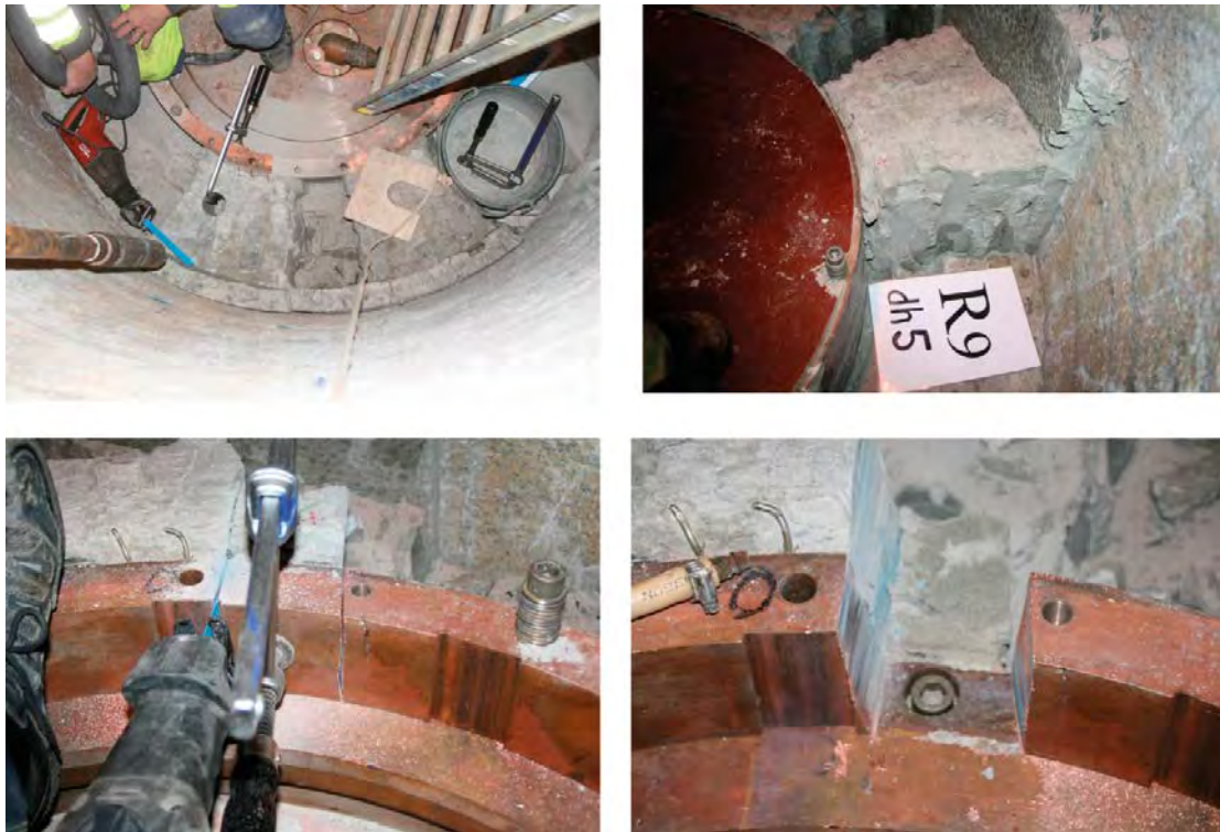
Figure 4-16. Sample taken of the canister in deposition hole No 5. Top left: Saved part of the buffer seen from above. Top right: Saved part of the buffer seen from the side. Bottom left: Sawing of the copper ring. Bottom right: Copper ring after the sample was taken. (Figure 5-7 in Johannesson and Hagman 2013.)
