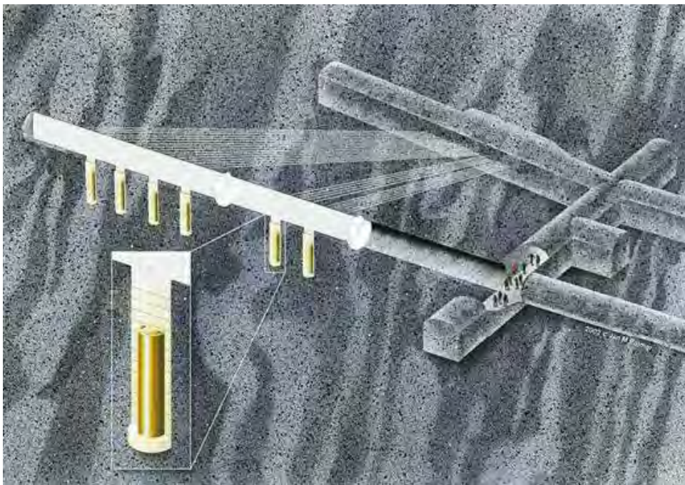
Figure 1-2. Artist's view of the Prototype Repository. The adjacent tunnel to the right in the figure (denoted G-tunnel in Figure 2-2) contains the instrument panels. Bright streaks between the Prototype Repository tunnel and the G-tunnel denote lead-through pipes. In total 32 lead-through pipes were required in order to host all cables from the Prototype Repository. In addition, two lead-through pipes were installed in the outer plug in order to facilitate on-line sampling of gas and water from the outer section.
