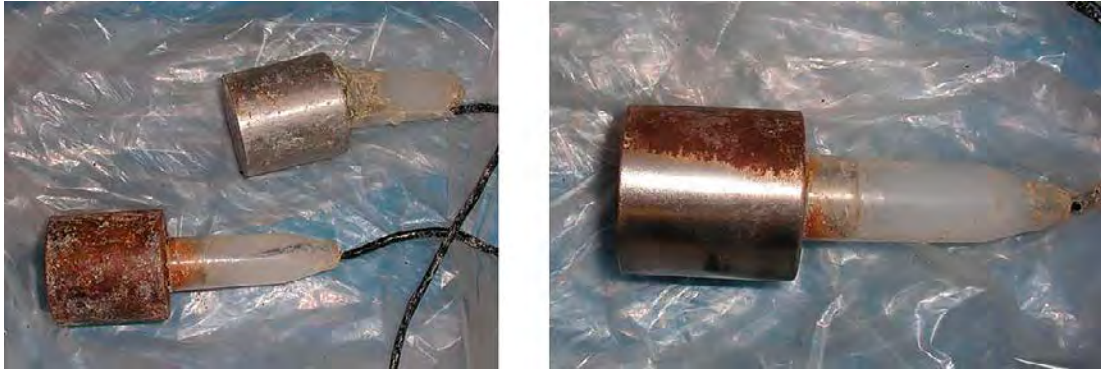
Figure 5-57. Electrodes from the backfill in the outer section showing surface corrosion. (Figure 8.1 in Wieczorek et al. 2014.)
