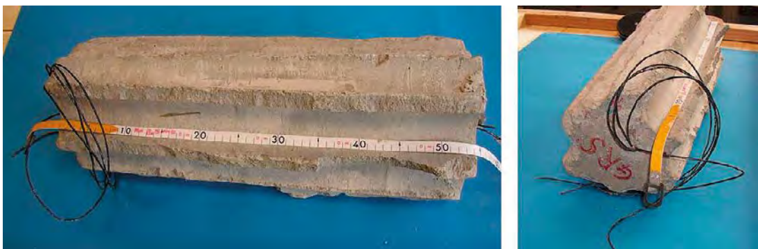
Figure 5-58. Core section from the top central buffer of deposition hole No 5 with embedded electrode chain. (Figure 8.2 in Wieczorek et al. 2014.)
