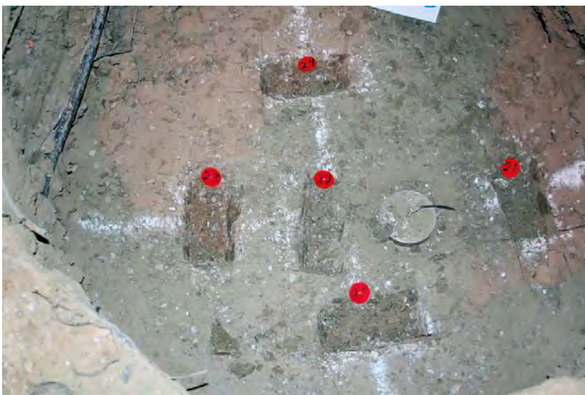
Figure 4-6. Samples taken from the tunnel backfill inside a deposition hole together with an installed sensor. (Figure 3-6 in Johannesson and Hagman 2013.)
