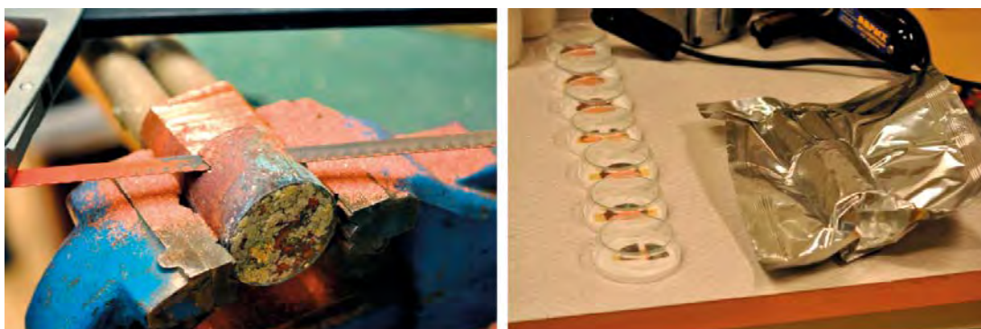
Figure 5-42. Left: Cutting out samples from the copper electrode “Black”. Right: Temporary storage of samples from the copper electrode “Black”. (Figure 2-4 in Rosborg 2013b.)
