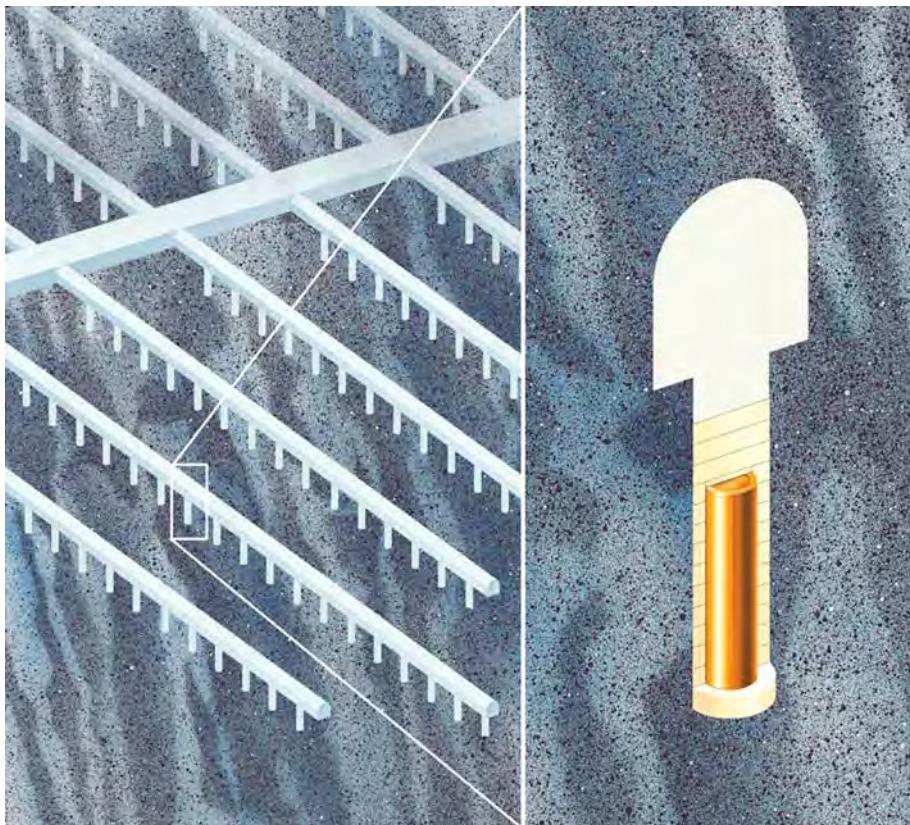
Figure 1-1. Illustration of the KBS-3V method at a depth of about 500 m in the Swedish bedrock. To the left: layout of deposition tunnels. To the right: layout of a deposition hole. (The vertical (V) emplacement mode was distinguished from the horizontal (H) emplacement mode first in the early 2000ies.)
