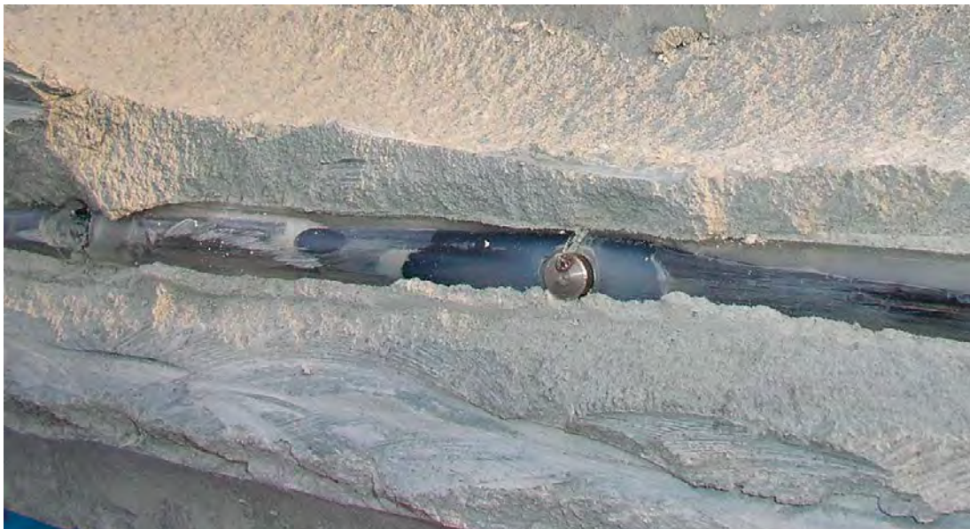
Figure 5-59. Electrode chain embedded in the buffer. (Figure 8.3 in Wieczorek et al. 2014.)
