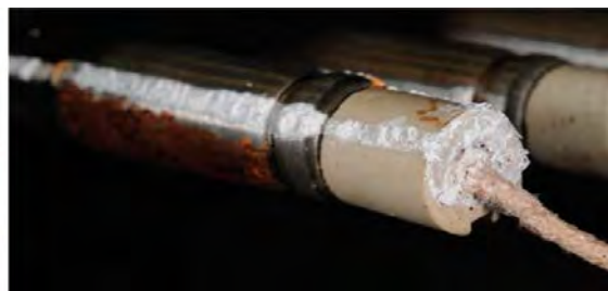
Figure 5-53. Some heater elements in the canister in deposition hole No 6 have swollen due to sorption of water by the insulation material.
