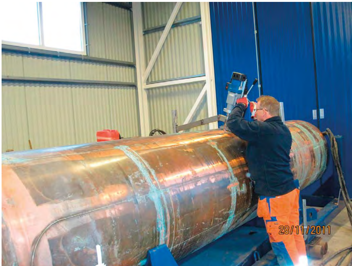
Figure 4-17. Sampling of the canister in deposition hole No 6 by drilling of 28 mm cores through the 50 mm thick copper shell. (Figure 2-2 in Taxén et al. 2012.)
