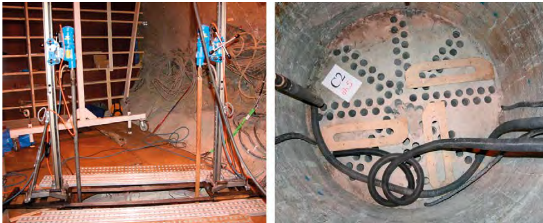
Figure 4-7. Left: The core drilling machines standing on the tunnel floor. Right: Holes from cores taken from a buffer block. Wooden templates were used to position the drill bit. (Figure 4-1 in Johannesson and Hagman 2013.)
