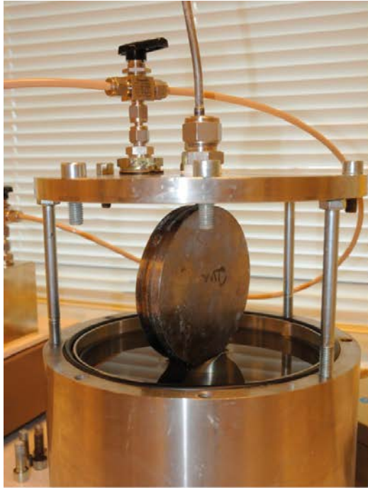
a) Test cell with a total pressure sensor before immersion into water.
