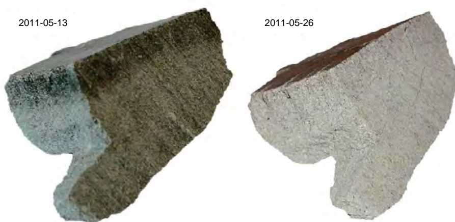
Figure 5-9. Bentonite sample from block R10 in deposition hole No 6. (Block position is shown in Figure 2-14). Left: Parts of the innermost 10 mm in the buffer block were dark at removal. Right: The darkness disappeared irreversibly upon drying. (Figure 3-56 in Olsson et al. 2013.)
