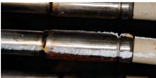
Figure 5-53. Some heater elements in the canister in deposition hole No 6 have swollen due to sorption of water by the insulation material.
