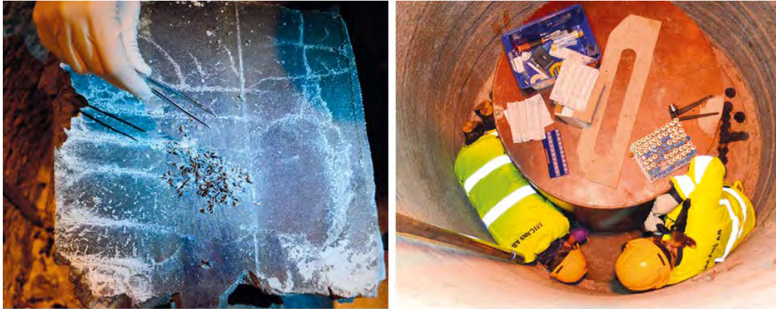
Figure 4-9. Left: The method whereby, using a sterile scalpel, bentonite samples were scraped off the buffer surface that had been in close contact with the copper canister. Right: The sampling site in deposition hole No 6. (Figure 2-2 in Arlinger et al. 2013.)
