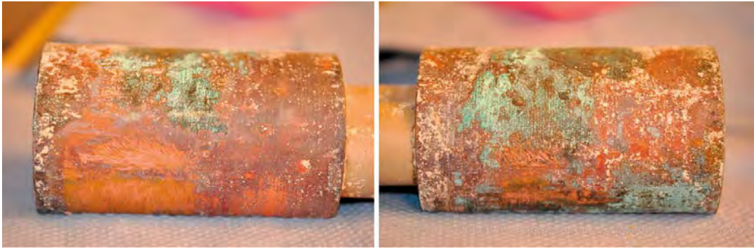
Figure 5-43. The two photographs show where corrosion products were scraped off from copper electrode “Black”. Left: the sample area termed “H” where mainly brownish corrosion products existed. Right: the sample area termed “V” where mainly blue-green corrosion products were sampled. (Figure 2-5 in Rosborg 2013b.)
