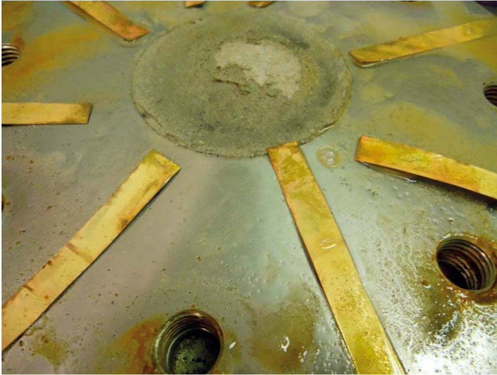
Figure 2-18. Photo taken during dismantling of Test 3, showing the artificial fracture after removal of the upper lid. The bentonite has swelled and filled the radial slot and some bentonite can also be seen in the “fracture”.
