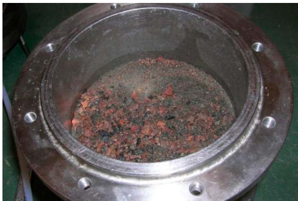
Figure 3-9. Significant settling was observed at low initial densities in the hydraulic conductivity tests for MakPak® 0–5 mm (photo) and natural sand/gravel 0–4 mm. Initially the cylinder was entirely filled with material but during the test the specimen settled to about 70% of the initial height.
