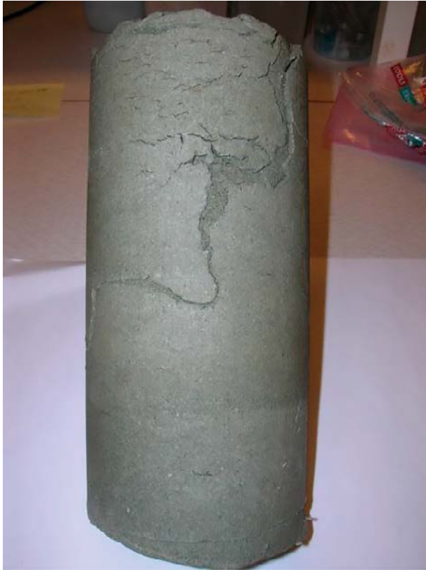
Figure 2-17. Photo of the bentonite specimen from Test 1. A very evident flow channel can be seen on the surface.
