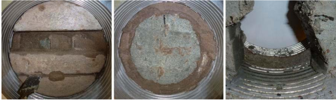
Figure 4-48. Dismantling of Test 4B. LEFT: First the concrete beams were removed from the outside. MIDDLE: The outermost part of cast cement was left in place to be able to make observations from the inside once the bentonite sealing was removed. The bentonite sealing is seen in the centre. RIGHT: The bentonite sealing was removed carefully from the filter side.
