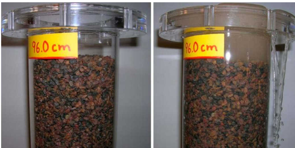
Figure 3-11. The result from the settling test on macadam 2–4mm. No substantial settling is observed in the material.
