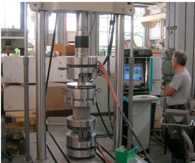
Figure 3-15. Compressibility tests performed on the new Leca-block specimens received from Nyströms Cement AB. The tests were performed at the department of Structural Engineering at LTH/Lund University since the available Trittech 50kN press was insufficient in capacity.
