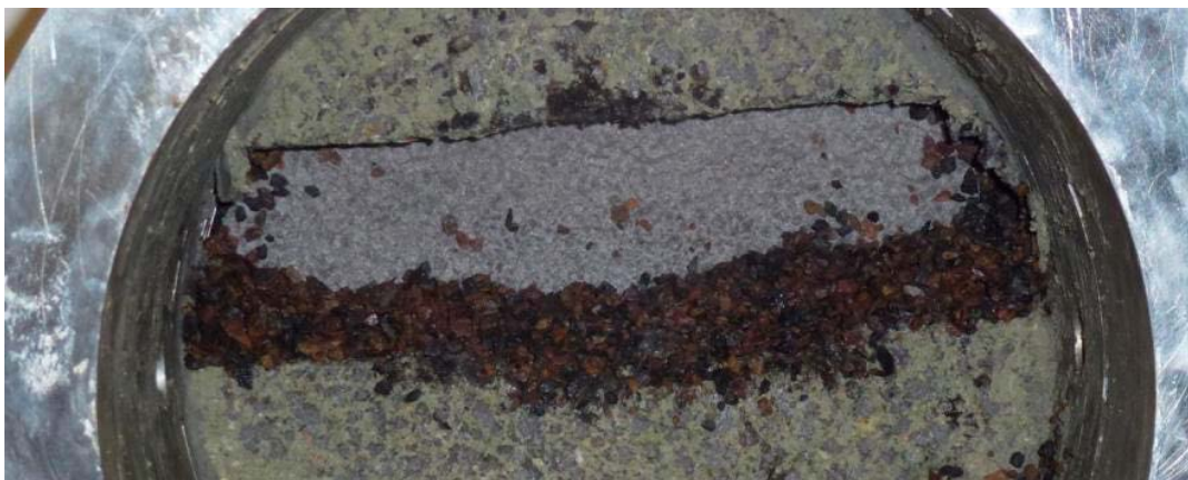
Figure 4-56. View from the backfill side of the equipment. Behind the Leca-beams both the macadam filter and the geotextile is visible. No backfill bentonite intrusion was observed in the Leca-macadam filter in Test 5.
