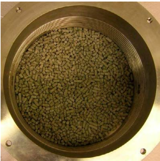
Figure 4-9. The 10 mm – thick pellet layer between the backfill and the Leca beams. Rod shaped MX-80 bentonite pellets with a diameter of 6 mm were used.
