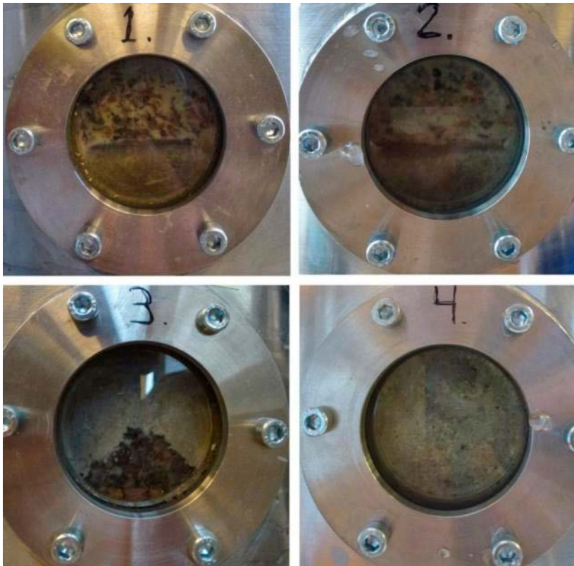
Figure 4-41. View through the windows at test dismantling. There is bentonite intrusion from the backfill past the Leca-beams into the macadam filter.
