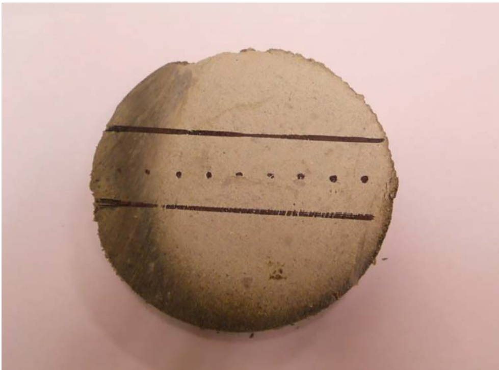
Figure 2-19. Photo showing a cross-section of the bentonite specimen in Test 3. The bentonite has swelled unsymmetrical, only taking up water at one side.
