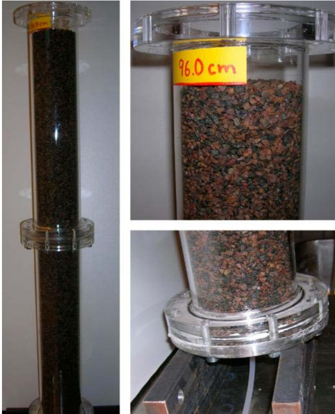
Figure 3-10. The test arrangement for the settling test on macadam 2–4 mm.
