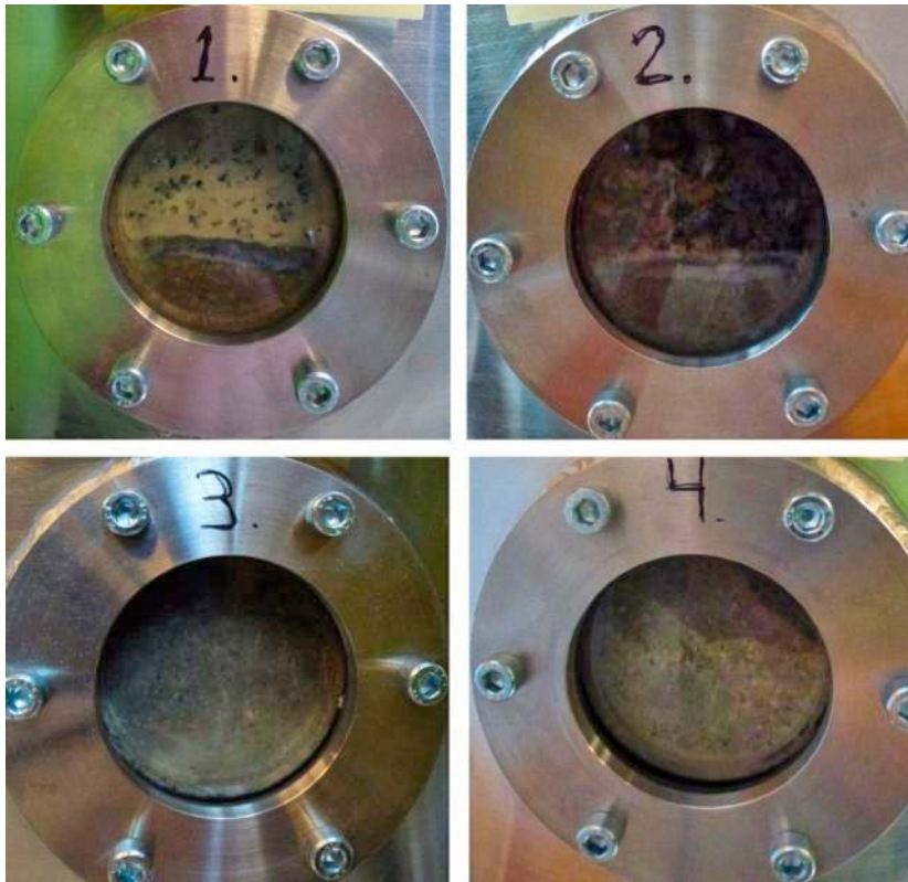
Figure 4-31. Photos taken at test termination. Windows 1 and 2 shows the bentonite sealing, the geotextile and the macadam filter. Windows 3 and 4 shows the Leca beams and the pellets surrounding the backfill bentonite. The backfill bentonite has swelled and intruded into the space between the Leca beams and the windows. Window 1 seems to show that the bentonite intruded all the way into the macadam filter.
