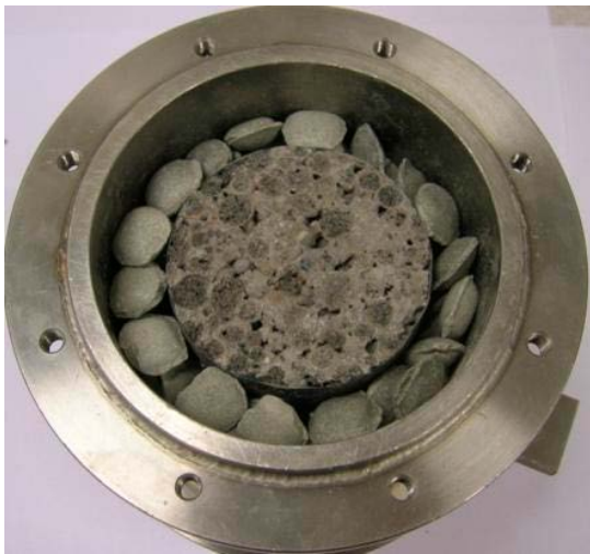
Figure 3-18. The slot is filled with pellets made from MX80 bentonite to prevent interface flow.
