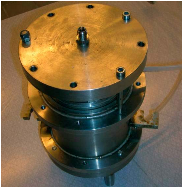
Figure 3-25. The clogging tests on the stiff draining material used the specimens from the hydraulic conductivity tests.
