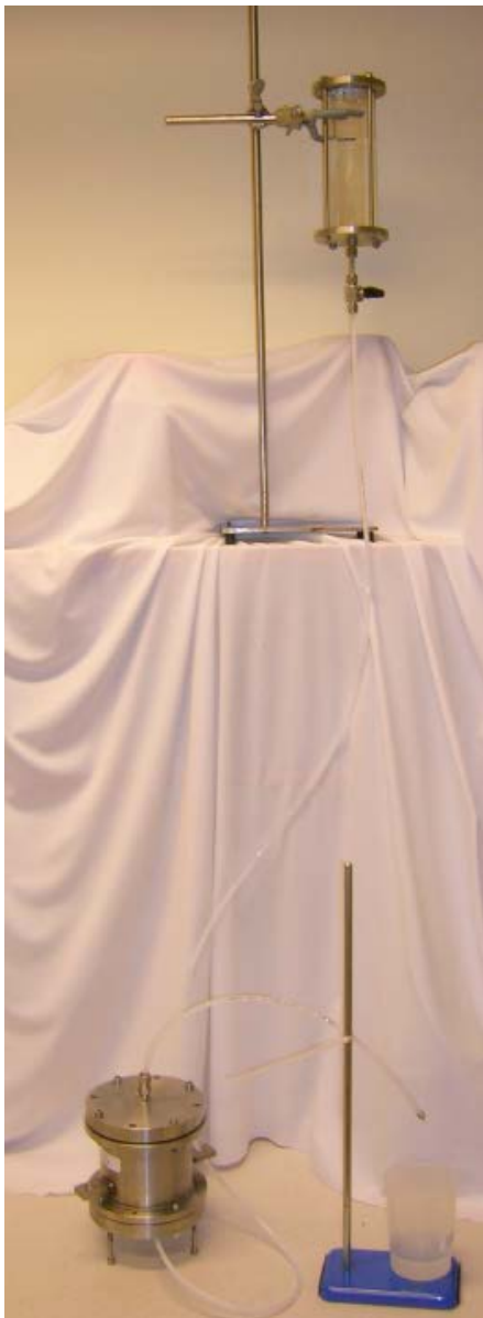
Figure 3-7. The hydraulic conductivity test arrangement.
