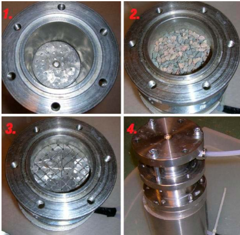
Figure 3-21. Geological drainage material specimen preparation for the clogging tests. The specimen is confined between two specially prepared steel filters to keep it in place and distribute the in- and outflow evenly over the specimen area.
