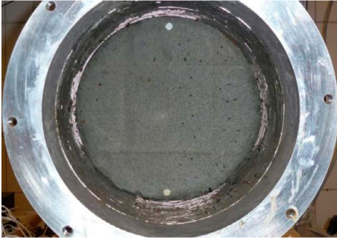
Figure 4-39. The bentonite sealing and the thumbtacks used to measure the axial expansion. The sealing expanded about 6–7 mm in axial direction which corresponds to about 12–14%.
