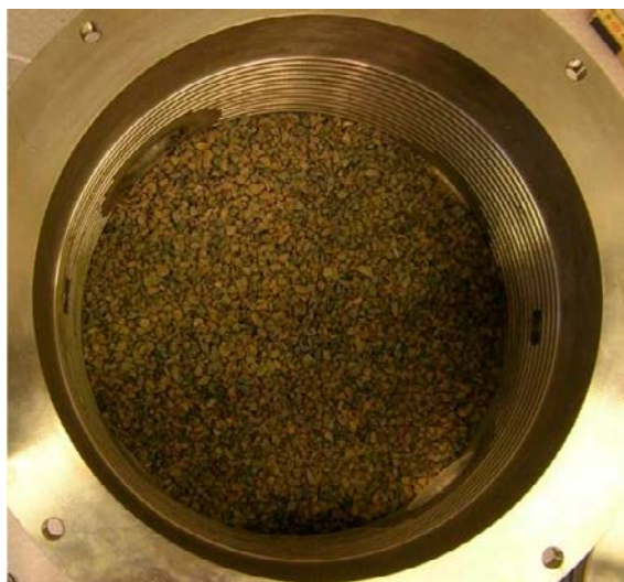
Figure 4-7. The 30 mm layer of 2–4 mm macadam from AB Sydsten emplaced in the test equipment.
