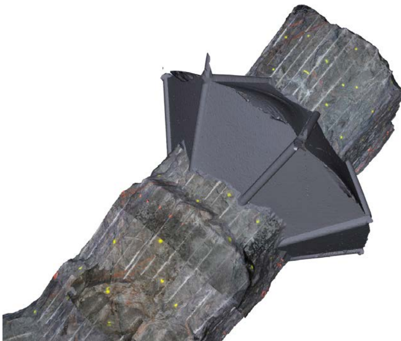
Figure 4-1. Illustrative 3D-model structured of data from laser scanning of TAS01 and the excavated slot abutment (seen from above).
