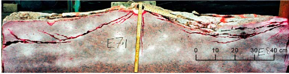
Figure 9-12. A cross-cut through a bench in a quarry (Olsson and Bergqvist 1996).
