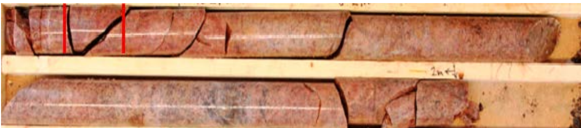
Figure 8-9. Core images where the measured section is marked with two red lines.
