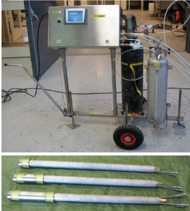
Figure 8-3. Control unit, pressure tank and gas vessel mounted on a transport carriage (upper picture). Packer system for section lengths 10 and 20 cm and for single-hole packer measurements (lower picture).
