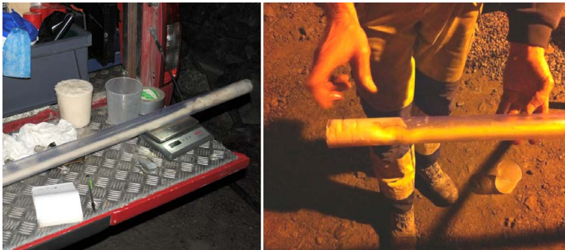
Figure 4-7. Calibration of the charging equipment using tubes of acrylic glass. Note the transition between the bottom charge and emulsion string.
