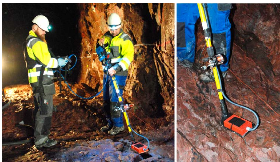
Figure 7-2. GPR measurements at the TAS04 tunnel floor.
