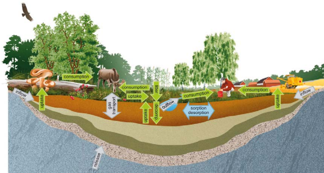
Figure 8-2. A conceptual representation of important fluxes affecting the transport and accumulation of elements in a wetland ecosystem and in arable land on a drained part of a mire, where human exposure is an important consideration in the safety assessment. Green arrows are fluxes mediated by biota, grey arrows are water and gas fluxes, the blue arrow represents sorption/desorption processes, and consumption also includes water for drinking. The mire was preceded by a lake and a marine stage in which gyttya/clay and postglacial clay were deposited prior to the peat.
