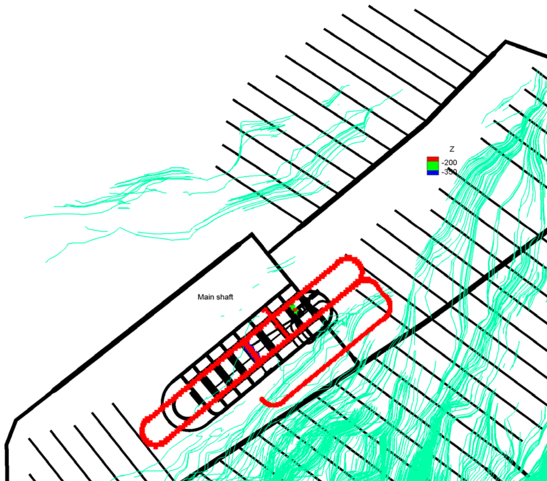
Figure 6-27. Backward particle tracking trajectories for Case B. Focused around the main shaft. Only trajectory parts above elevation -370 m are shown.
