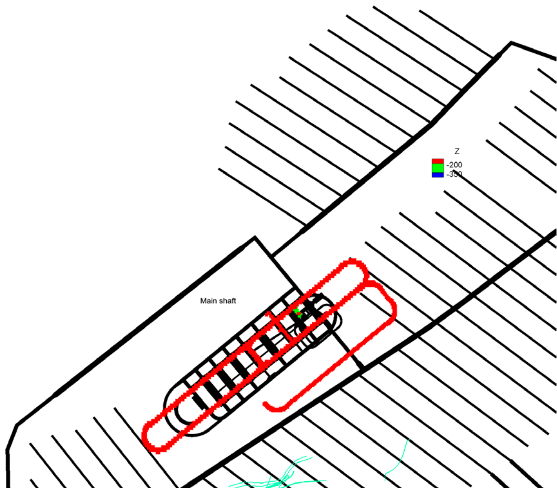
Figure 6-28. Backward particle tracking trajectories for Case B. Focused around the main shaft. Only trajectory parts above elevation -200 m are shown.
