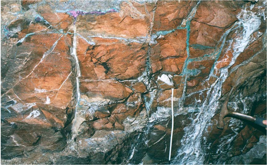
Figure 2-21. Sealed fractures in the natural cement zone at the Maqarin site in Jordan (note field hammer at bottom right for scale). The zone of interaction in the cement is relatively narrow (Pitty and Alexander 2011).
