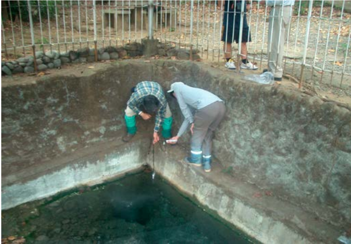
Figure 2-13. Alkaline groundwater flowing from a fracture in the gabbro of the Zambales ophiolite, Philippines. The groundwater here has a pH of 11.1 and releases a mixture of hydrogen (up to 3,500 ppm) and methane (up to 5,000 ppm) bubbles (misty area in top corner of the pool).
