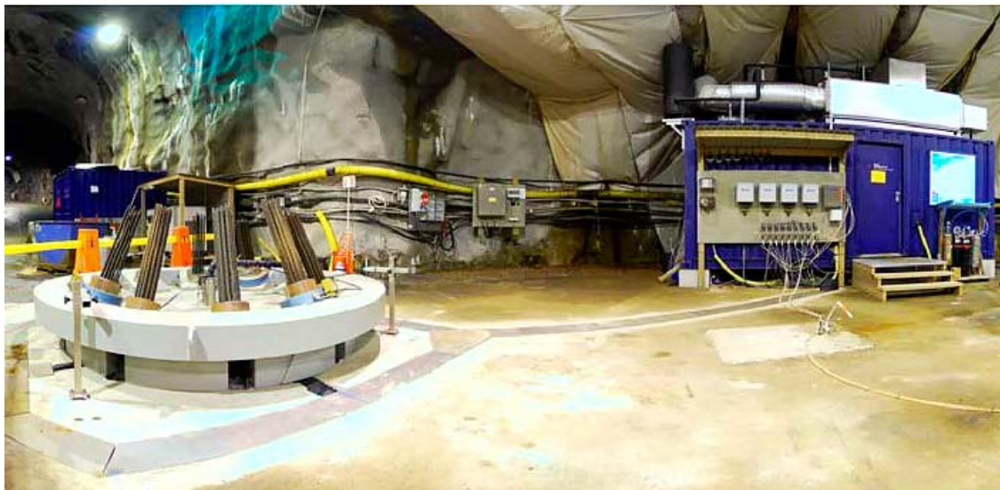
Figure 2-26. The large scale gas injection test at the -420 m level in the Äspö URL (SKB 2011).
