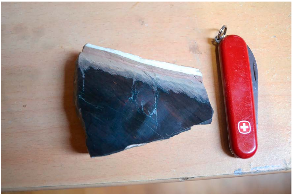
Figure 2-22. Sealed fracture from the natural cement zone at the Daba site in central Jordan (site details in Pitty and Alexander (2011)). The knife is 8 cm long and the white material at the top of the sample is calcite fracture fill with the bleached zone in the black cement indicating the leached zone. Image courtesy H. Alexander Photogenics.
